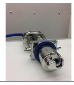
FIGURE 3.2: The probe holder rented from ExpoPharma. The probe is mounted from the back.
