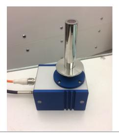
FIGURE 3.4: NIR probe used for both off-line and in-line measurements.
