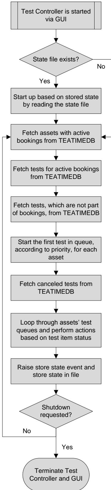
Figure 21: Test controller work flow
