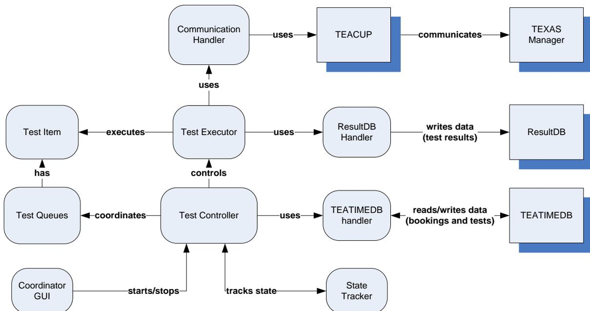
Figure 20: The interaction diagram for the test automation
