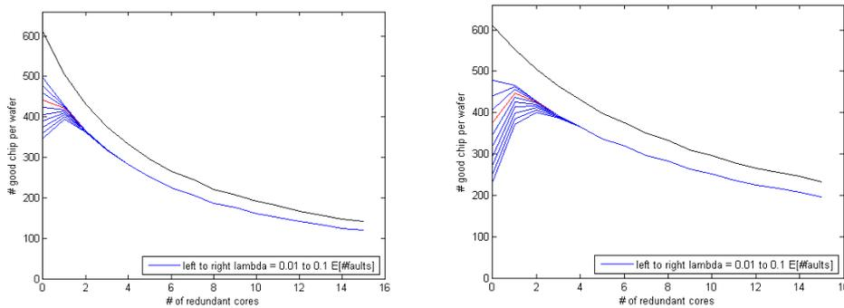
**Figure 13: The number of good chips per wafer with different amount of redundant cores for example system configuration for 4 and 8 required cores.**
