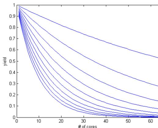
Figure 8: The combined yield of a system with multiple cores requiring all the cores to work
