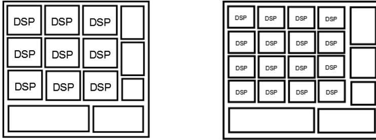
Figure 11: The example SoC topology for 9 and 16 cores. The area for the multi core cluster remains the same for both cases before redundant cores are added.
