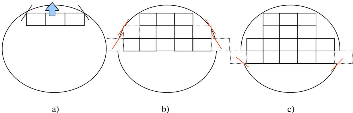
Figure 2: Illustrations of the steps in the numerical algorithm. a) *Step 1*, pushing the row of chips towards the top of the wafer, until the top corners hit the wafer edge. b) *Step 2*, adding more chips until the top corners cut the wafer depicted by the red lines. c) *Step 3*, same as b) except for the lower half wafer the chip's bottom corners are checked to be inside the wafer edge
