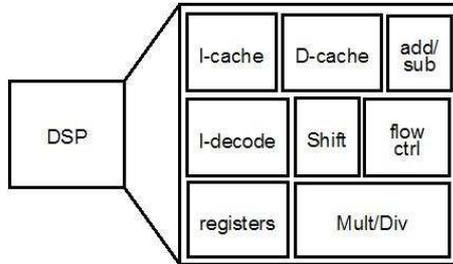
Figure 10: imaginary DSP architecture logic floor plan
