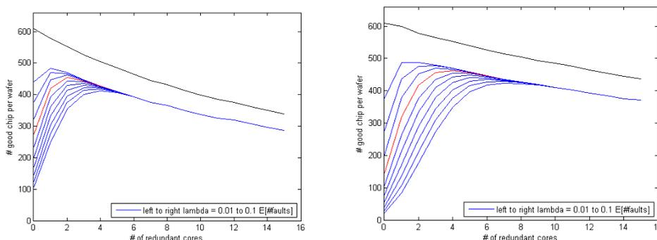
**Figure 14: The number of good chips per wafer with different amount of redundant cores for example system configuration for 16 and 32 required cores.**
