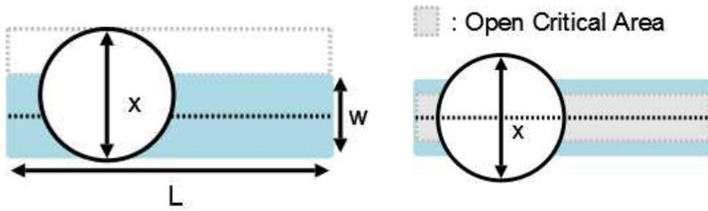
Figure 5: a conductive wire and a harmful defect size, shows how the difference between diameter and width converts into critical area
