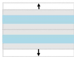
Figure 6: multiple parallel conductive wires. Shows how the critical areas have grown together and continues to expand only from the top and bottom most wires.
