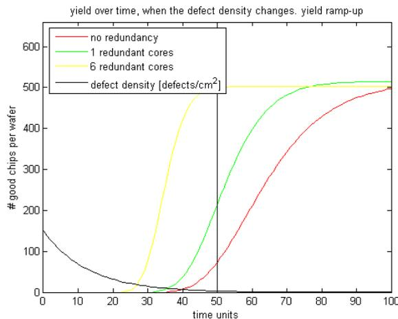
**Figure 16: yield ramp for a 64 core DSP cluster, 3 configurations of redundancy. Black line defect density over time**
