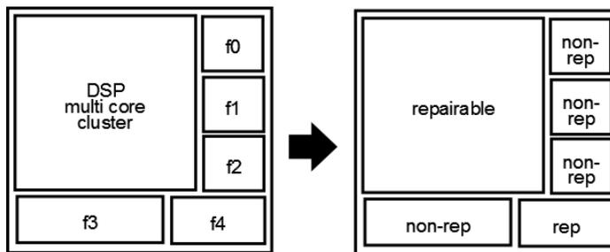
Figure 9: An imaginary system with a multi core cluster, divided into repairable and non-repairable blocks on the right
