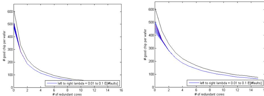
**Figure 12:** The number of good chips per wafer with different amount of redundant cores for example system configuration for 1 and 2 required cores.
