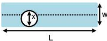
Figure 4: conceptual illustration of a blue conductive wire with a defect of harmless size to the left and a harmful defect size to the right
