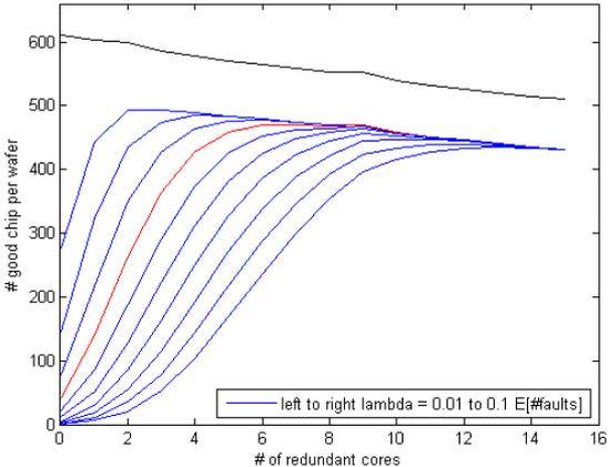
**Figure 15: The number of good chips per wafer with different amount of redundant cores for example system configuration for 64 required cores.**
