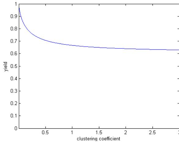
Figure 3: Negative Binomial distribution function for a fixed  $\lambda = 0.5$  and a varying  $\alpha$ .
