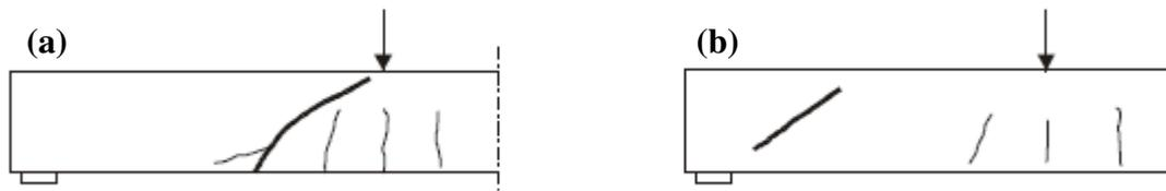
Figure 2.7 (a) Shear flexure, (b) Shear tension (Walraven 2002)
