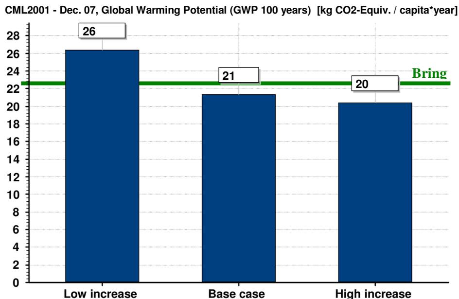
Figure 5.5 Emissions from co-mingled collection with different collection levels. A low increase gives a total amount of 93.6 kg collected recycling; the base case gives a total amount of 103.8 kg and the high increase gives a total amount of 106.9 kg.
