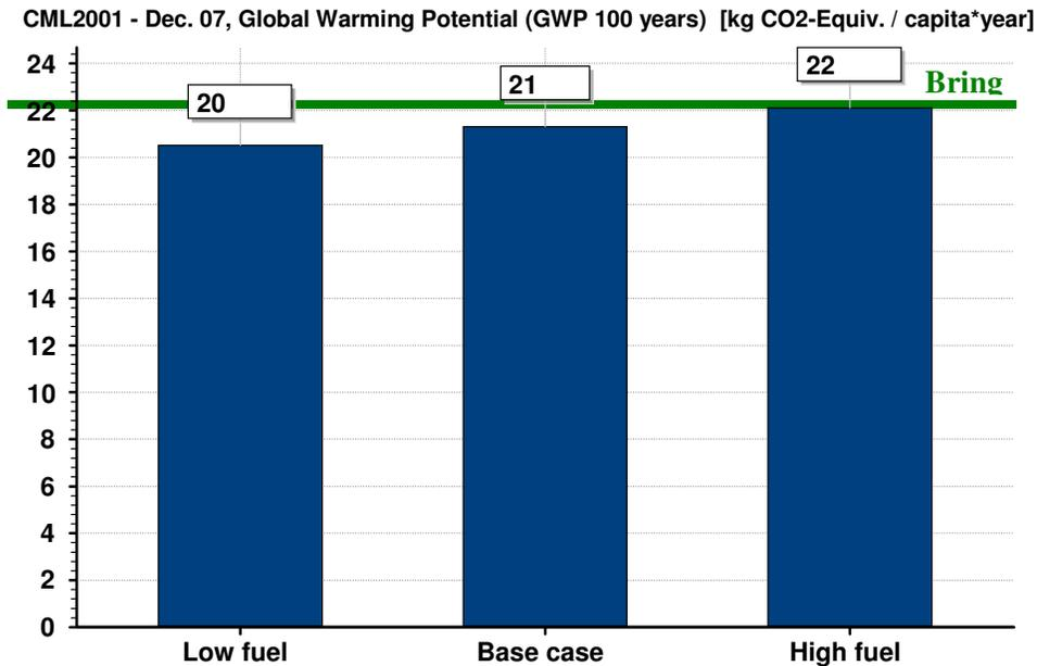
Figure 5.1 Emissions from co-mingled system with varied diesel consumption for the collection truck. The low fuel scenario use 19.76 litres per tonne; the base case use 22.29 litres per tonne and the high fuel scenario use 24.74 litres per tonne.
