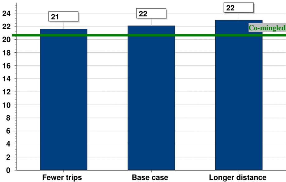
Figure 5.3 Emissions from bring system with varied car transport to recycling site. The fewer trips scenario has a distance of 2km and 12 trips per year; the base case has a distance of 2km and 25 trips per year while the longer distance scenario has a distance of 4km and 25 trips per year.
