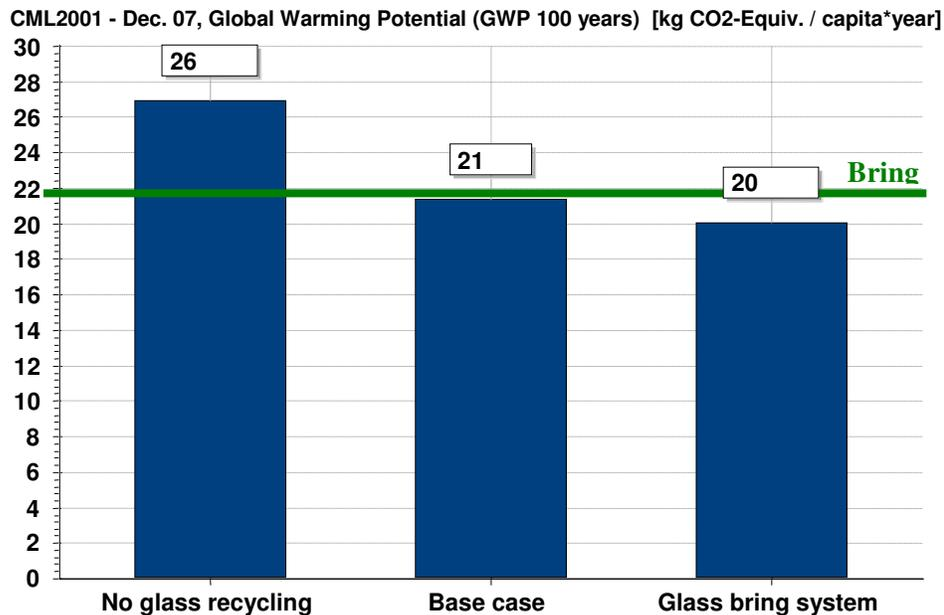
Figure 5.6 Emission with different glass scenarios in co-mingled collection. In the no glass recycling case glass is collected co-mingled and then landfilled; in the base case glass is collected co-mingled and recycled and in the glass bring system case, glass is collected separately in a bring collection.
