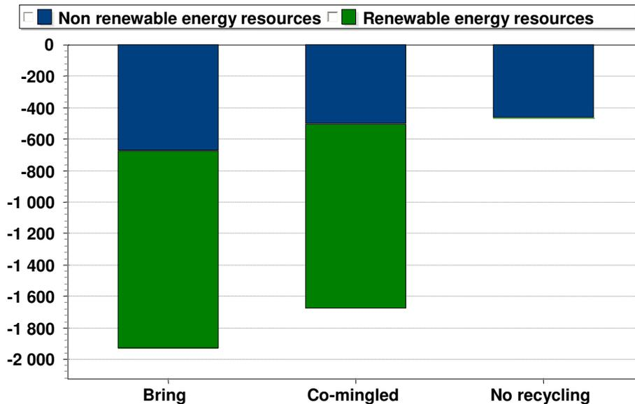
Figure 4.2 Primary energy demand in gross calorific value for complete collection systems. Divided into renewable and non renewable energy sources. Recyclables have not been included as an energy source.
