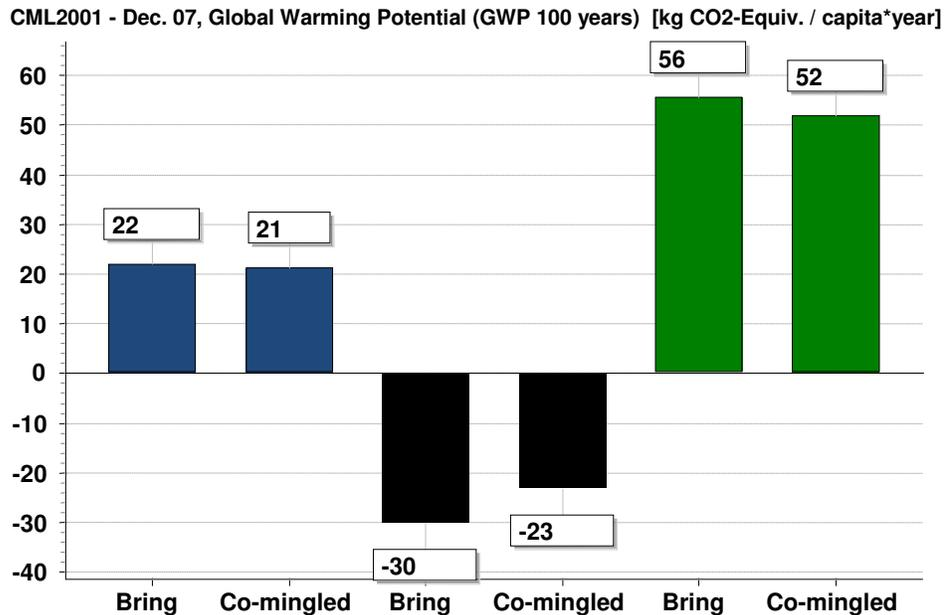
Figure 5.4 Emissions with electricity from natural gas (the first two blue bars), coal (the middle two black bars) and average Swedish electricity (the last two green bars).
