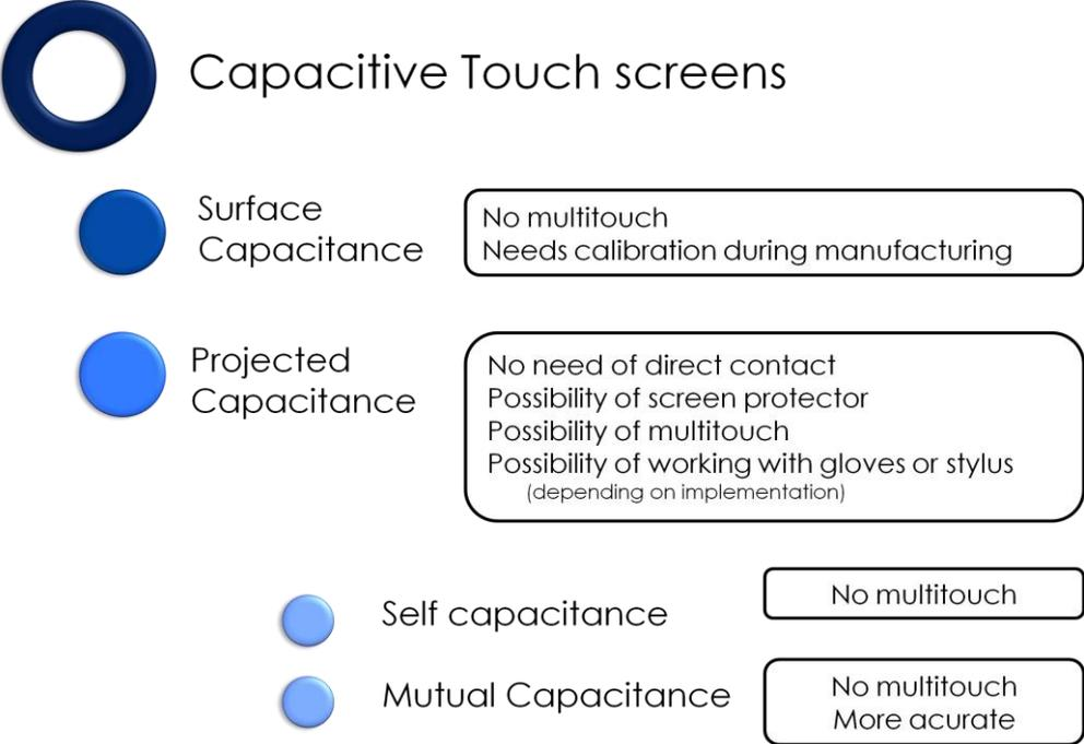
Figure 2.1 Types of capacitive touch screens.
