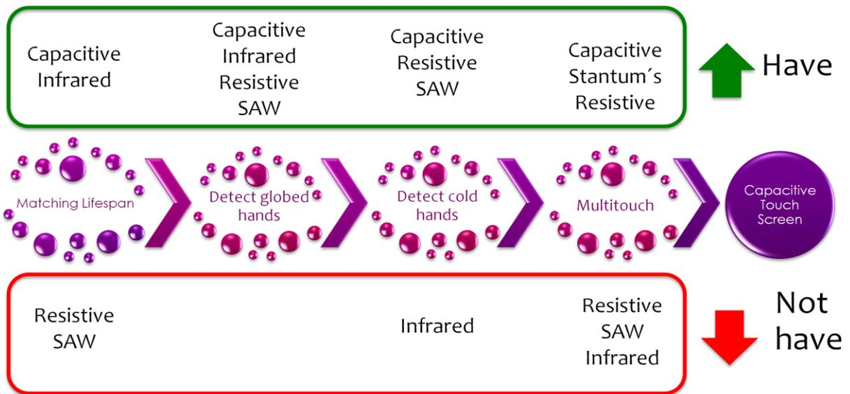
Figure 3.1 Requisites for an in-vehicle touch screen
