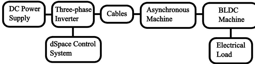
Fig. 6.4: Block diagram of the physical drive system setup.
