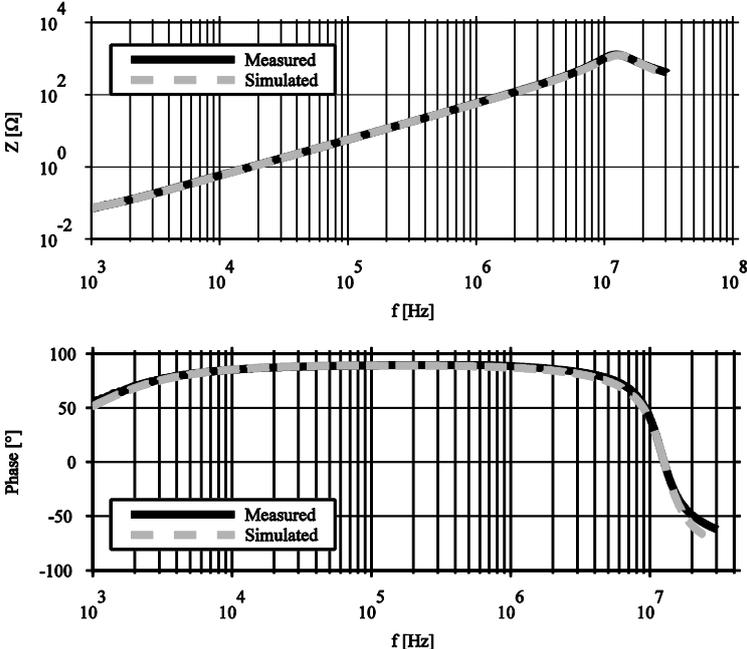
Fig. 5.3: The impedance and phase plot of the measured and modeled inductor ( $10\mu H$ ).
