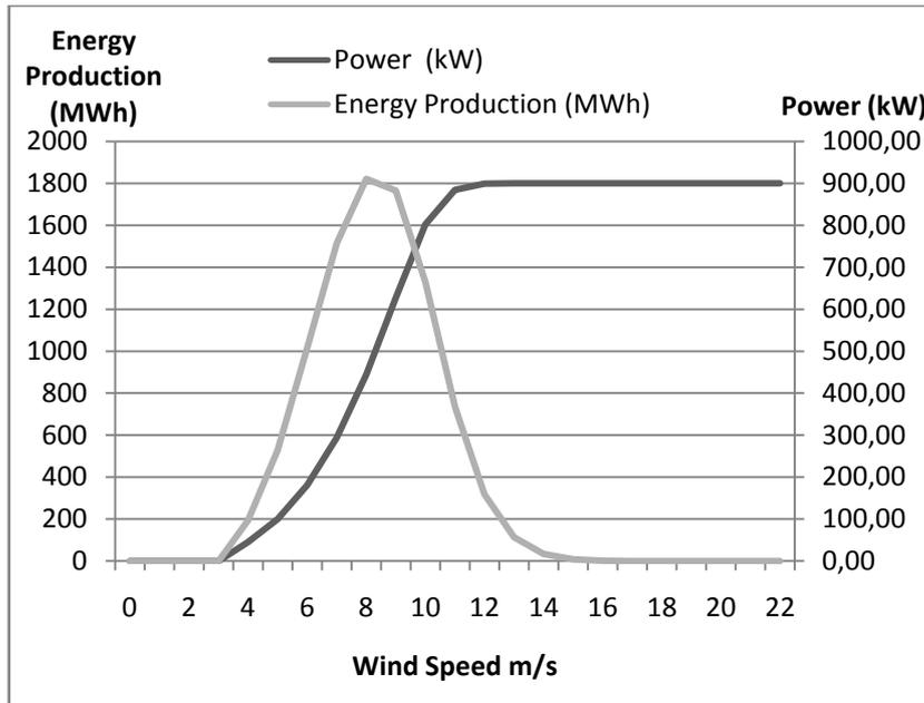
Figure11. This Figure shows the power output at different wind speeds and, combined with the wind speed allocation in Figure10, the total energy production for the different wind speeds.
