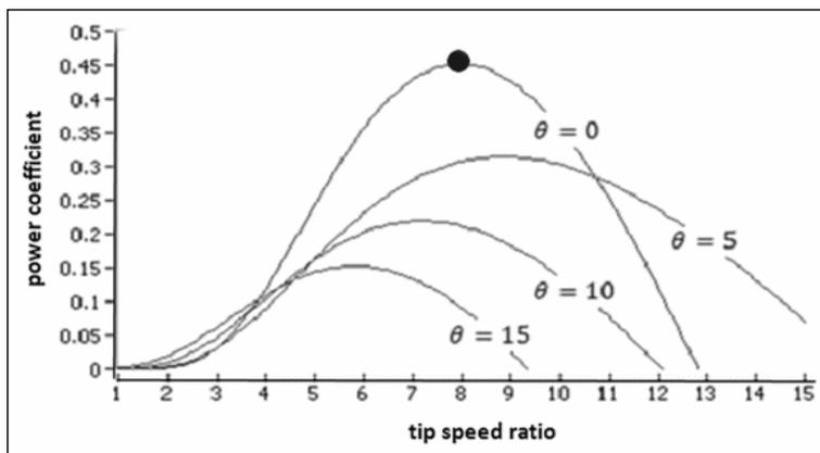
Figure12. Power coefficient at varying tip speed ratios and pitch angles.
