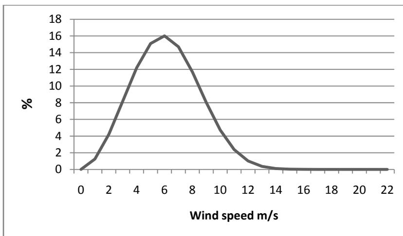
Figure10. Distribution of wind speed during one year at a specific location.
