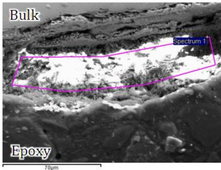
Figure 26 SEM image of the corrosion products on copper from Modification C.
