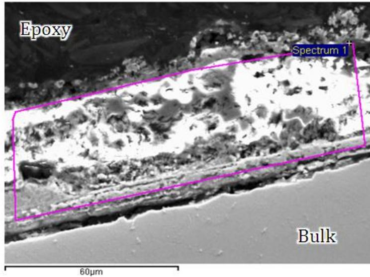
Figure 23 Cross section of copper coupon that has been exposed to Modification B.
