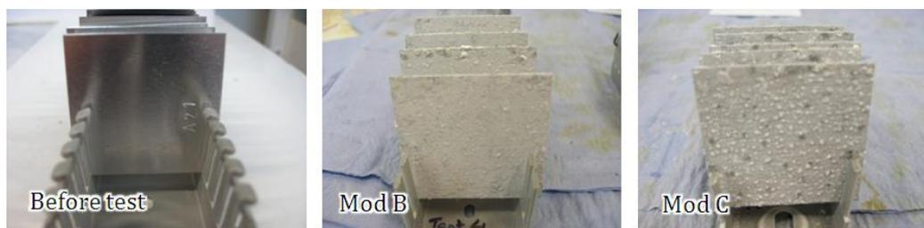
**Figure 5** Pictures of before and after test ISO 21207 method B, Modification B (Mod B) and Modification C (Mod C) of aluminum coupons.
