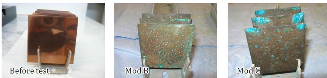
**Figure 10** Pictures of copper coupons before and after test ISO 21207 method B Modification B (Mod B) and Modification C (Mod C).
