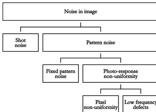
Figure 2.1 A hierarchical view of the noise components in an image captured by a digital camera
