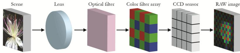
Figure 2.2 Digital camera pipeline
