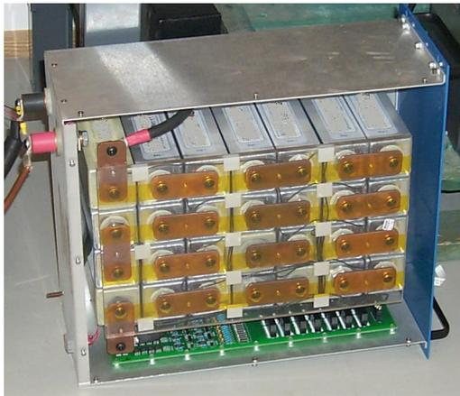
**Figure 5.8** EC bank with active balancing simulated in the *Size II* system.
