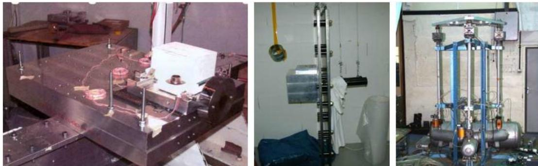
Figure 10 Example of metal-to-metal impact STFs a) mono-plate b) bi-plate c) tunable plate [16]
