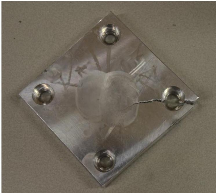
Figure 115 Cracked anvil plate
