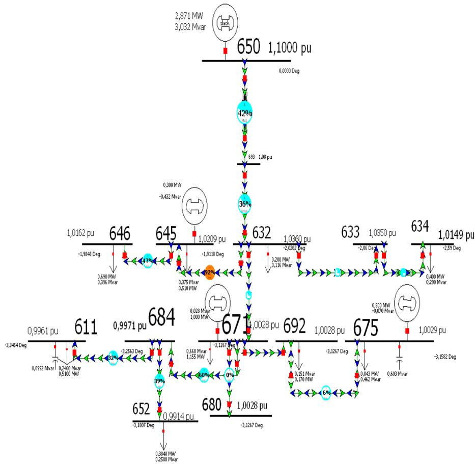
Figure 28: Over view of the IEEE 13- Node test system with some modification.
