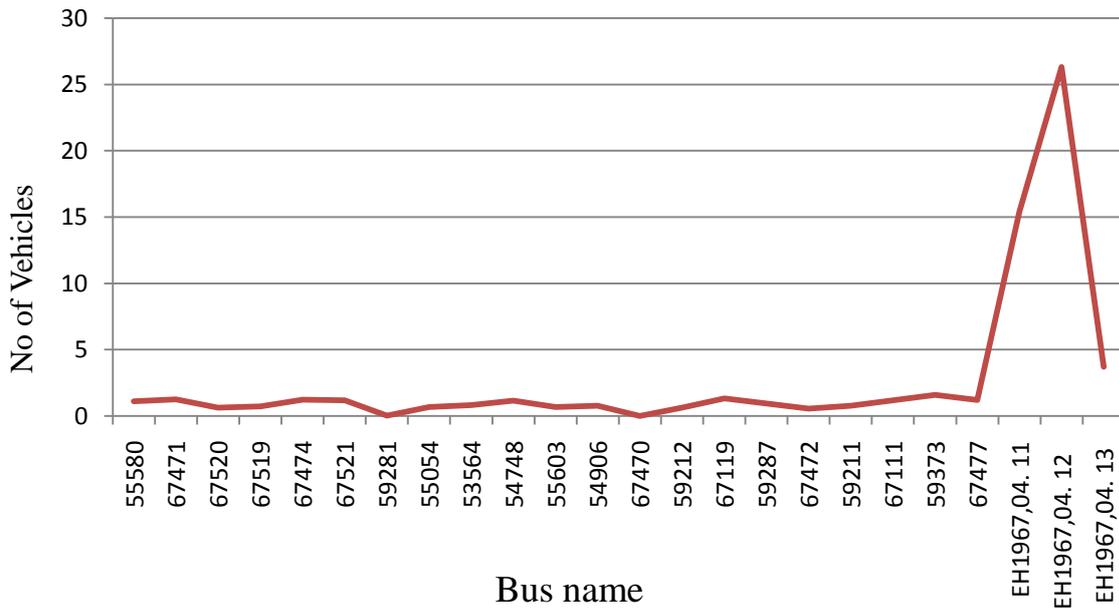
Figure 9: Calculated probable number of vehicles at substation RS1 only for transformer 2
