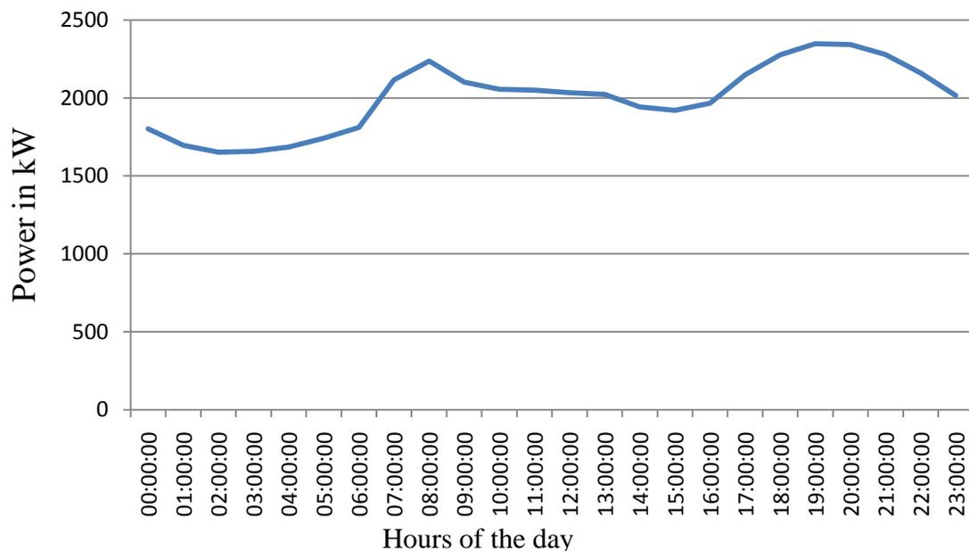
Figure 7: Load profile of a day in the winter for line RF1
