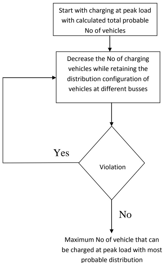
Figure 18: flow chart for calculation maximum possible charging
