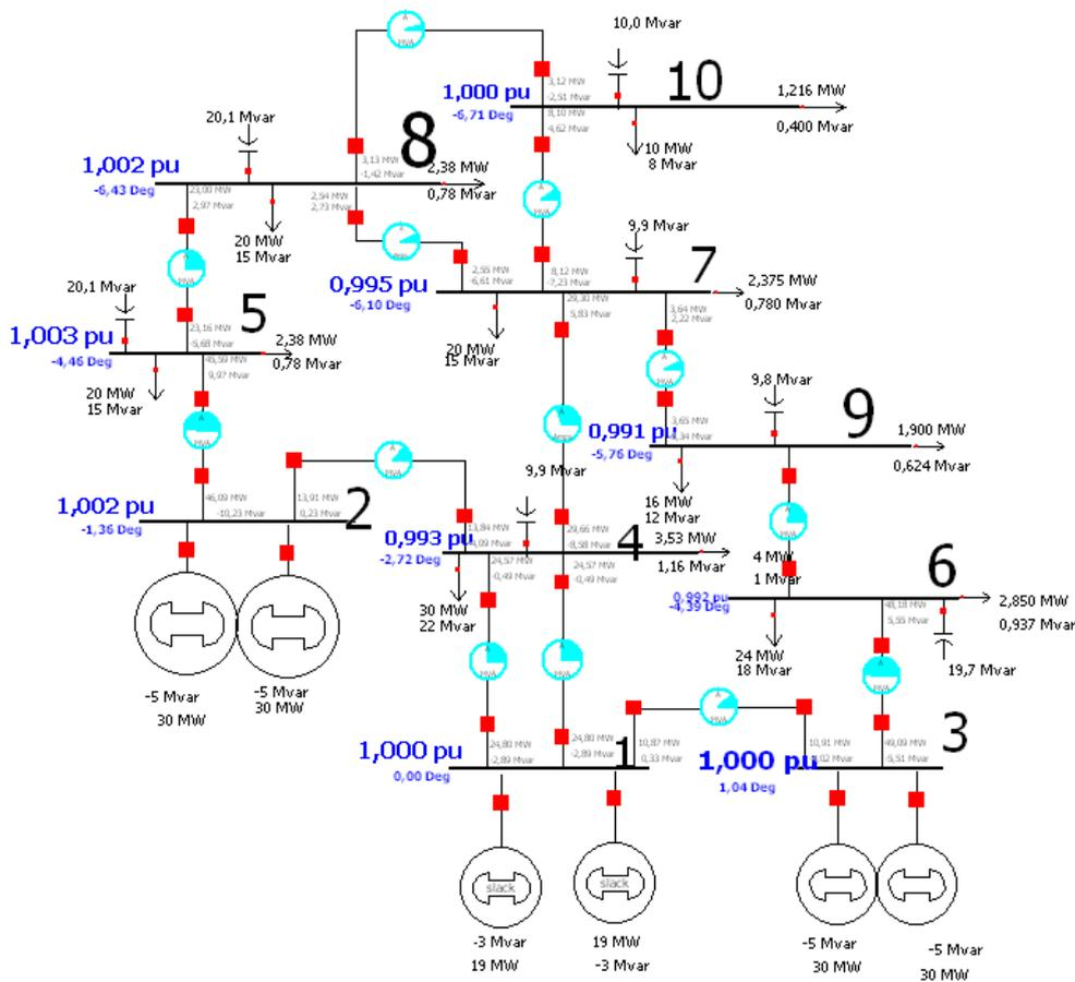
Figure 22: Single line of 10 bus test system
