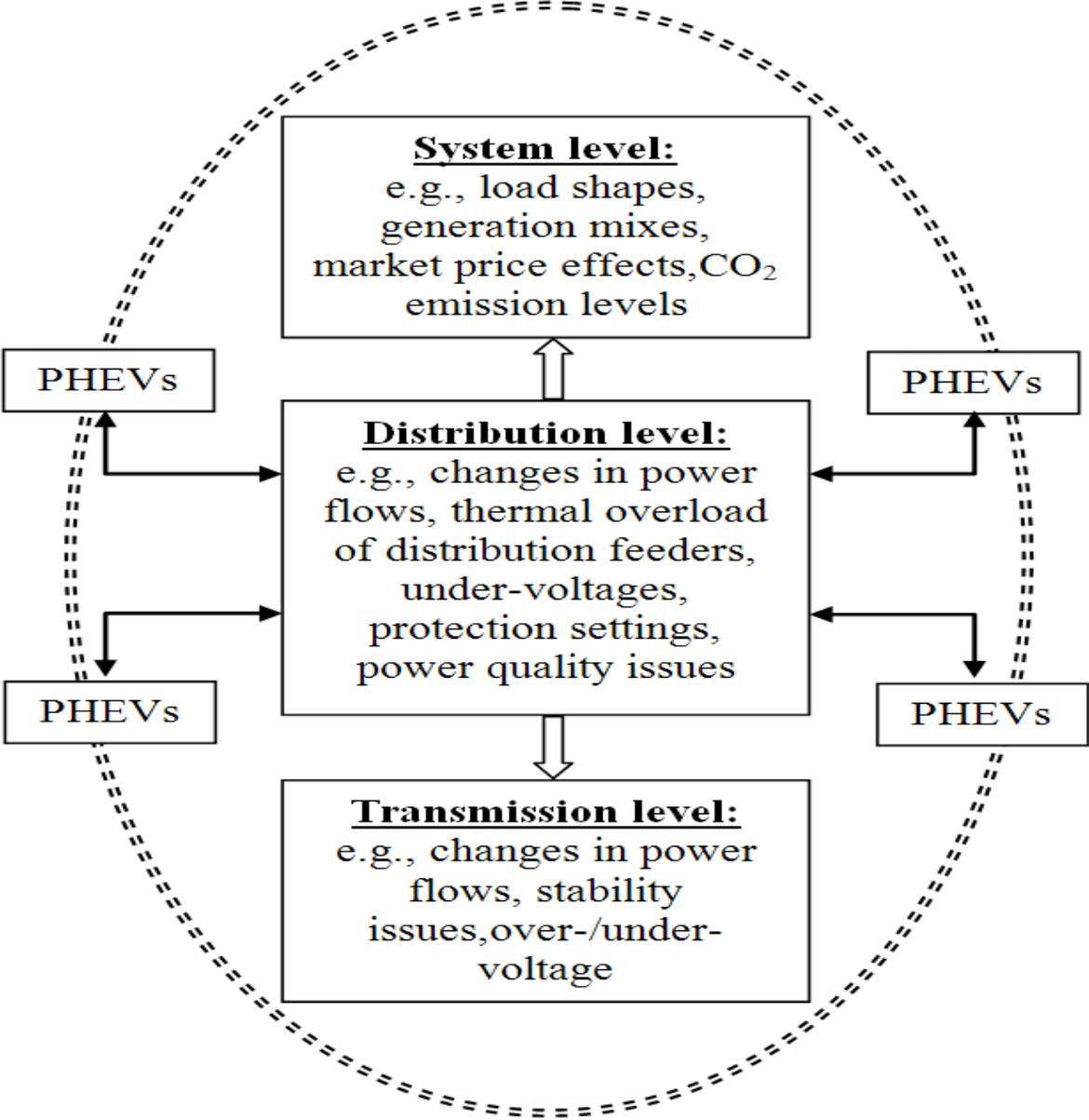
Figure 1: Overview of possible effects of PHEVs on power systems
