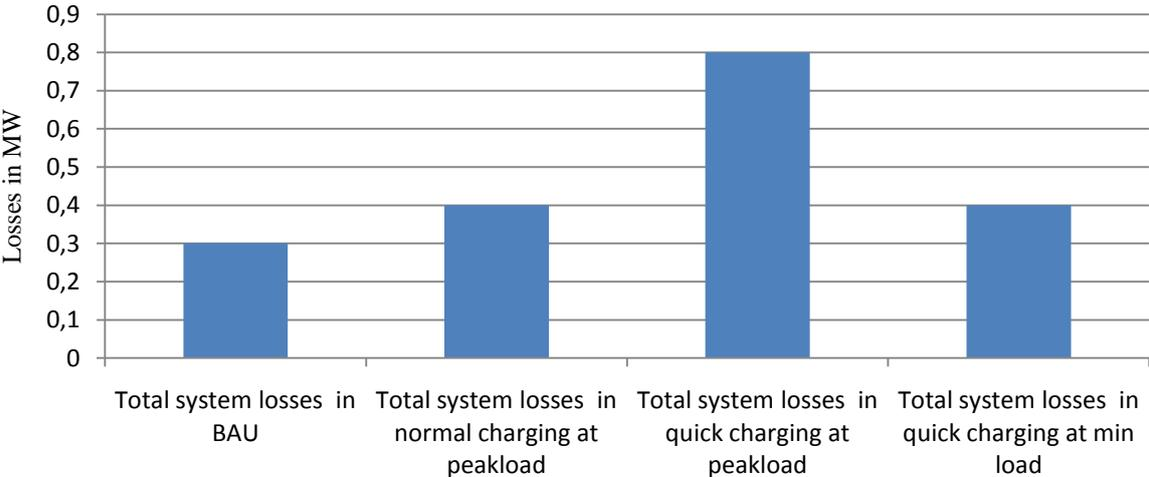
Figure 6: Total system active power losses
