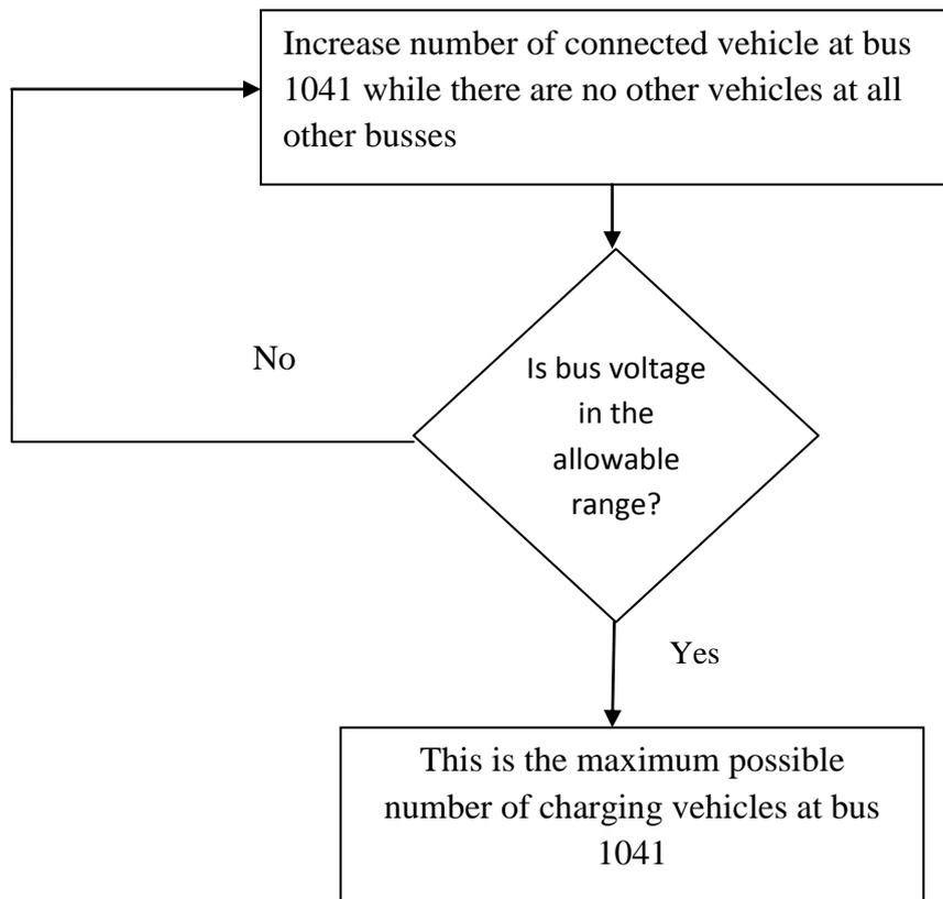
Figure 27: Iterative method for calculation maximum possible charging at one bus
