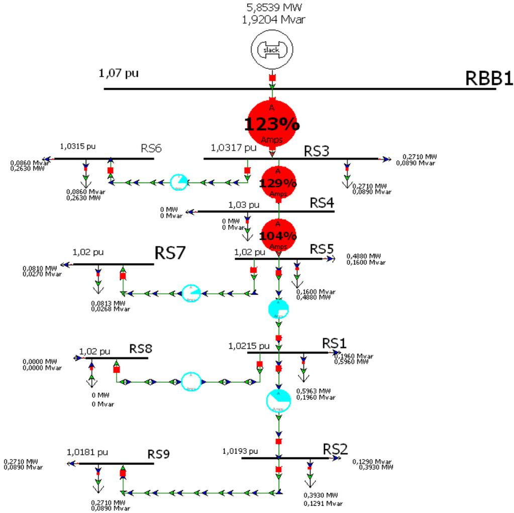
Figure 17: single line diagram of the 10 kV residential network in the Gothenburg
