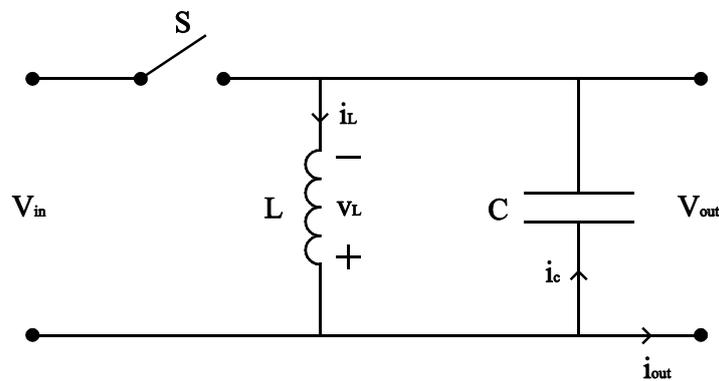
Figure 2.7 Circuitry when the switch is off.
