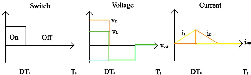
Figure 2.9 Switch, voltage and current waveforms in DCM
