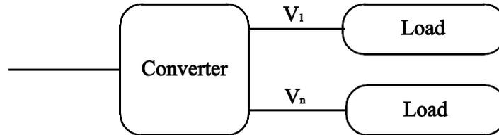
Figure 2.2 Centralized power architecture block diagram
