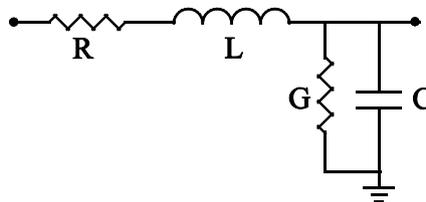
Figure 2.11: Equivalent model of the behaviour for a cable
