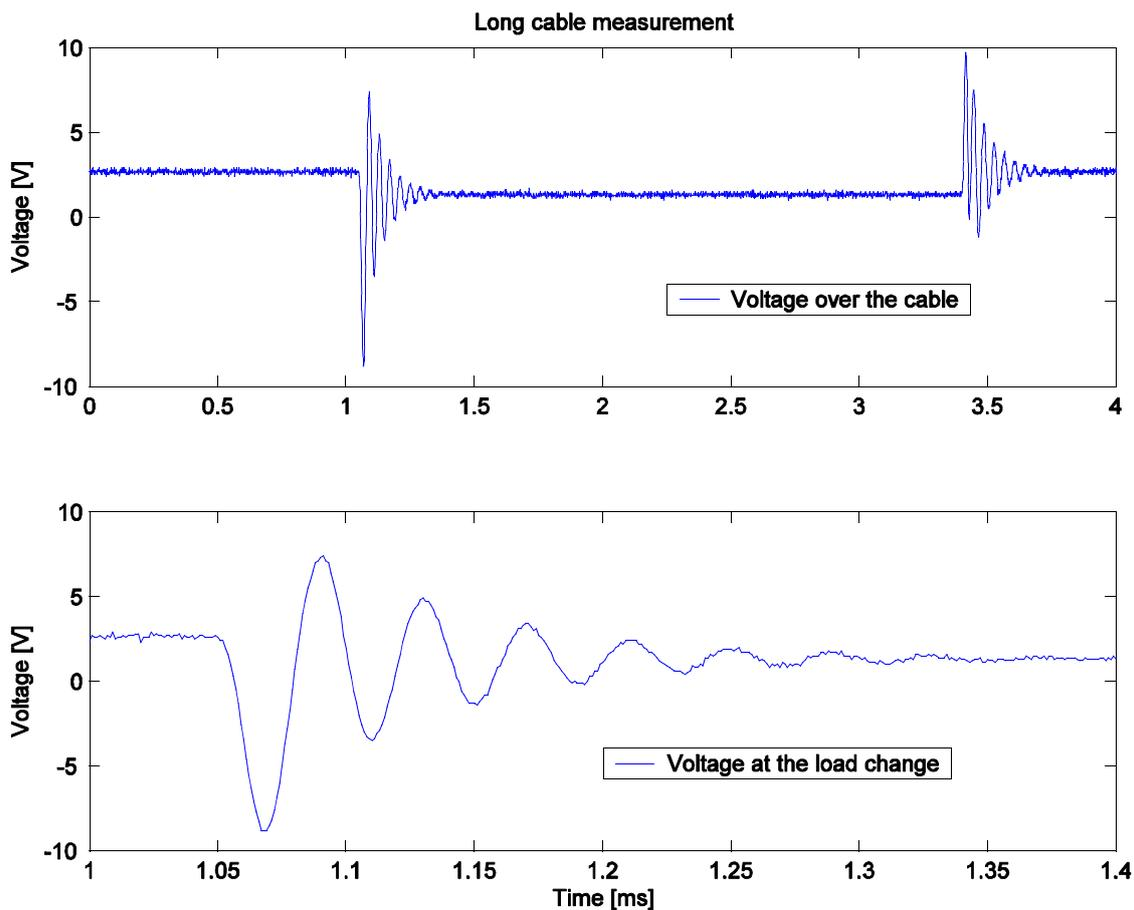
Figure 4.2 Long cable voltage measurement during a 2A to 1A pulsed load, and then back to 1A.
