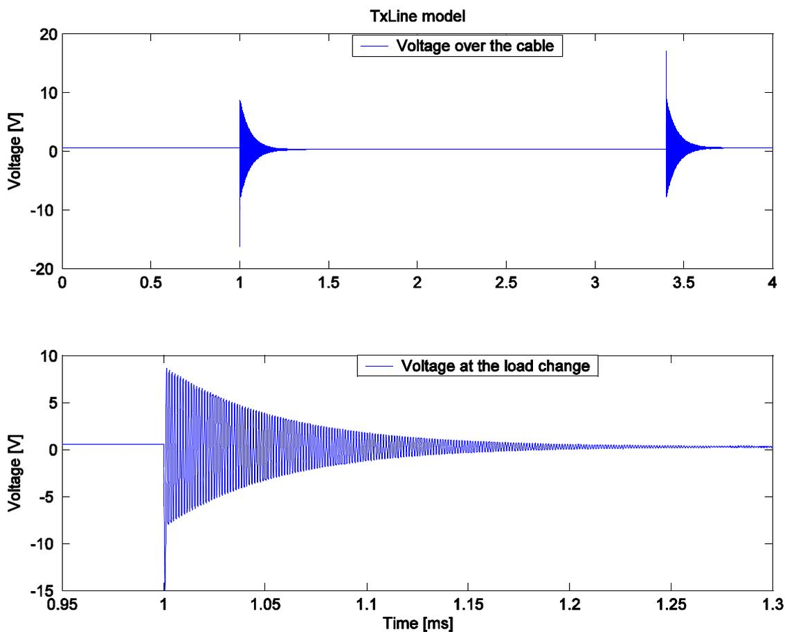
Figure 4.5 TxLine tool model simulation 1-2A pulsed current load
