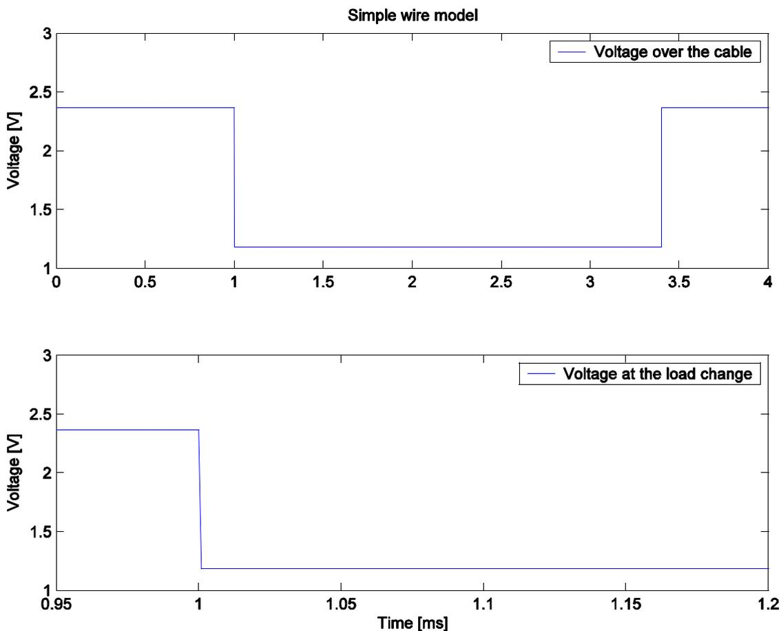
Figure 4.3 Simple wire model simulation, 1 – 2A pulsed current load
