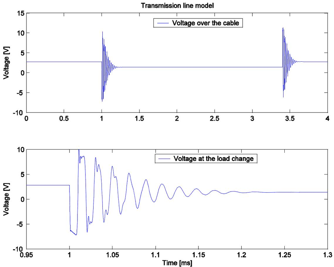
Figure 4.4 Transmission line model simulation, 1 – 2A pulsed current load
