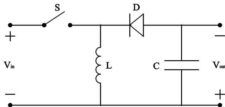
Figure 2.5 Buck boost converter topology
