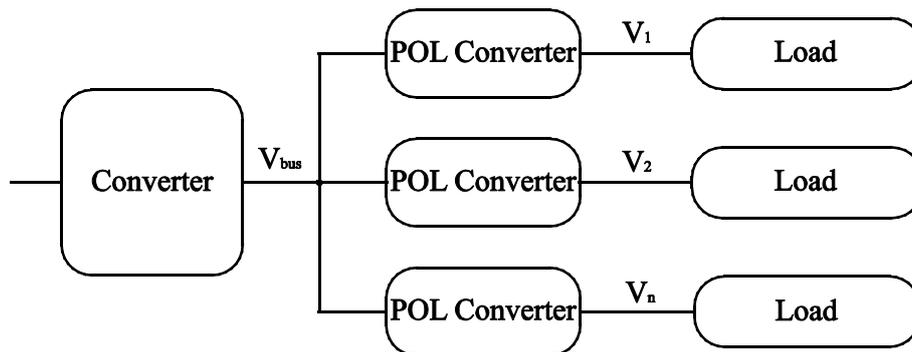
Figure 2.3 Distributed power architecture block diagram
