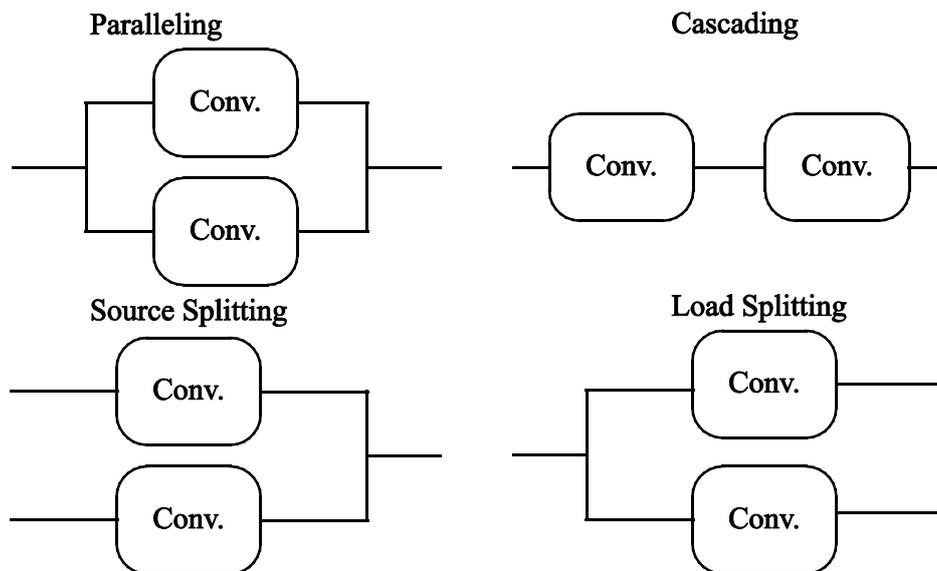
Figure 2.1 Distributed power system structures, Paralleling, Cascading, Load splitting and source splitting
