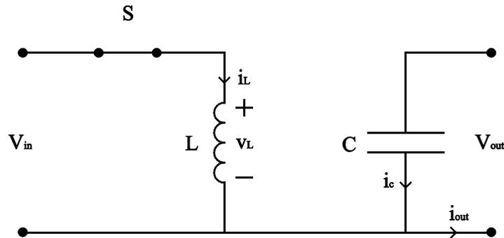
Figure 2.6 Circuitry when the switch is on.
