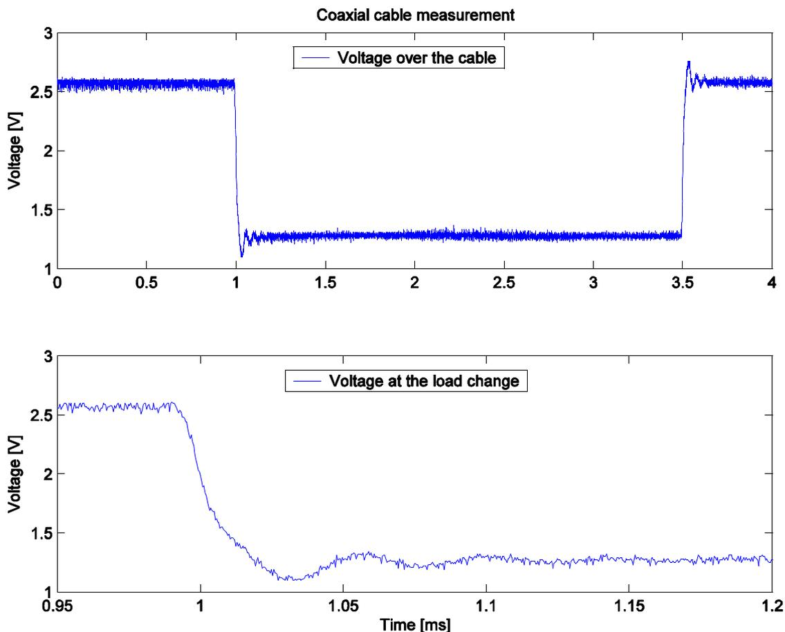
**Figure 4.7:** The voltage over a coaxial cable during the switching with a pulsed load. The top graph is during 4 milliseconds, and the bottom one is zoomed from 0.95milliseconds to 1.2 milliseconds.
