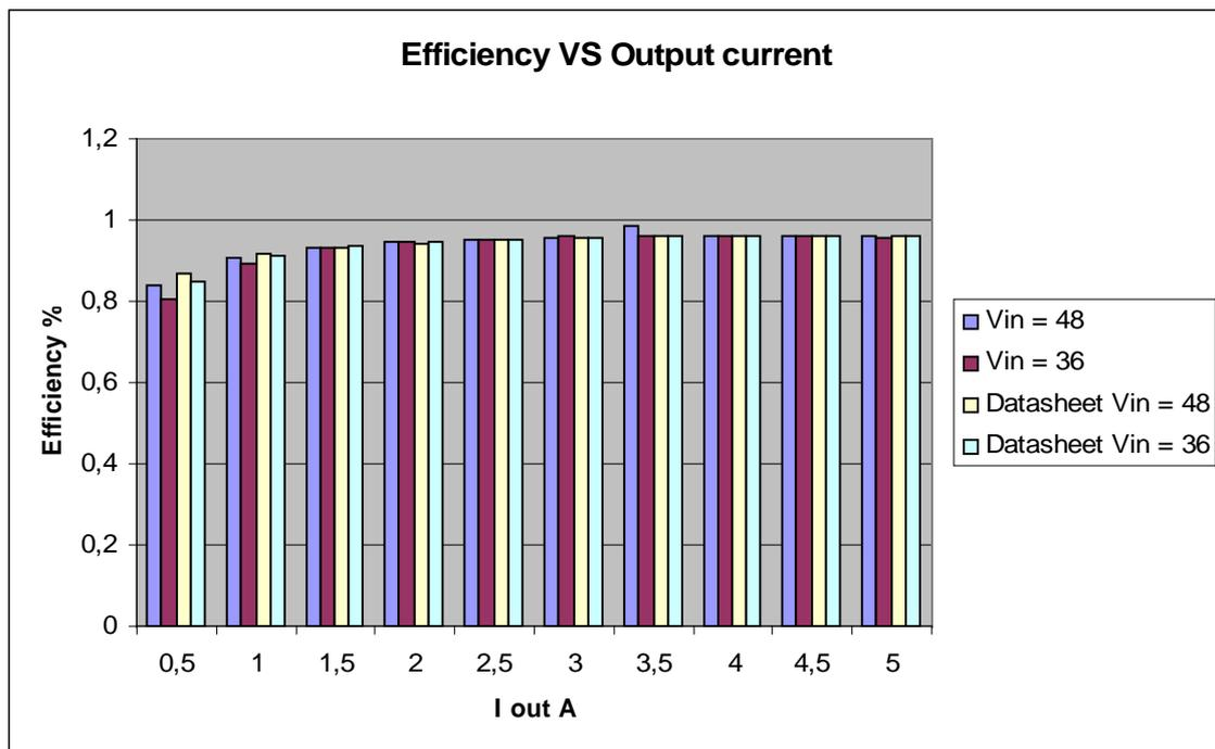
Figure 5.4: Efficiency versus output current
