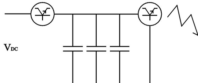
**Figure 6.3 Approximate radar wave transmission circuit**
