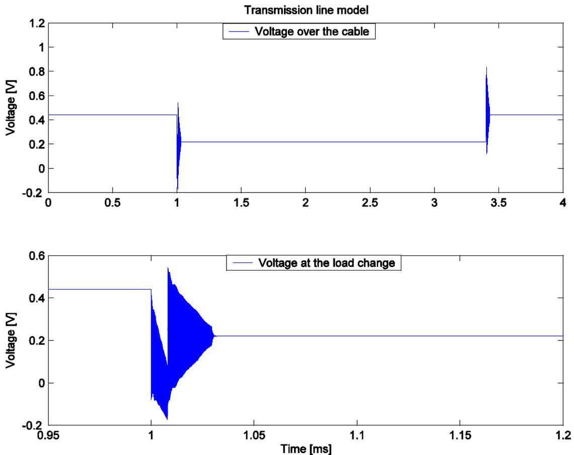
**Figure 4.8:** The voltage over a coaxial cable with a pulsed current load. Top graph shows the 4 milliseconds, and the bottom one is zoomed between 0.95 milliseconds and 1.2 milliseconds.
