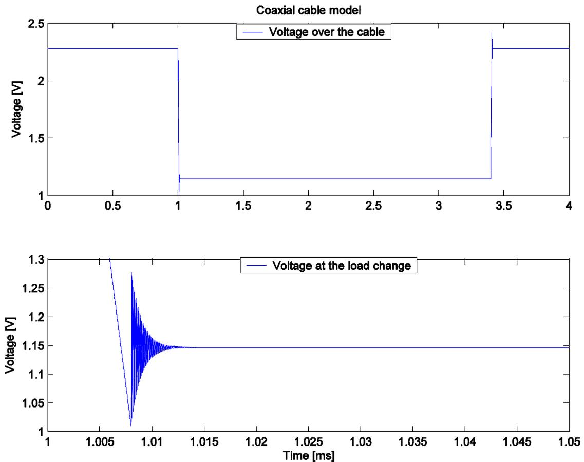
**Figure 4.9: Voltage over the coaxial cable model during a pulsed load. Top graph shows 4 milliseconds, and the bottom graph is zoomed from 1 millisecond to 1.05 milliseconds.**
