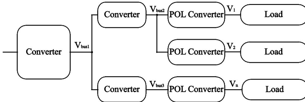
Figure 2.4 Intermediate bus architecture block diagram
