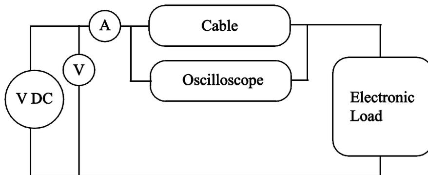
**Figure 4.1 Cable measurement setup**
