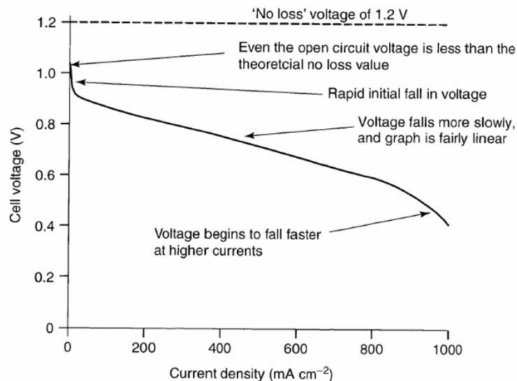
**Figure 19.** Voltage-current density diagram for a low temperature, air pressure fuel cell. Courtesy of John Wiley & Sons Limited [P1].
