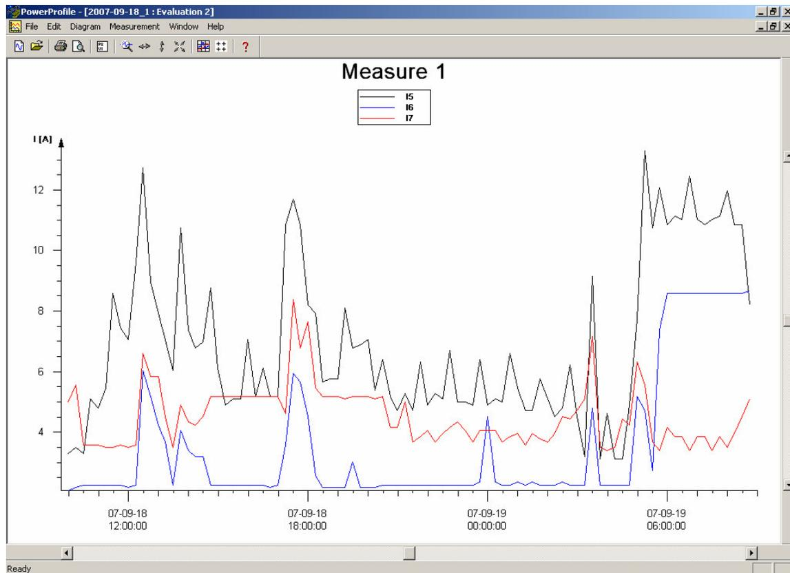
**Figure 16.** Data from the generator three phase current measurement.
