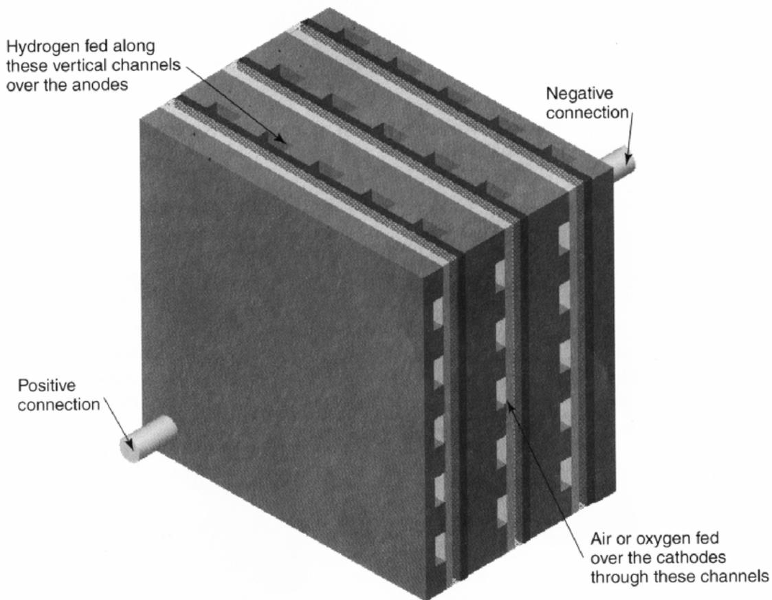
**Figure 6.** A fuel cell stack, consisting of three cells connected with bipolar plates.
