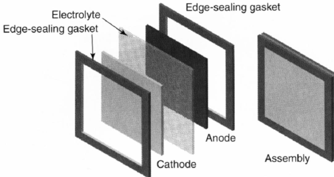
**Figure 7.** Structure of a fuel cell with edge seals to prevent leakage of the gas at the edges of the electrodes. Courtesy of John Wiley & Sons Limited [P1].
