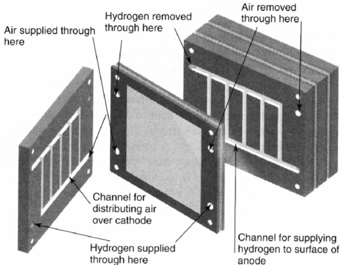
**Figure 9.** Fuel cell stack with internal manifolding. A more complex bipolar plate is used to allow the reactant gases to be fed to the electrodes through internal channels.
