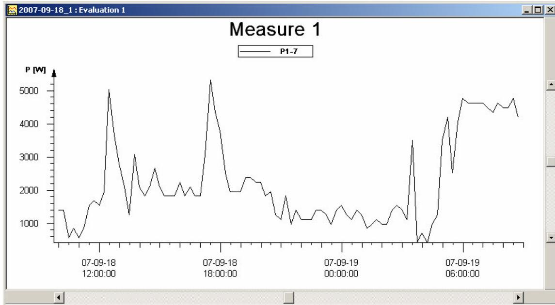
Figure 17. Power consumption for a one day and night sailing trip.
