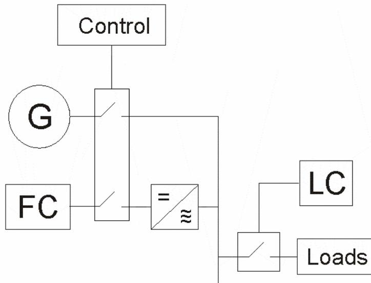
**Figure 25.** Block diagram of the fuel cell and generator hybrid system, where FC are the Fuel cells, G is the generator and LC is the load control. This is a simplified schematic of the three phase part of the system.
