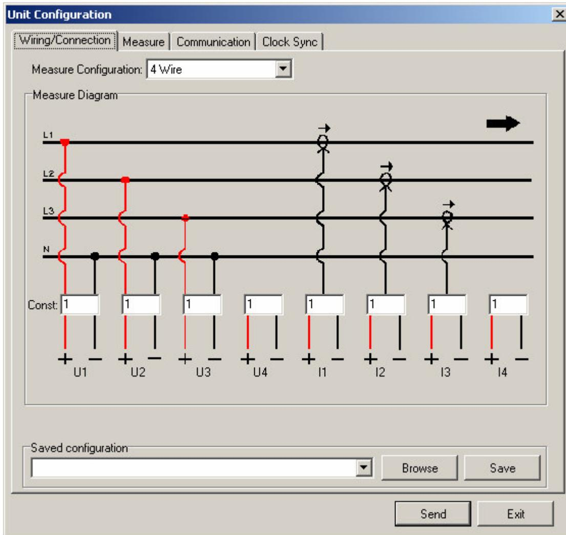
**Figure 13.** Unit configuration where different kind of wiring and connection settings can be made.
