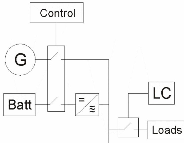
**Figure 26.** Block diagram of the battery and generator hybrid system, where G is the generator, Batt are the batteries and LC is the load control. This is a simplified schematic of the three phase part of the system.
