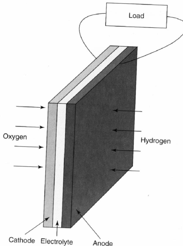
**Figure 1.** Basic structure of a fuel cell. Courtesy of John Wiley & Sons Limited [P1].
