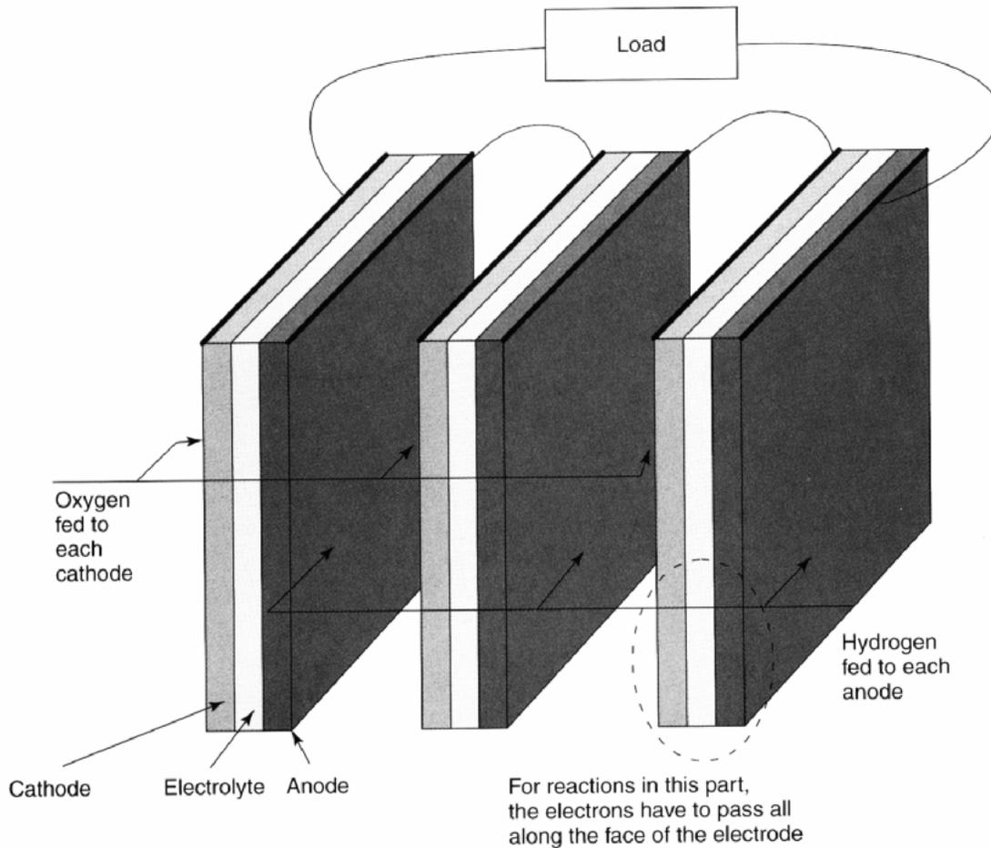
**Figure 5.** Simple series connection from the anode of one cell to the cathode of the next one. Courtesy of John Wiley & Sons Limited [P1].
