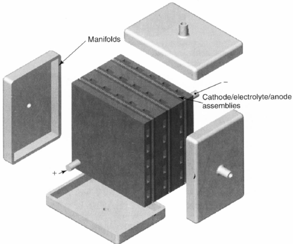
**Figure 8.** Fuel cell stack with external manifolding. Courtesy of John Wiley & Sons Limited [P1].
