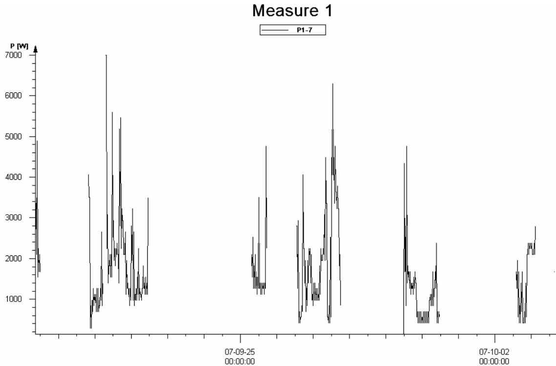
**Figure 20.** Power measurement during a 14 day period. The periods without measurements occurred when the ship was at harbor where the generator is not used.
