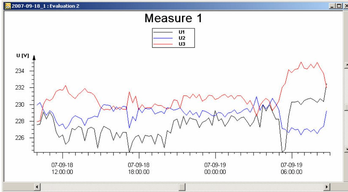
**Figure 15.** Example on how a measurement presentation in PowerProfile looks like. In this case the presented parameters are the phase voltages from the generator in the ship.
