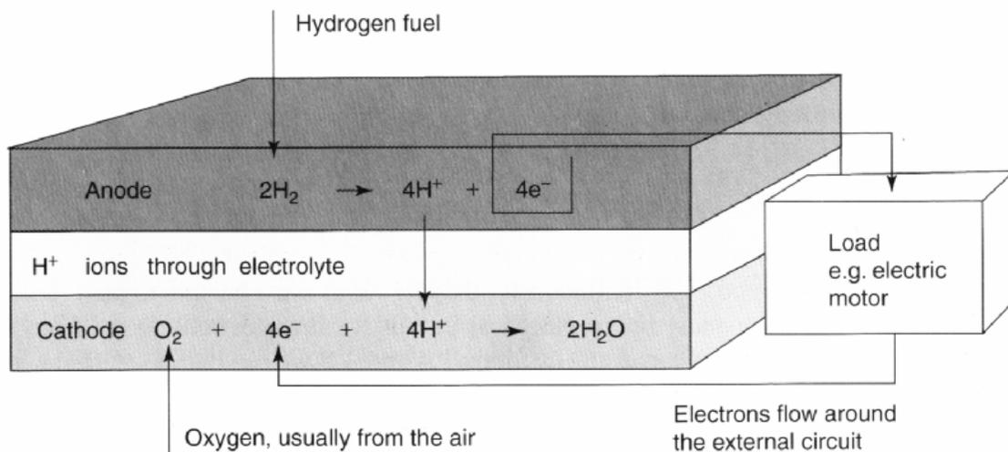
**Figure 2.** Electrode reactions and electrical flow for an acid electrolyte fuel cell. The electrons flow from the anode to the cathode via an external circuit. Courtesy of John Wiley & Sons Limited [P1].
