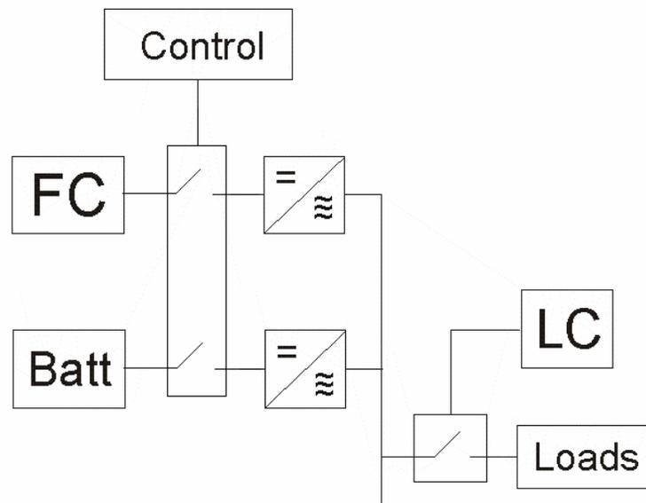
**Figure 27.** Block diagram of the fuel cell and battery hybrid system, where FC are the Fuel cells, Batt are the batteries and LC is the load control. This is a simplified schematic of the three phase part of the system.
