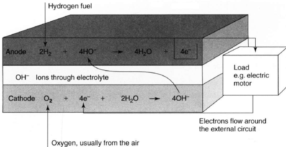
**Figure 3.** Electrode reactions and electrical flow for an alkaline electrolyte fuel cell.
