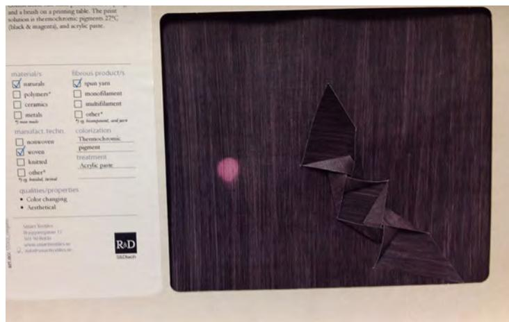
Wall paper sample which changed when the sun heated it up. It means that the environment of the ward could change depending on the sun and light coming through the windows
