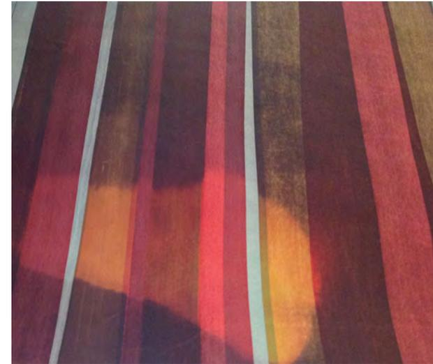
The fabric, whose color changes according to changes of temperature. The heat makes it fade away, which could be very easily factor in determining room temperature in a hospital ward
