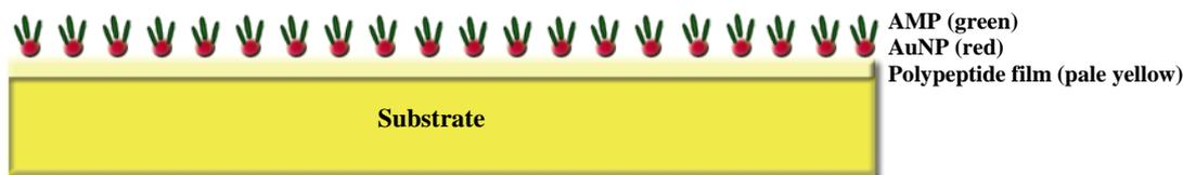
*Figure 1: A polypeptide coated substrate with attached AuNPs and AMPs.*
