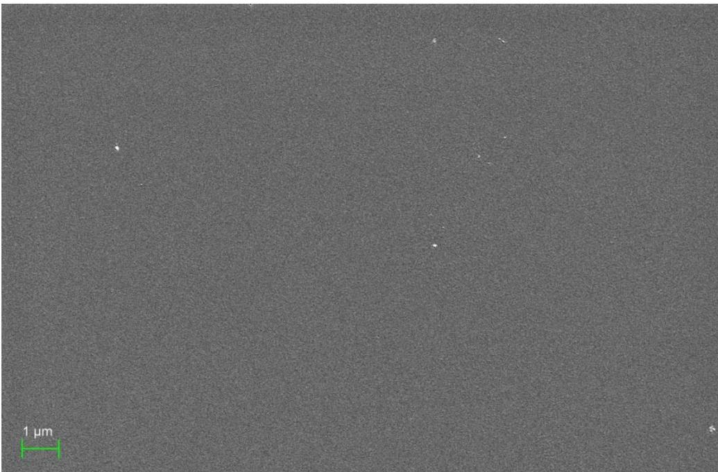
**Figure 4:** AuNPs on PMMA substrate, reference surface. The PMMA substrate was cleaned with ethanol.
