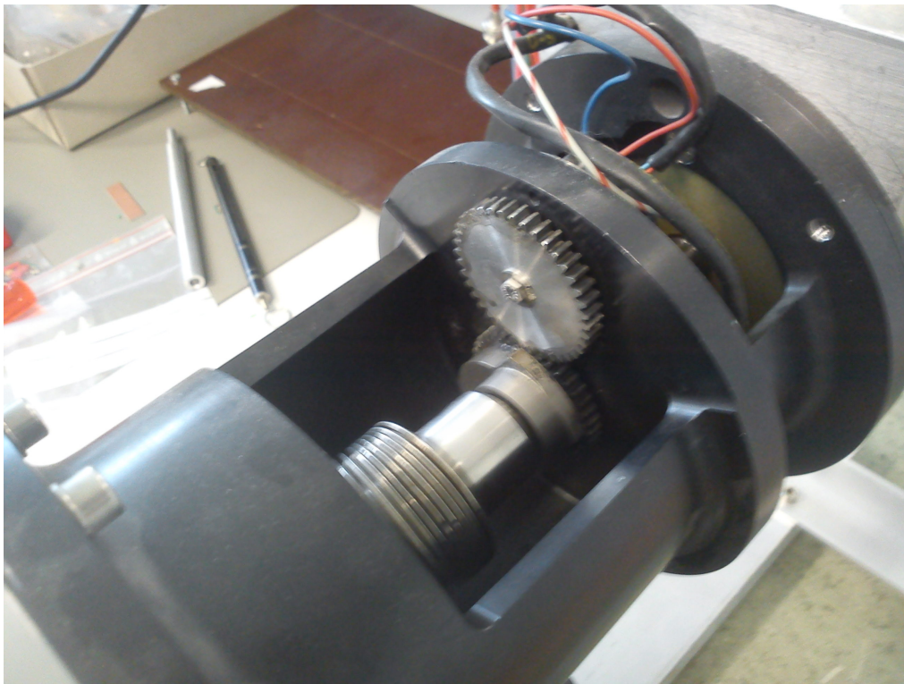
Figure 1.2.3: Actuator feedthrough of the rotary wire scanner used in the Super Proton Synchrotron (SPS) at CERN. To the left, the bellows are shown and to the right the gear transferring the motion from the motor shaft to the scanner shaft is visible.
