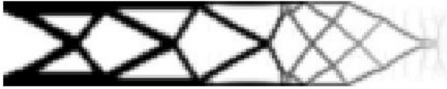
Figure 4.4.1: 2D topology optimisation for a volume fraction of 0.3. The fork base is located to the left
