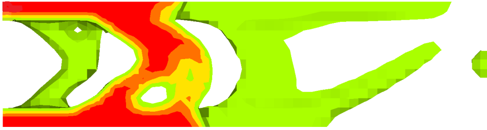
Figure 4.4.4: "Optimised" design of the fork using a parallelepiped design space.
