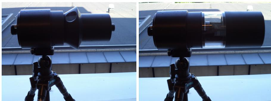
Figure 6: The old conical scanner with a rotating hood and a small quartz window can be seen to the left and the prototype scanner with a non-rotating quartz window can be seen to the right.
