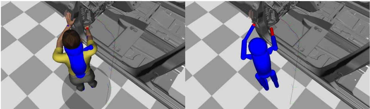
Figure 31: Shows a collision between the manikin and the car with (left figure) and without the manikin mesh rendered (right figure). The blue figure shows the collision model of the manikin and the red part indicates where the collision occurs.
