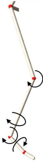
Figure 10: A close up of a leg in the manikin skeleton. The knee rotates around one axis, while the foot rotates around three.
