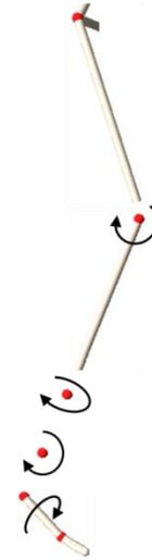
Figure 11: An exploded view of the leg in Figure 10. The knee is modeled with one link connecting the shin to the femur. Three links are used to model the ankle, in which two zero-length links are connected to the shin.
