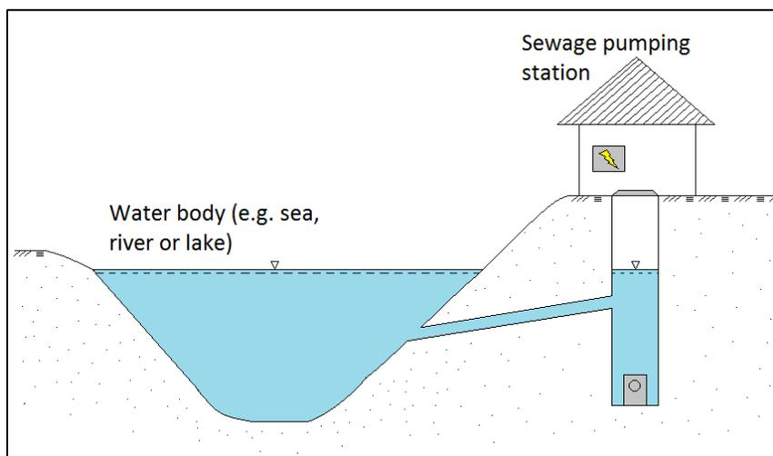
*Figure 11 The level to which the water rise in the chamber is limited by the water level of any connected water source*
