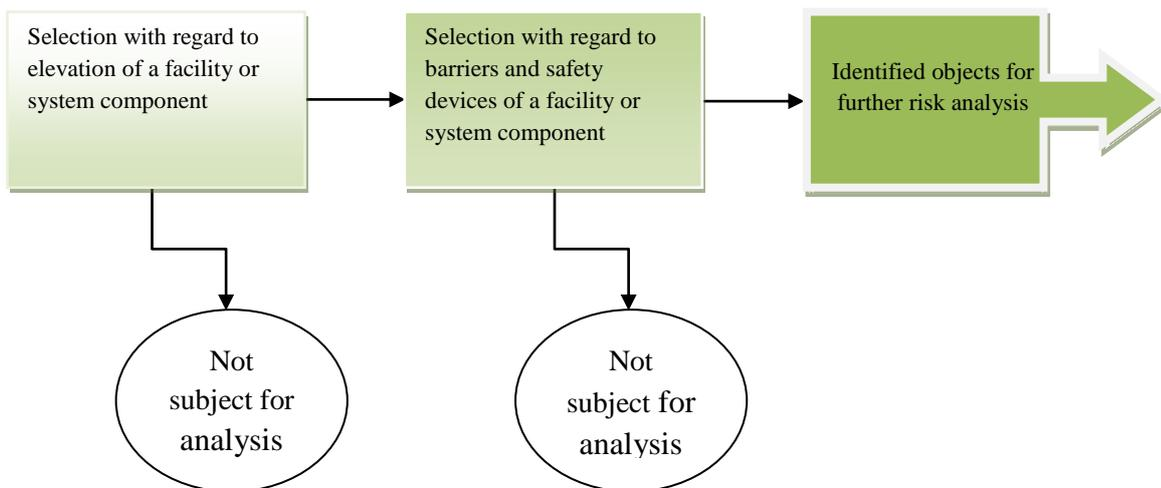
*Figure 3 Flow chart describing the selection process for facilities and system components*
