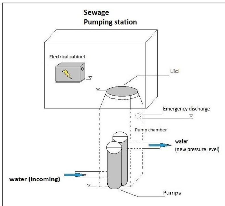
Figure 12 Schematics for sewage pumping stations with the electrical cabinet located above the lid of the pumping chamber
