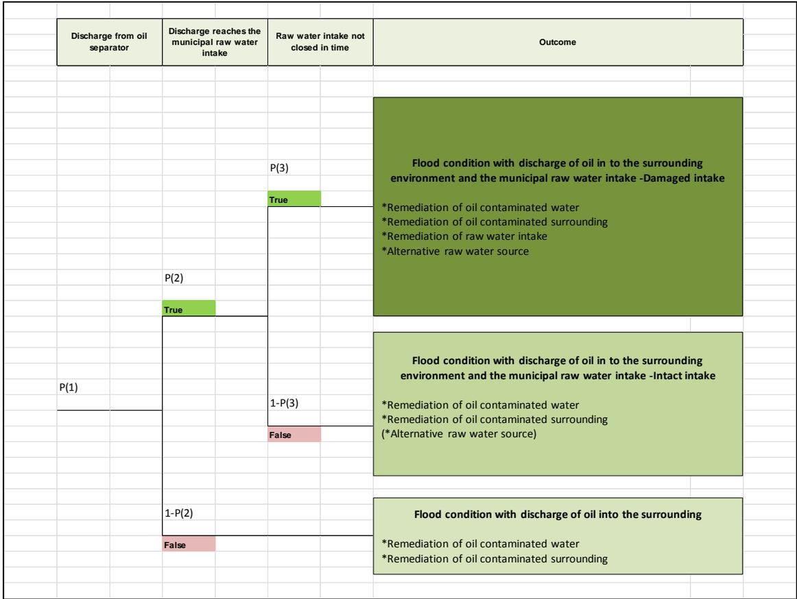
Figure 34 Event tree for the oil separator at Alelyckan recycling centre
