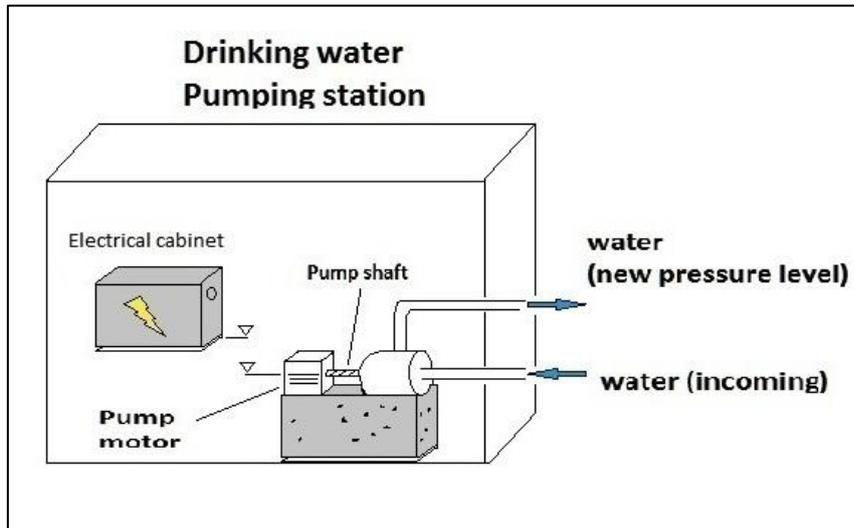
Figure 9 Schematics for drinking water pumping stations with the electrical cabinet located above the pump shaft
