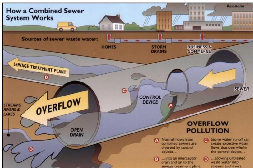
Figure 7 Schematic description of a typical CSO (NYDEC, 2014)
