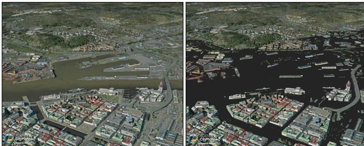
Figure 8 The Frihamnen area in central Gothenburg: to the left normal water conditions at + 0 m and to the right extreme water level conditions at + 3.80 m (Agency9, 2014)
