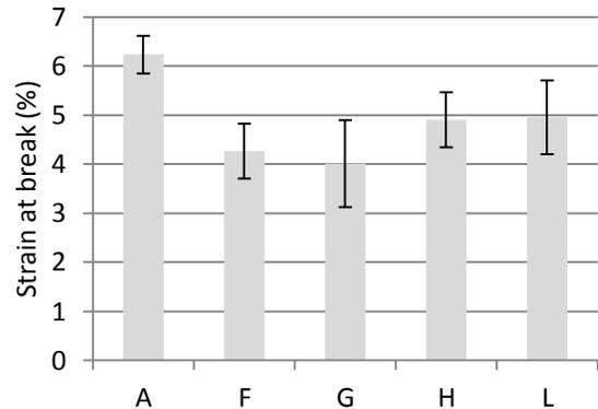
**Figure 4-9.** The elongation (%) of 200 g/m<sup>2</sup> sheets, compression moulded at 170°C. The error bars are projected at a 95% CI, n=8 apart from for A:n=32.
