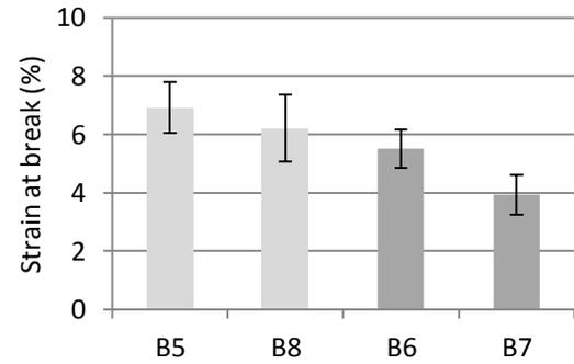
Figure 4-6. The elongation of composite specimens of sheet B, compression moulded at 170°C. The error bars are projected at a 95% CI. B5 and B8 are tensile tested at Innventia, and B6 and B7 at another laboratory, n=8.
