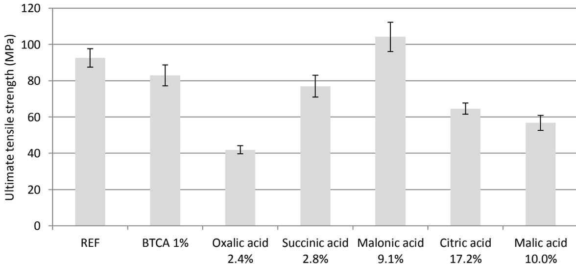
**Figure 4-11. The influence of acid concentration on ultimate tensile strength of test composites hot pressed at 170°C, 31.25 MPa for 15 min, compared to untreated reference samples of all-cellulose composites(n=32). The error bars are projected at a 95% CI, n=8 for all acid-treated composites.**
