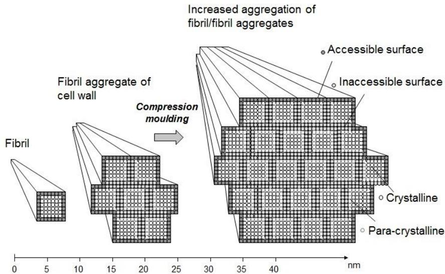
Figure 2-5. A representation of fibril (4 nm width) aggregation to larger fibril aggregates (mean width 20nm) (Halonen, 2012).
