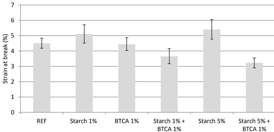
**Figure B2-4.** The elongation (%) obtained from the physical modification by starch, combined with the chemical modification of BTCA, compression moulded at 170°C at 31.25 MPa for 15 min, compared to untreated reference samples of all-cellulose composites(n=32) . The error bars are projected at a 95% CI, n=8, for all additive-treated composites.
