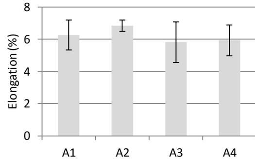
**Figure 4-3.** The elongation (%) within sheet A, compression moulded at 170°C. The error bars are projected at a 95% CI, n=8.
