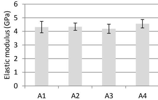
**Figure 4-2.** The module (GPa) within sheet A, compression moulded at 170°C. The error bars are projected at a 95% CI, n=8.
