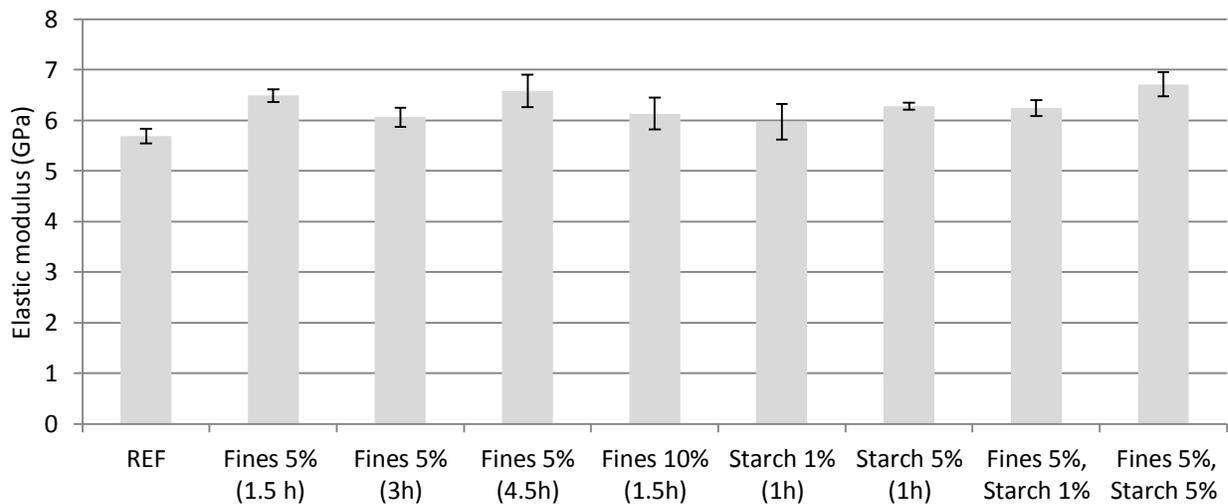
**Figure B2-1.** The values of modulus (GPa) obtained from the physical modification by starch and fines compression moulded at 170°C at 31.25 MPa for 15 min, compared to untreated reference samples of all-cellulose composites(n=32) . The error bars are projected at a 95% CI, n=8, for all additive-treated composites.
