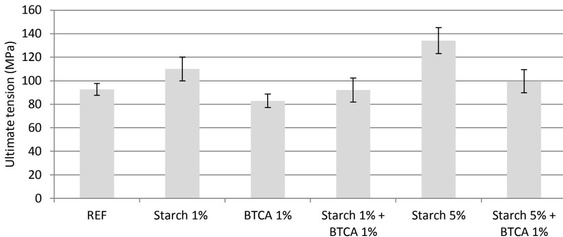
**Figure 4-21.** The ultimate stress data (MPa) obtained from the physical modification by starch, combined with the chemical modification of BTCA, compression moulded at 170°C. The error bars are projected at a 95% CI, n=8 apart from for the reference where n=32.
