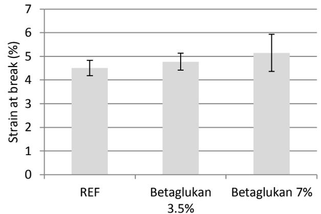
**Figure 4-20.** The elongation (%) obtained from the physical modification by beta-glucan, compression moulded at 170°C. The error bars are projected at a 95% CI, n=8 apart from for the reference where n=32.
