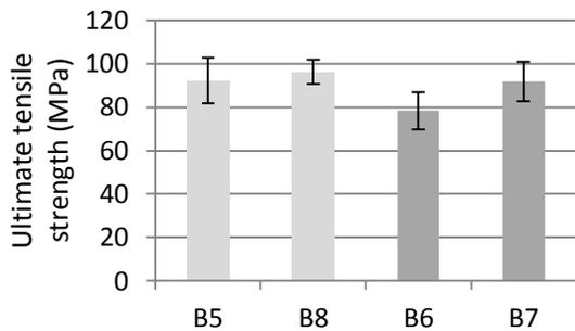
**Figure 4-4.** The ultimate tensile strength within sheet B, compression moulded at 170°C. The error bars are projected at a 95% CI. B5 and B8 are tensile tested at Innventia, and B6 and B7 at another laboratory, n=8.
