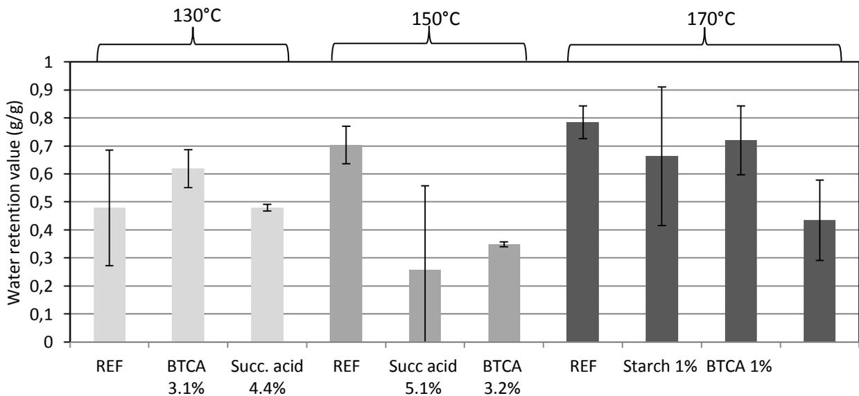
Figure 4-16. The water retention at three different temperature levels for curing at 15 min: 130°C (light gray), 150°C (medium gray) and 170°C (dark gray). Duplicates of each quality were made (n=2), and the error bars shows the standard deviation.
