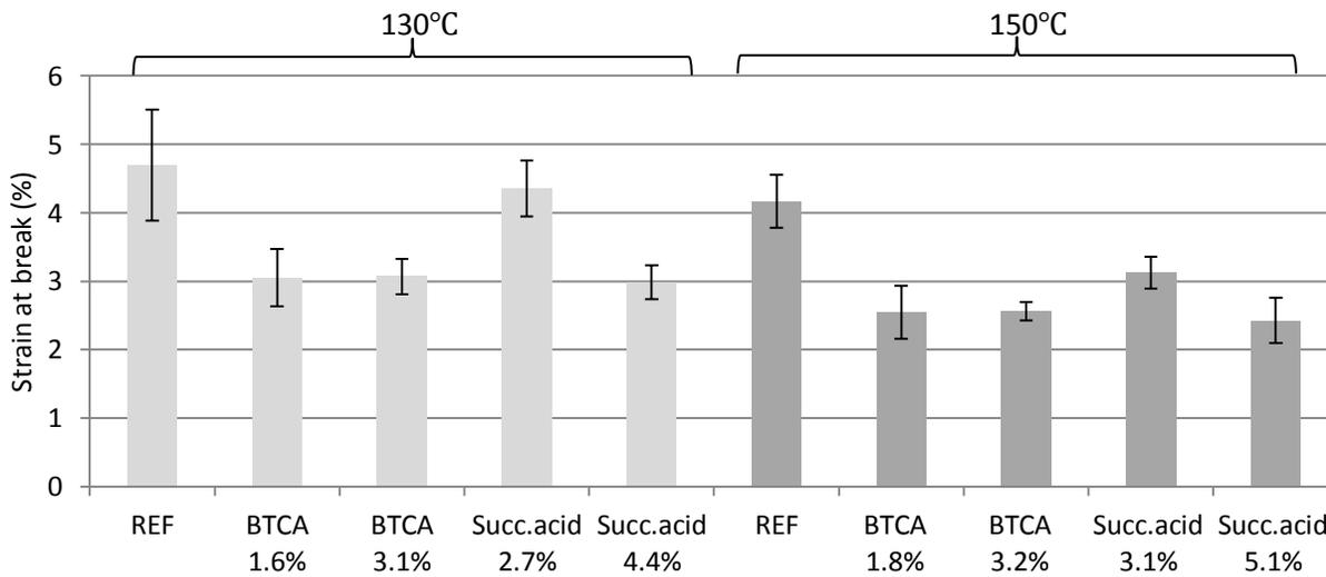
Figure B1-2. The influence of acid concentration on the elongation values of test composites hot pressed at two temperature levels, 130 and 150°C at 31.25 MPa for 15 min, compared to untreated reference samples of all-cellulose composites(n=8). The error bars are projected at a 95% CI, n=8 for all acid-treated composites.
