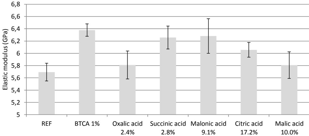
**Figure 4-12.** The influence of acid concentration on the elastic modulus values of test composites hot pressed at 170°C, 31.25 MPa for 15 min, compared to untreated reference samples of all-cellulose composites(n=32). The error bars are projected at a 95% CI, n=8 for all acid-treated composites.
