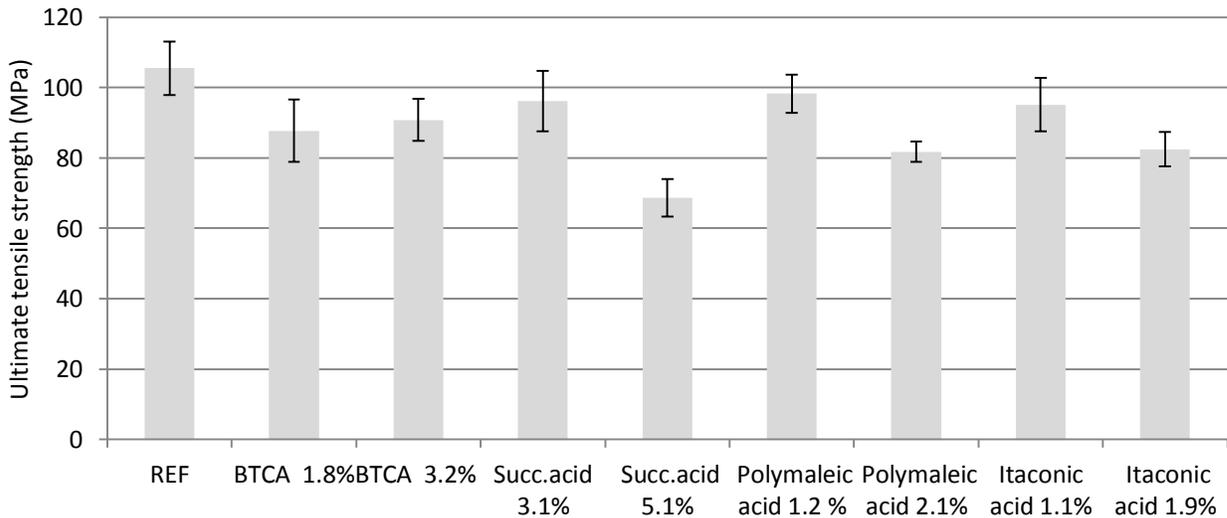
**Figure 4-15.** The influence of acid concentration on the ultimate stress values of test composites hot pressed at 150°C. The error bars are projected at a 95% CI, n=8.
