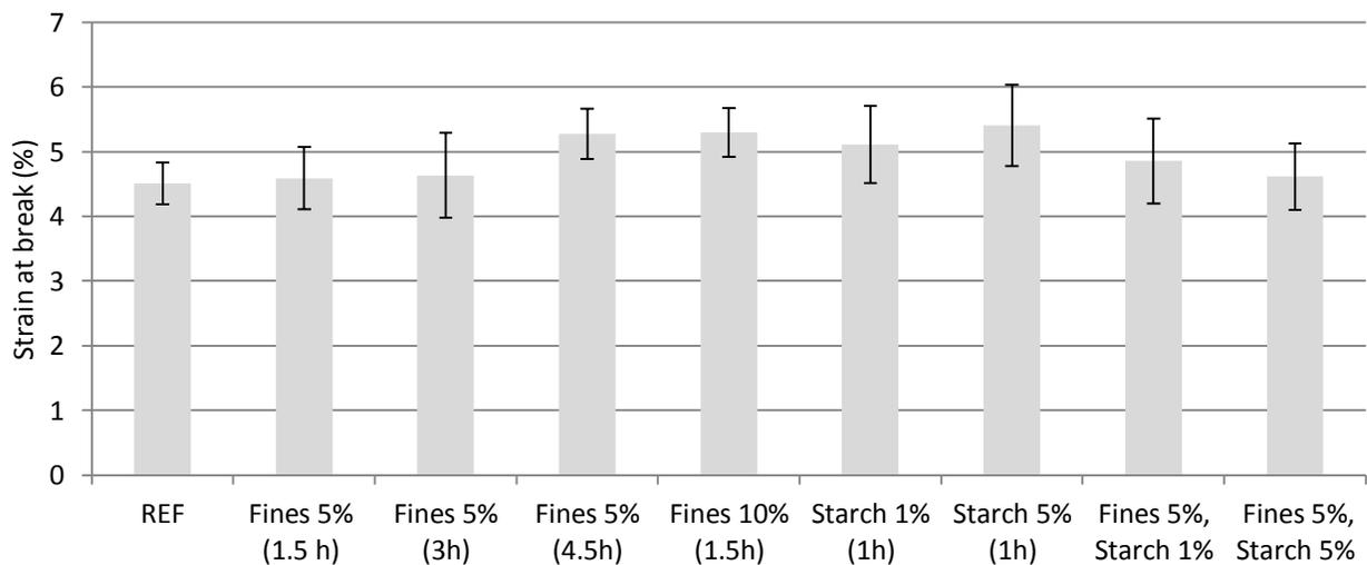
**Figure B2-2.** The values of elongation (%) obtained from the physical modification by starch and fines compression moulded at 170°C at 31.25 MPa for 15 min, compared to untreated reference samples of all-cellulose composites(n=32) . The error bars are projected at a 95% CI, n=8, for all additive-treated composites.
