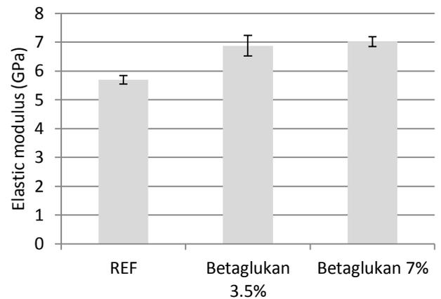
**Figure 4-19.** The modulus (GPa) obtained from the physical modification by beta glucan, compression moulded at 170°C. The error bars are projected at a 95% CI, n=8 apart from for the reference where n=32.
