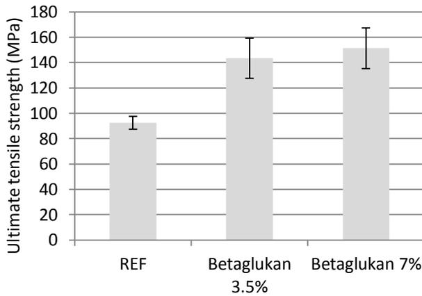
**Figure 4-18.** The ultimate tensile strength (MPa) obtained from the physical modification by beta glucan, compression moulded at 170°C. The error bars are projected at a 95% CI, n=8 apart from for the reference where n=32.
