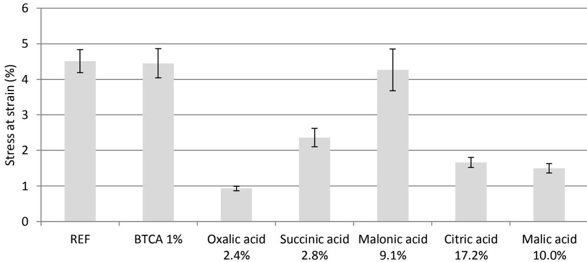
**Figure 4-13.** The influence of acid concentration on the elongation of test composites hot pressed at 170°C, 31.25 MPa for 15 min, compared to untreated reference samples of all-cellulose composites(n=32). The error bars are projected at a 95% CI, n=8 for all acid-treated composites.
