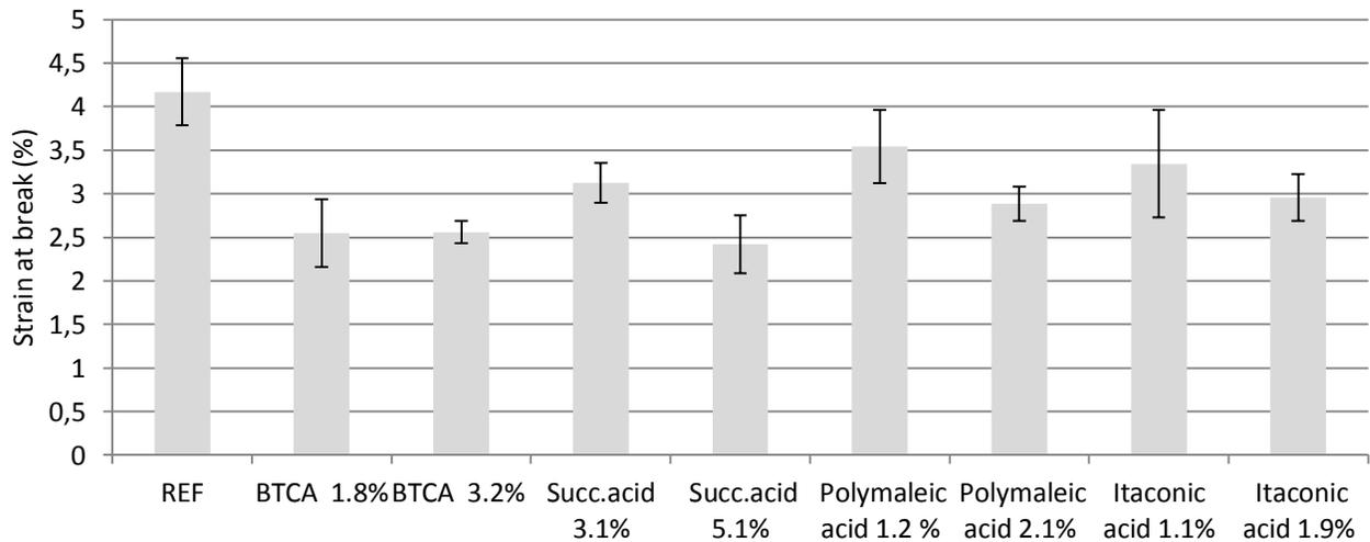
**Figure B1-4.** The influence of acid concentration on the elongation values of test composites hot pressed at 150°C at 31.25 MPa for 15 min, compared to untreated reference samples of all-cellulose composites(n=8) . The error bars are projected at a 95% CI, n=8, for all acid-treated composites.
