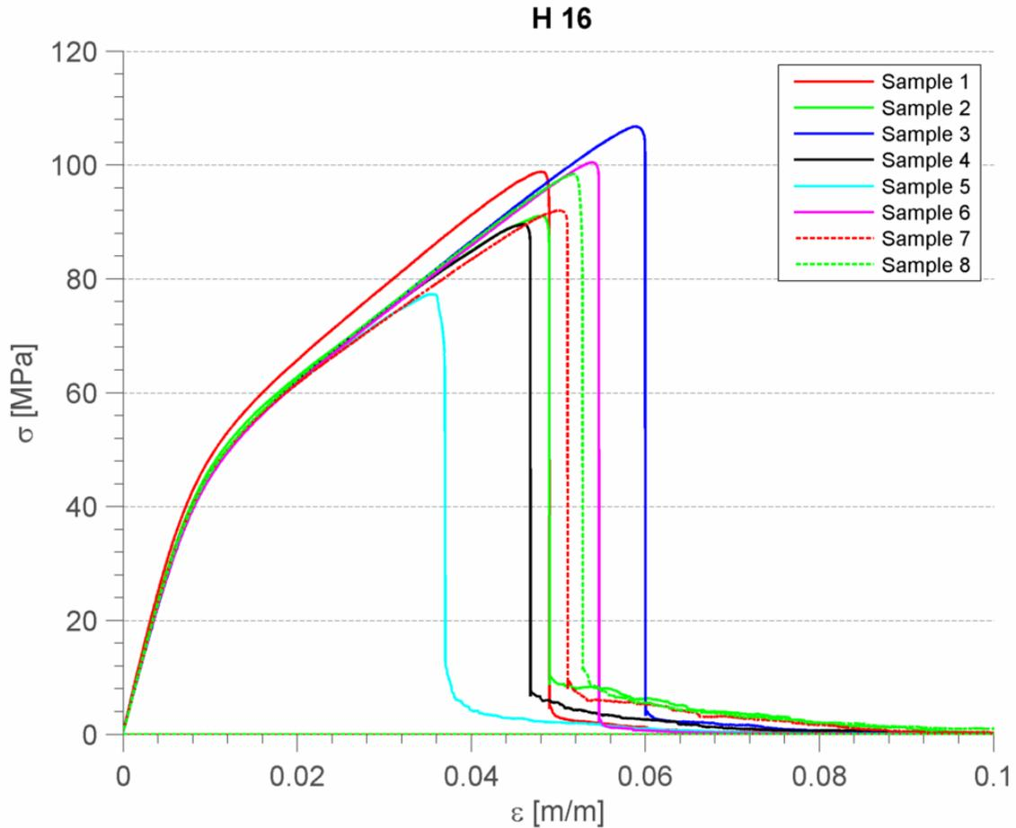
Figure A-1. An example of the plot resulting from the tensile test data converted by Matlab. The data was also exported to an excel file, resulting in table A-1 for the crosslinking additives, and table A-2 for the other polymers.
