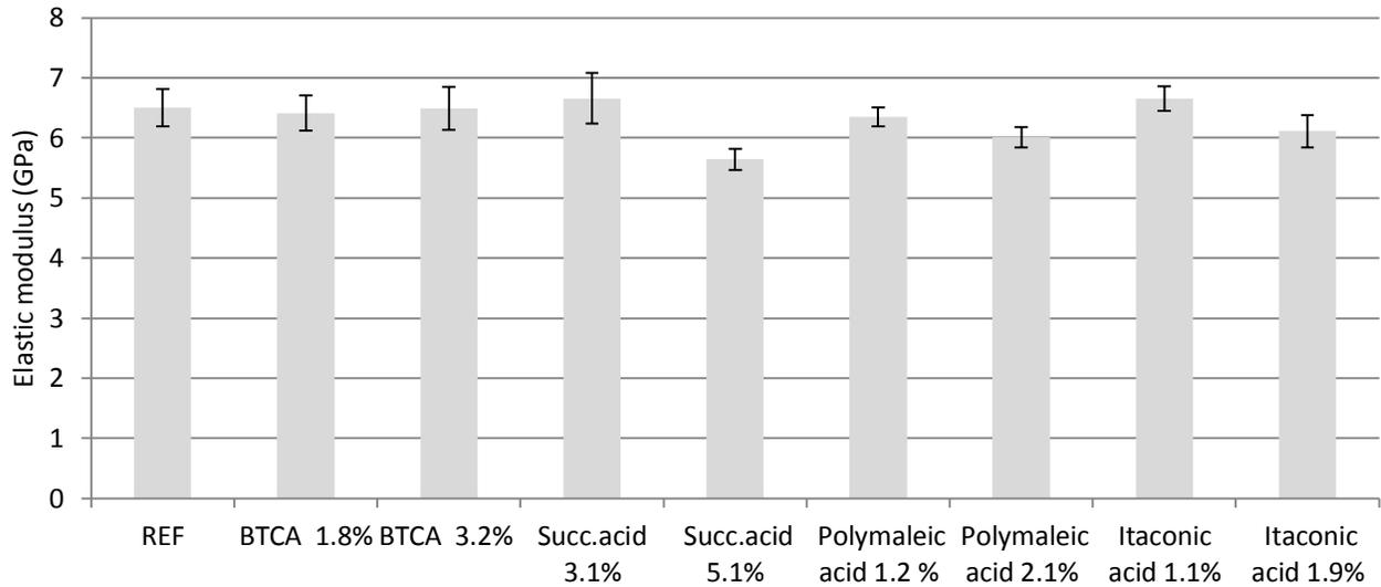
**Figure B1-3.** The influence of acid concentration on the elastic modulus values of test composites hot pressed at 150°C at 31.25 MPa for 15 min, compared to untreated reference samples of all-cellulose composites(n=8) . The error bars are projected at a 95% CI, n=8, for all acid-treated composites.
