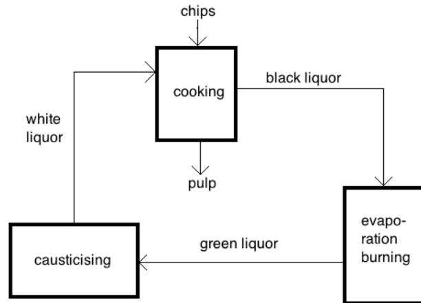
Figure 2-7. A simplified scheme of the liquor cycle in Kraft pulping.
