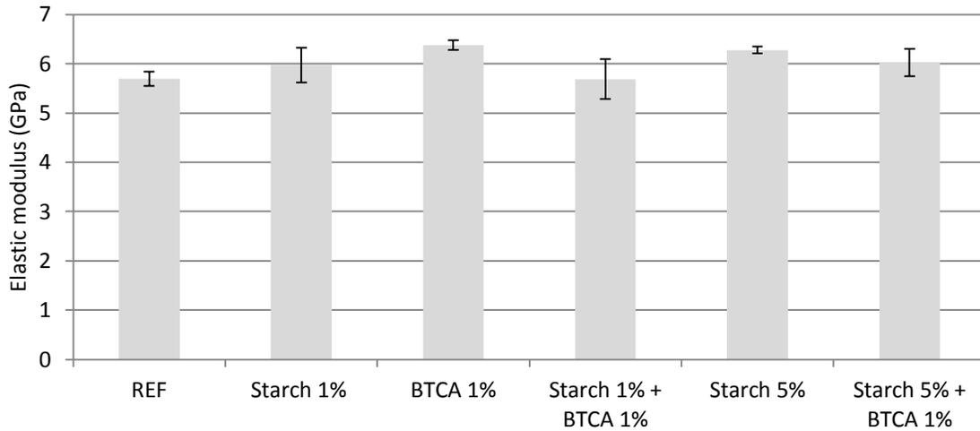
**Figure B2-3.** The elastic modulus (GPa) obtained from the physical modification by starch, combined with the chemical modification of BTCA, compression moulded at 170°C at 31.25 MPa for 15 min, compared to untreated reference samples of all-cellulose composites(n=32) . The error bars are projected at a 95% CI, n=8, for all additive-treated composites.
