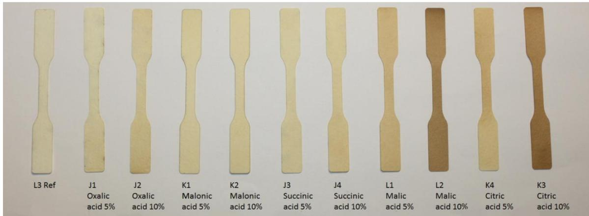
**Figure 4-10.** A picture of the first dog bone samples treated with carboxylic acids. Note that the concentrations here are the aimed concentrations for spraying; the real additive amount is seen in table 4-3.
