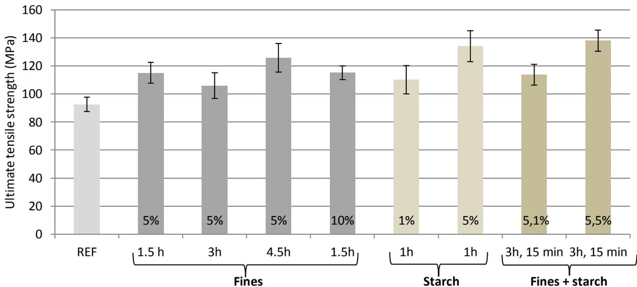
**Figure 4-17.** The ultimate tensile strength (MPa) obtained from the physical modification by starch and fines, compression moulded at 170°C. The error bars are projected at a 95% CI, n=8 apart from the reference sample where n=32.
