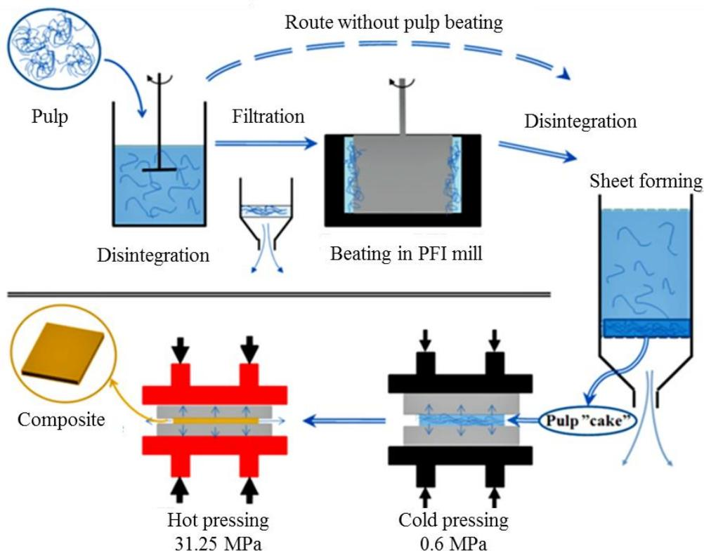
Figure 3-1. Shows a schematic picture of the process route from pulp to composite (Halonen, 2012).
