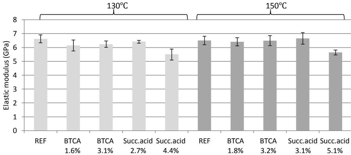
Figure B1-1. The influence of acid concentration on the elastic modulus values of test composites hot pressed at two temperature levels, 130 and 150°C at 31.25 MPa for 15 min, compared to untreated reference samples of all-cellulose composites(n=8). The error bars are projected at a 95% CI, n=8 for all acid-treated composites.
