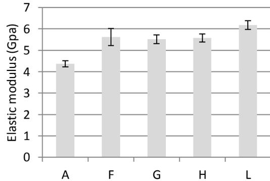
**Figure 4-8.** The module of 200 g/m<sup>2</sup> sheets, compression moulded at 170°C. The error bars are projected at a 95% CI, n=8 apart from for A:n=32.
