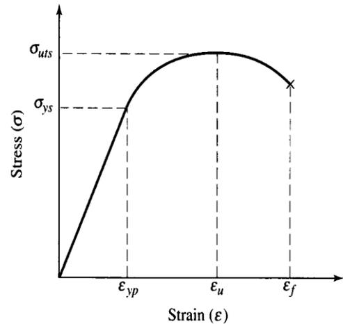
Figure 2-6. The stress-strain curve from a tensile test.
