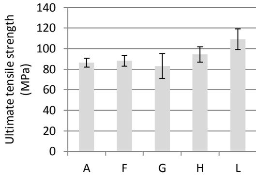
**Figure 4-7.** The ultimate tensile strength of 200 g/m<sup>2</sup> sheets, compression moulded at 170°C. The error bars are projected at a 95% CI, n=8 apart from for A:n=32.
