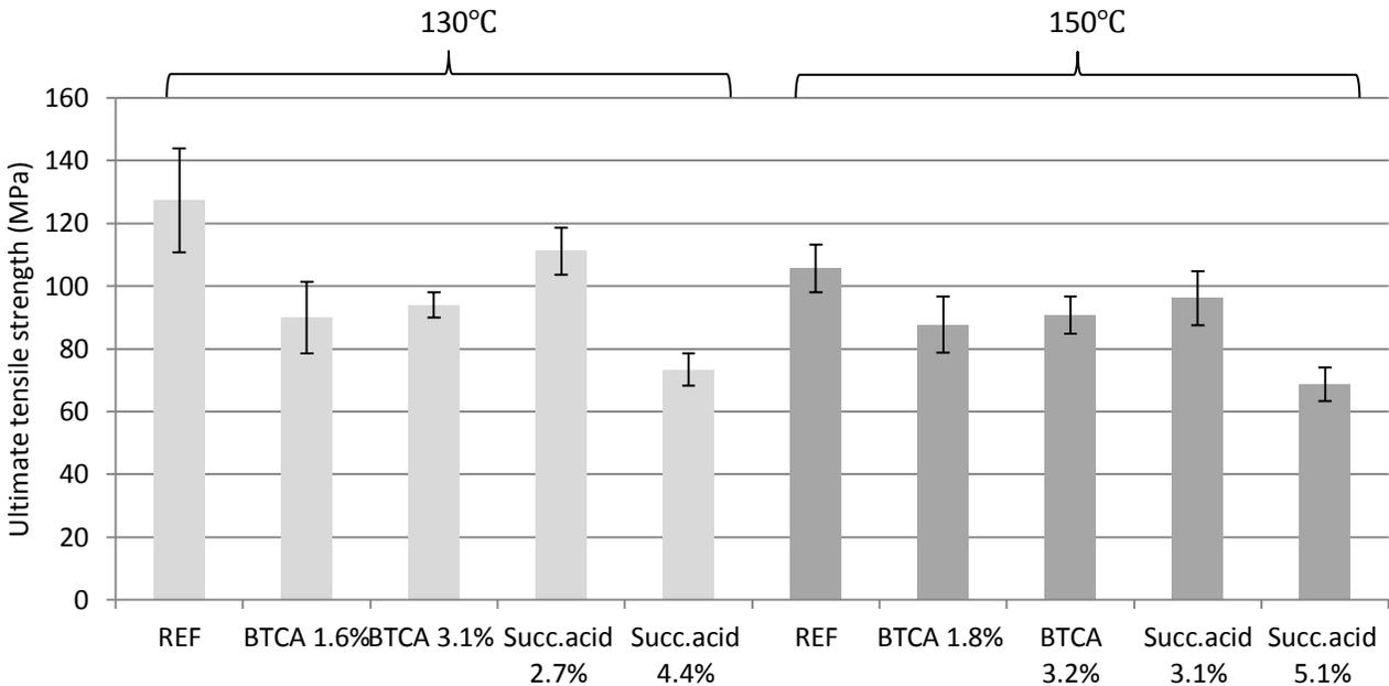
**Figure 4-14.** The influence of acid concentration on the ultimate tensile strength of test composites hot pressed at two temperature levels, 130 and 150°C at 31.25 MPa for 15 min, compared to untreated reference samples of all-cellulose composites (n=8). The error bars are projected at a 95% CI, n=8 for all acid-treated composites.
