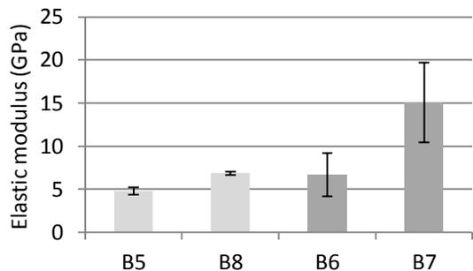
**Figure 4-5.** The module within sheet B, compression moulded at 170°C. The error bars are projected at a 95% CI. B5 and B8 are tensile tested at Innventia, and B6 and B7 at another laboratory, n=8.
