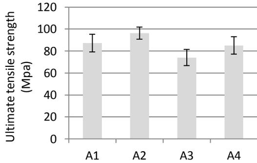
**Figure 4-1.** The ultimate tensile strength (MPa) values within sheet A, compression moulded at 170°C. The error bars are projected at a 95% CI, n=8.
