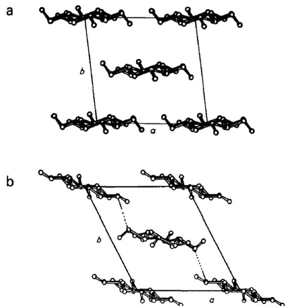
Figure 2-3. The axial projections of the a) native cellulose (cellulose I) and b) regenerated cellulose (cellulose II) (Sjöström, Cellulose 1993 a).
