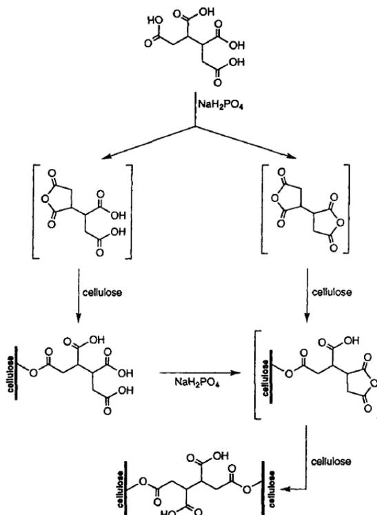
Figure 2-8. The reaction of BTCA during crosslinking with cellulose at 150°C in presence of NaH<sub>2</sub>PO<sub>4</sub>. (ZHOU, P. LUNER, & CALUWE, 1995)
