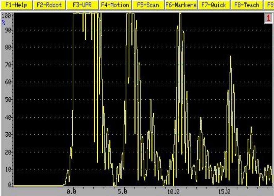
Figure 31: A-scan of the signal generated by probe I7-0512-RG placed over step 1 – the dead zone on about 4 mm.
