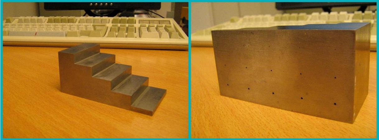
Figure 21: The reference block with flat-bottom holes.
