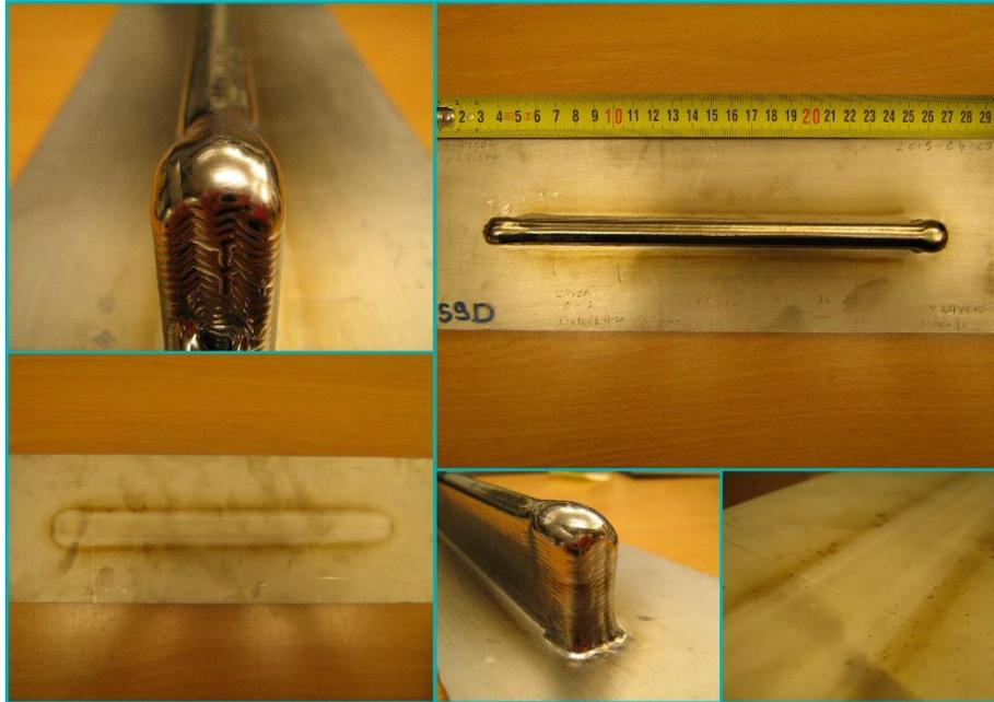
Figure 25: LMD walls in the raw state – rounded top surface (top left), distorted bottom of the piece (bottom left and right).
