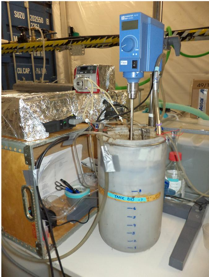
*Figure 7.2 One of the lab scale SBR's successfully installed at Brudaremassen*
