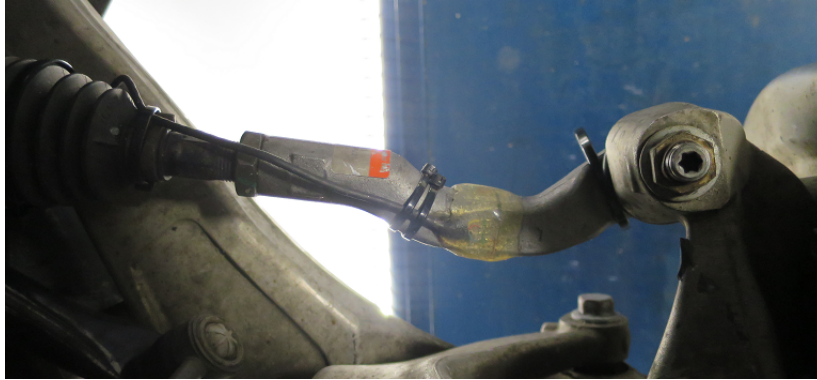
Figure 3.4: Tie-rod with strain gauge sensor mounted
