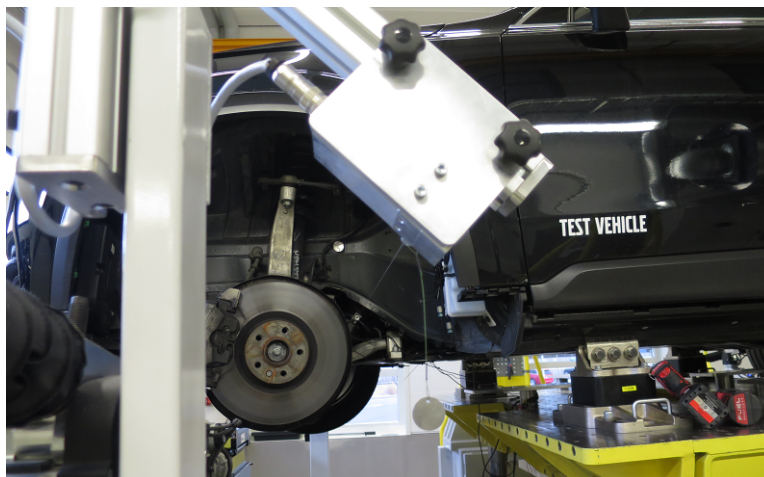
Figure 3.5: Rack travel versus steering wheel angle measurement
