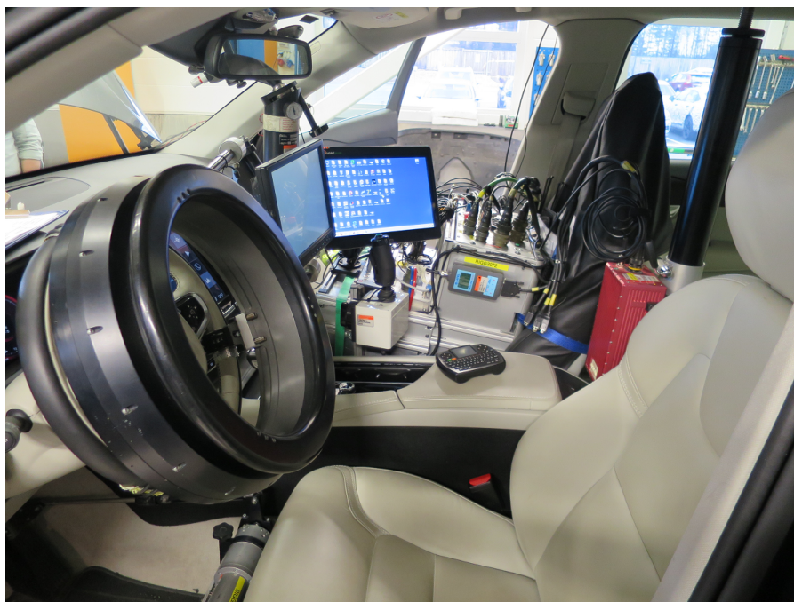
Figure 3.3: Steering robot mounted in the test vehicle
