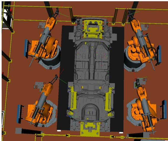
**Figure 1.1:** A snapshot from IPS illustrating four robots in a robot station, a car body (that is the workpiece), and 48 stud weld tasks on the workpiece. A close up of a robot is shown in Figure 1.2a and a close up of a task is shown in Figure 1.2b.
