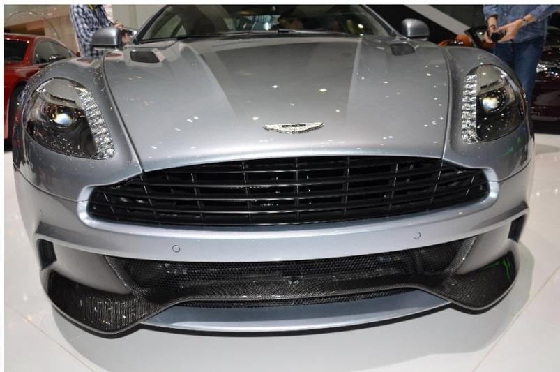
Figure 13. Picture of Aston Martin V12 Vanquish Centenary Edition where the outer bonnet is made of aluminium
