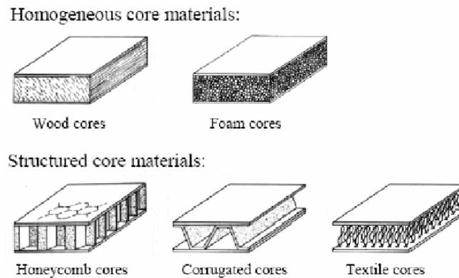
Figure 18. Different sandwich core types [19]
