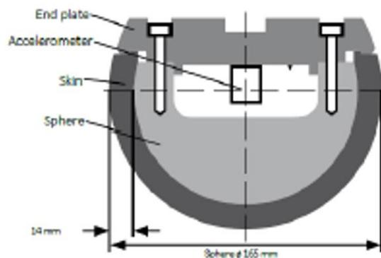
Figure 4. Illustrating the shape of head impact mass
