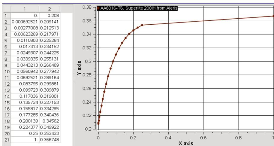
Figure 24. Representing the hardening curve of Aluminium AA6016-T6, Superlite 200IH from Aleris that is used into LS-DYNA
