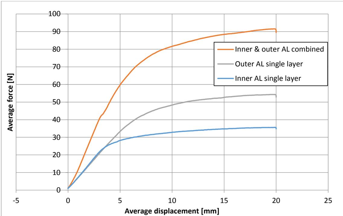
Figure 44. Stiffness results of inner and outer aluminium stiffness samples combined, outer aluminium stiffness sample single and inner aluminium stiffness sample single
