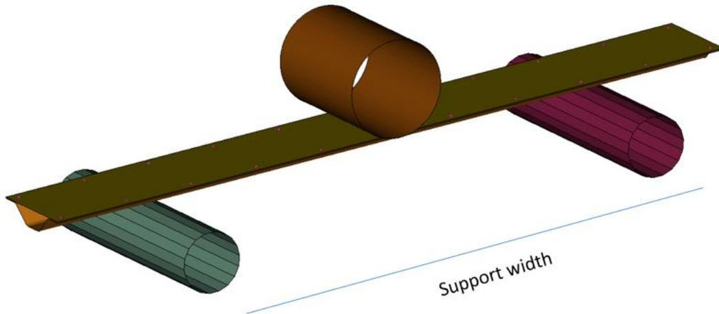
Figure 25. Illustration of the simulation in LS-DYNA. Representing the support widths
