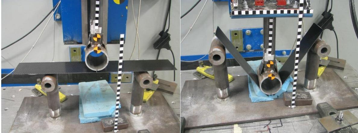
Figure 36. Visualizing before and after impact of CFRP/PVC foam sandwich material
