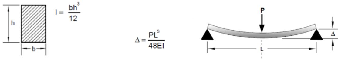
Figure 42. Shape factor and simply supported beam centre load of current design.  $\Delta$ ,  $E$ ,  $P$ ,  $L$  and  $I$  describes deflection, flexural modulus, force (load), Length of beam and moment of inertia of bending axis respectively.
