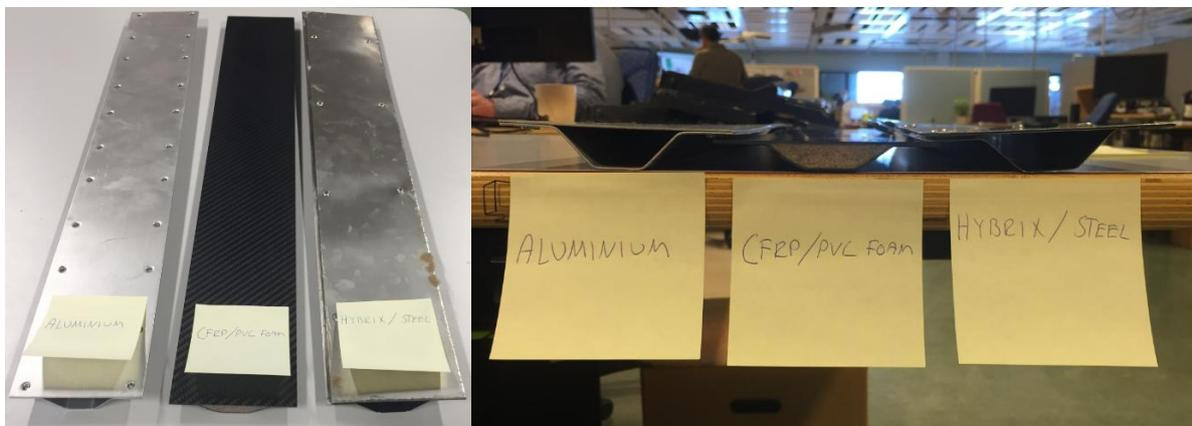
Figure 31. Visualizing the different beams made of aluminium, CFRP/PVC foam sandwich and Hybrix/steel.
