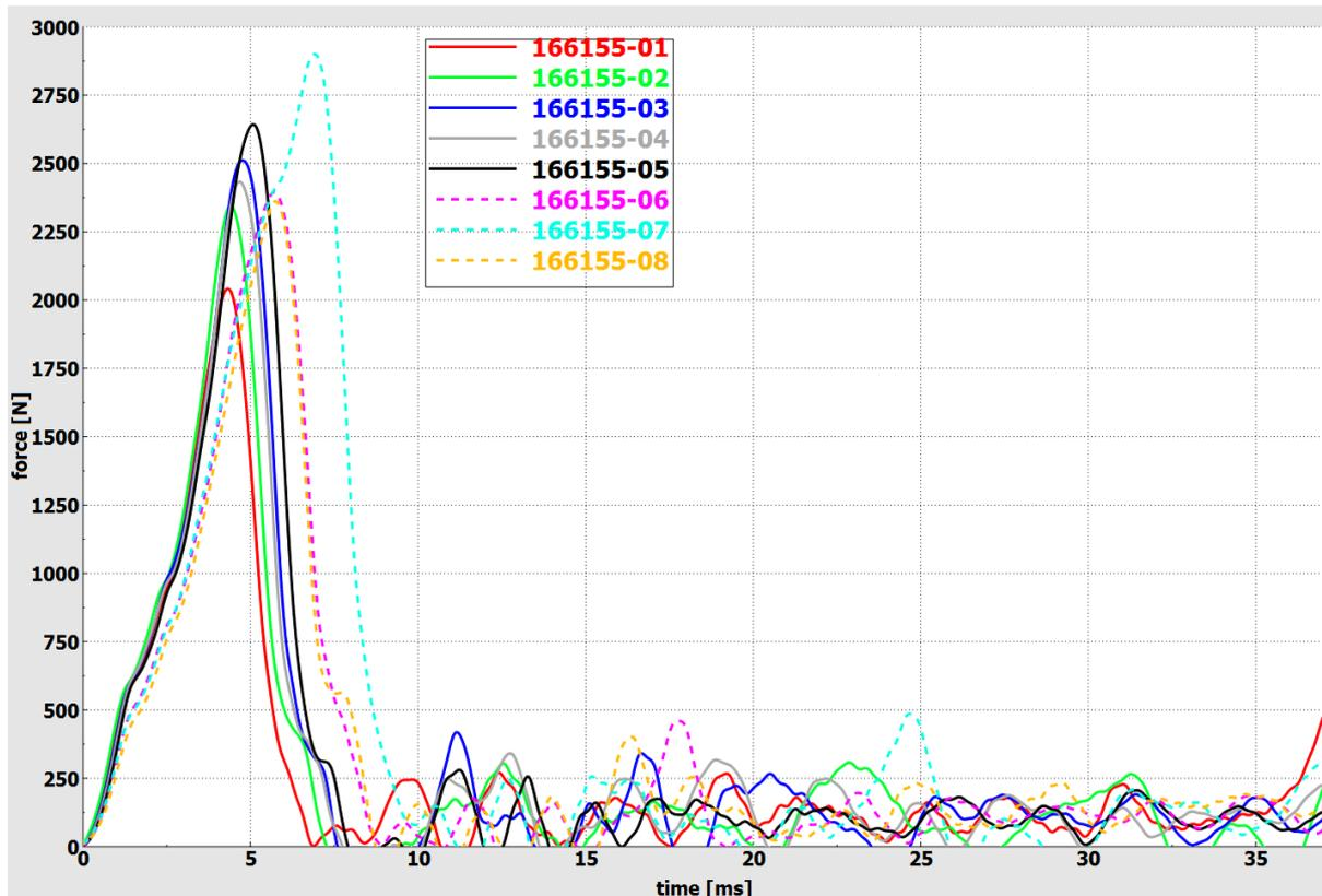
Figure 37. Force distribution for CFRP/PVC foam sandwich beams
