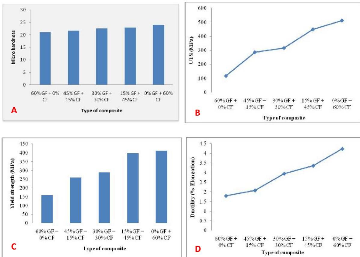
Figure 17. Changing in mechanical properties by replacing the glass fiber with carbon fiber. A is micro hardness, B is UTS, C is yield strength, D is ductility [16]
