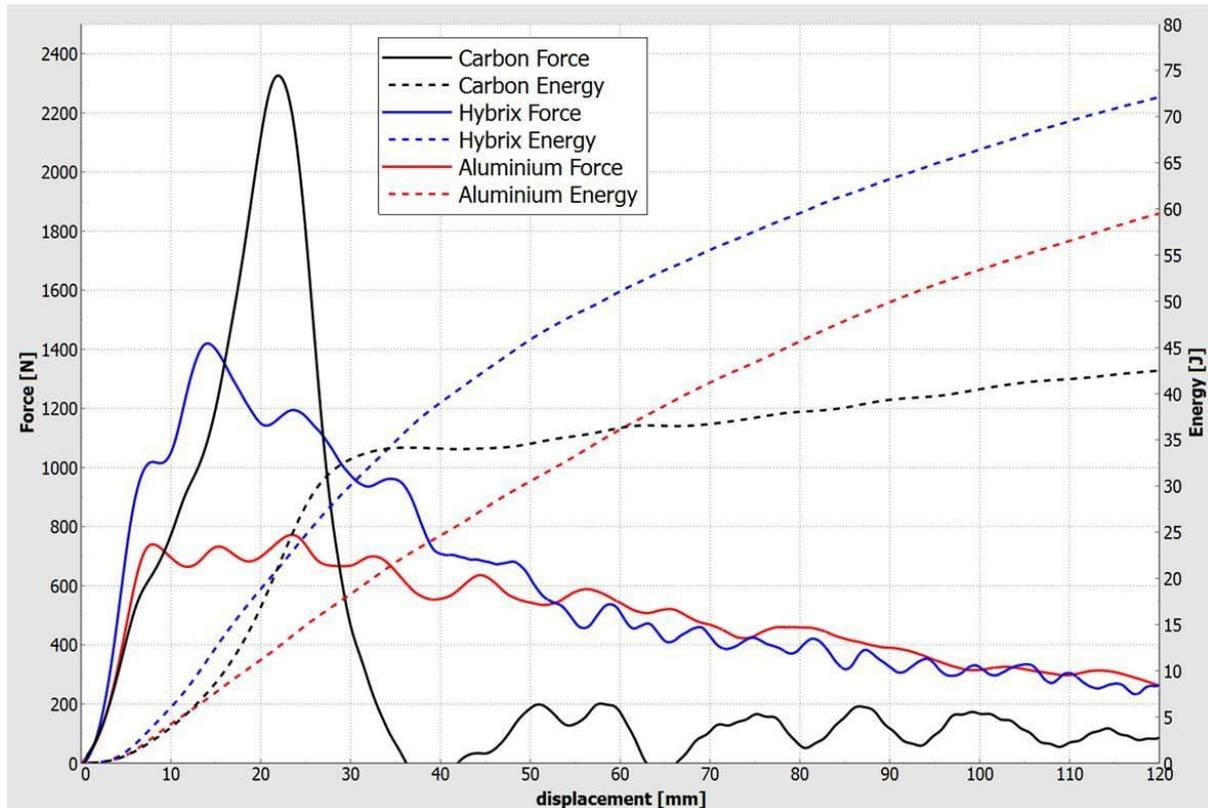
Figure 41. Force/displacement/Energy curves for the different materials
