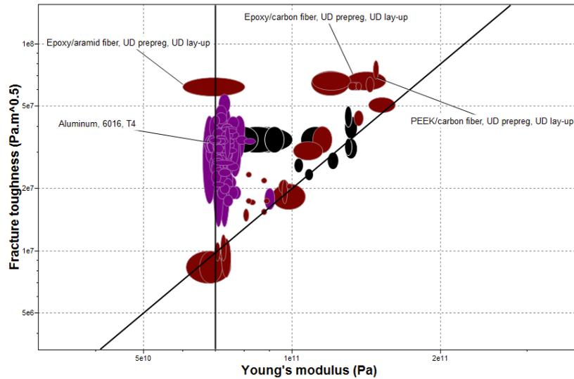
Figure 20. Fracture toughness vs. Young modulus
