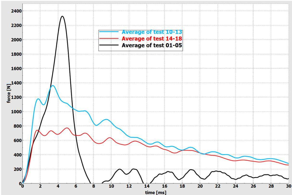
Figure 40. Comparison of the different materials subjected to the impact test. Each curve is an average of each material series in the testing. Black line is CFRP/PVC foam sandwich material, Blue line is Hybrix/Steel and Red line is the aluminium material
