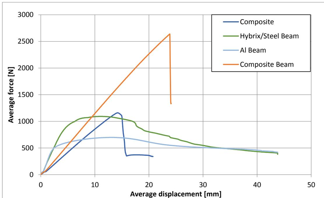
Figure 43. Stiffness result of CFRP/PVC sandwich material, Hybrix/Steel beam, Aluminium beam and CFRP/PVC foam sandwich rectangular samples
