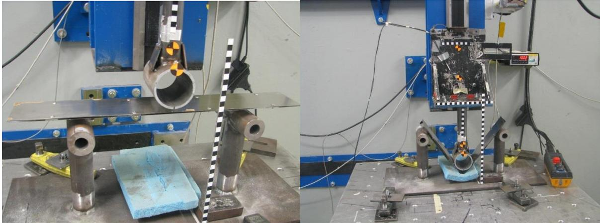
Figure 38. Visualizing before and after impact of Hybrix/steel beam
