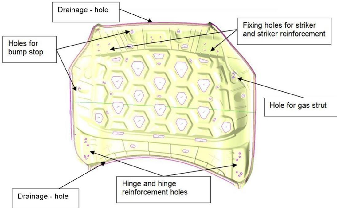
Figure 1. Inner bonnet structure of V526
