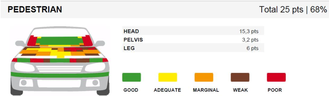
Figure 11. Pedestrian safety results from EuroNCAP Renault Twingo [28]
