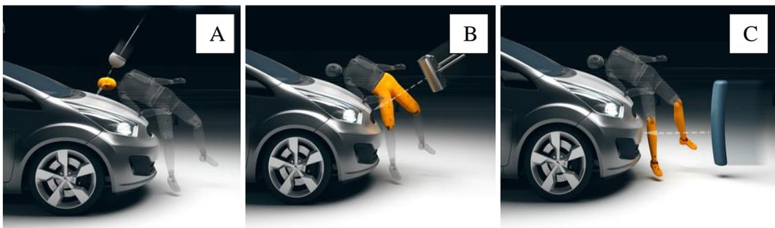
Figure 3. Crash impact testing of Car Bonnet at 40 km/h, A is head impact, B is leg impact and C is lower leg impact testing
