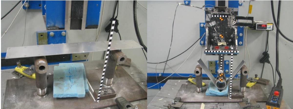
Figure 34. Before and after picture of one aluminium beam subjected to an impact velocity of 4 m/s
