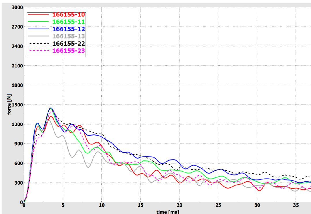
Figure 39. Force distribution of the Hybrix beam
