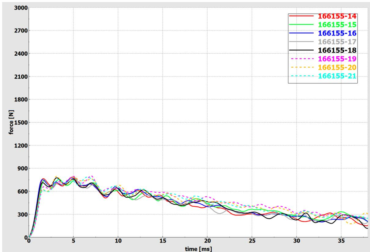
Figure 35. Force variation of aluminium beams
