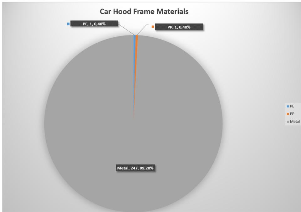
Figure 9. Results of materials used in bonnets
