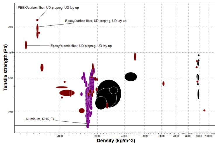
Figure 21. Tensile Strength vs. Density
