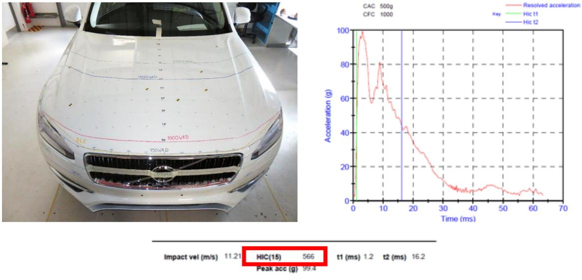
Figure 6. Crash impact testing of Volvo XC90
