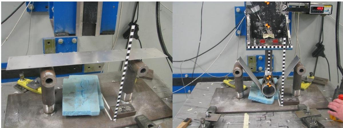
Figure 33. Before and after picture of one aluminium beam subjected to an impact velocity of 5 m/s
