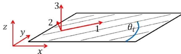
Figure 16. Illustration of relationship of material orientation and coordinate system
