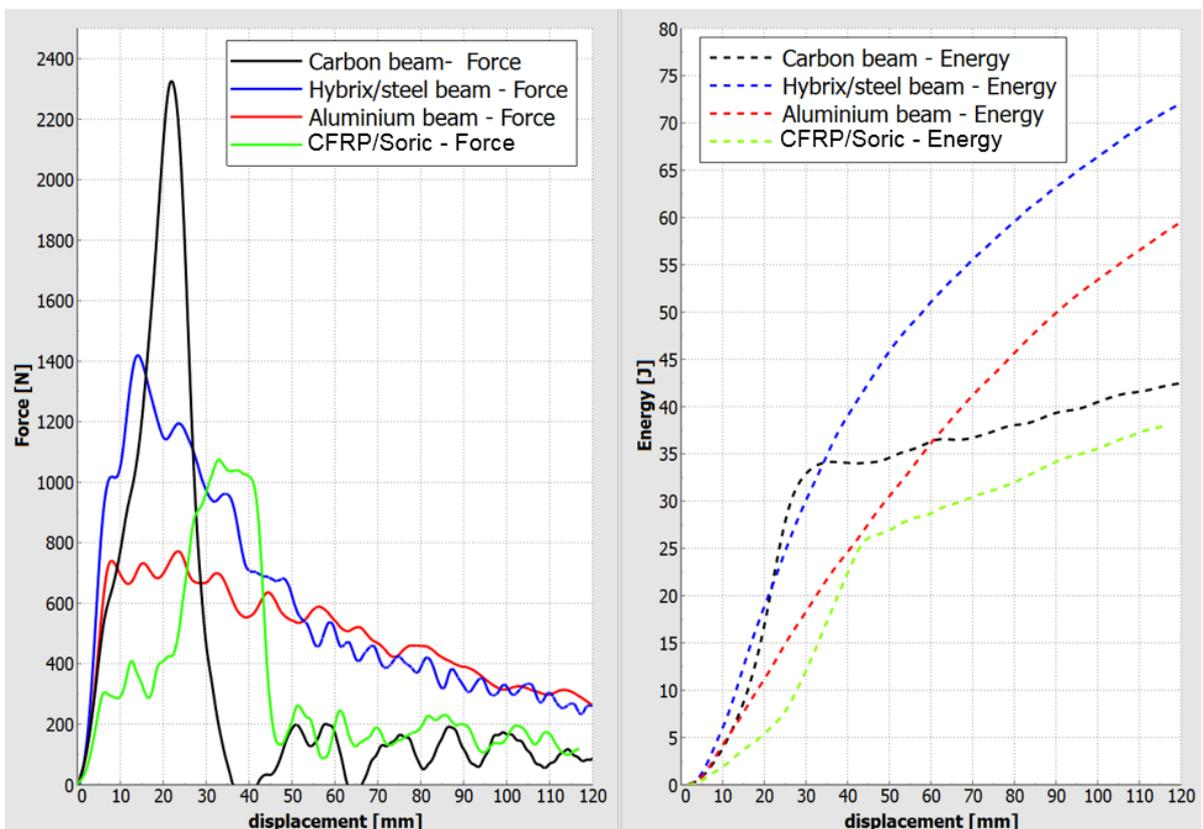
Figure 46. Energy curves of all materials including CFRP/Soric
