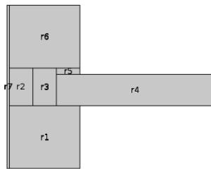
With the same reasoning as above, thermal resistance from any interior surface layer has been neglected. The cavity between the slab and the wall, denoted as “ $r3$ ” and “ $r5$ ” in the figure above has different dimensions depending on the width of the wall, see table below.
