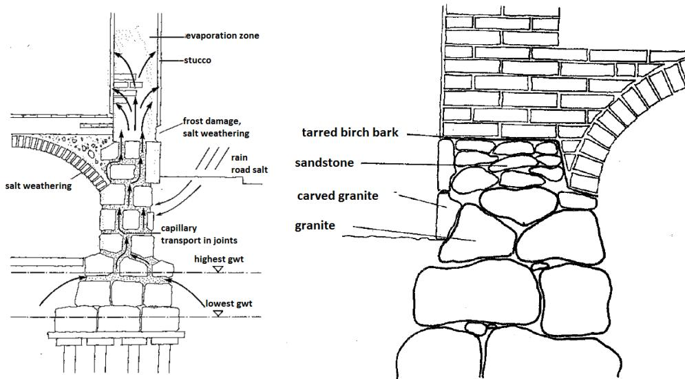
*Figure 3.4 Left: Section through foundation wall transitioning to façade wall, capillary suction transport (Humble, 1990). Right: Section through foundation wall transitioning to façade wall (Eriksson and Hansson, 1974).*
