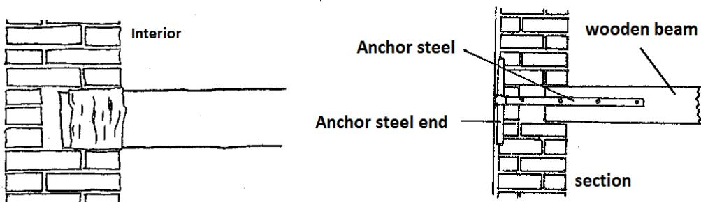
*Figure 3.6 Left: Basic example of beam box, covered with birch bark or bituminous paper (Eriksson and Hansson, 1974). Right: Basic example of beam box, with anchor steel (Eriksson and Hansson, 1974).*
