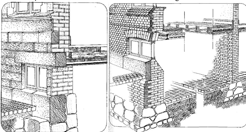
Figure 3.1 Examples of structural composition of two foundation walls (Björk et al., 2013).
