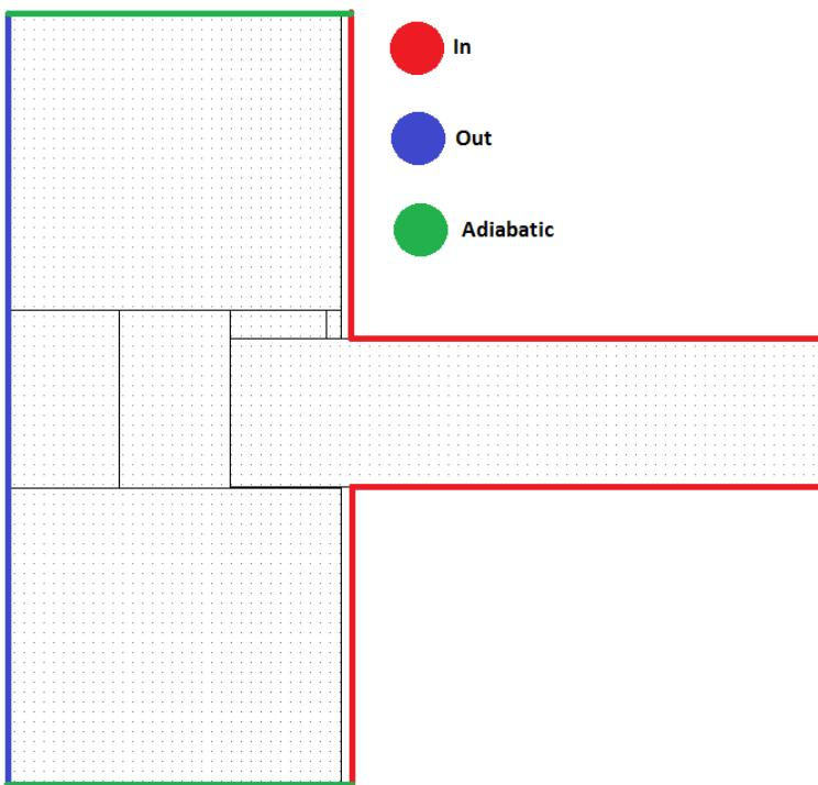
Figure 4, Basic geometry with boundary conditions
