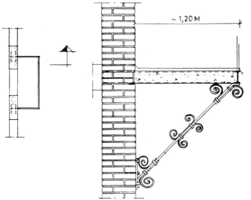
Figure 3.9 Balcony construction (Bjerking, 1974).
