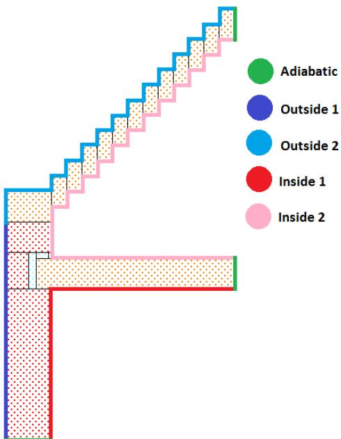
Figure 4, basic geometry with boundary conditions
