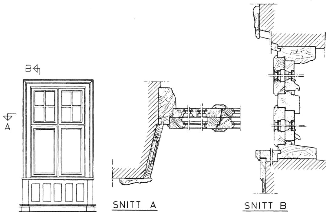
Figure 3.8 Window construction until 1910-1930 (Bjerking, 1974).
