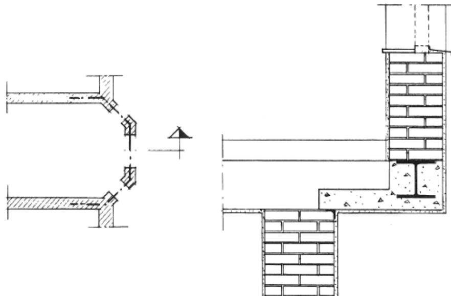
Figure 3.10 Bay window construction (Bjerking, 1974).
