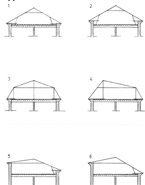
*Figure 3.2 Typical designs of roof trusses for cold attics (Bjerking, 1974).*
