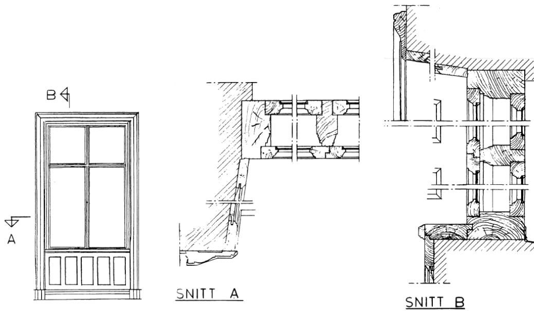
Figure 3.7 Window construction until 1920 (Bjerking, 1974).
