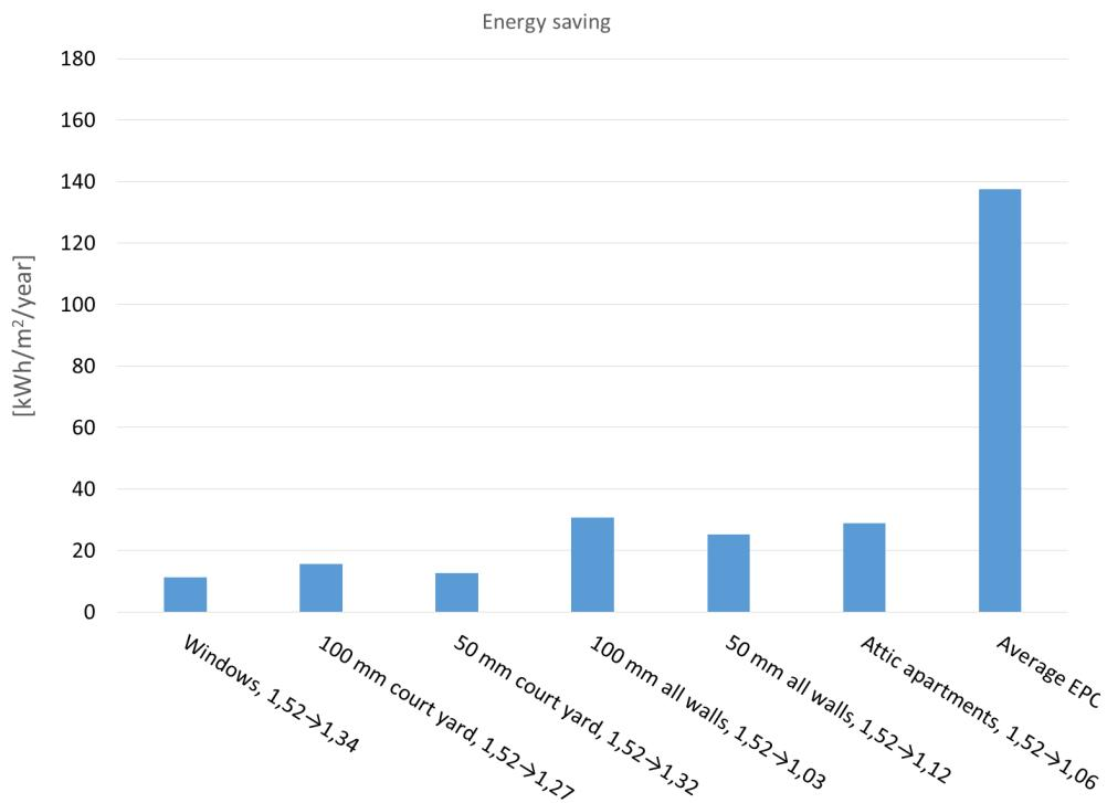
Figure 7.2 Diagram with energy savings due to U-value reduction from renovations and average EPC.
