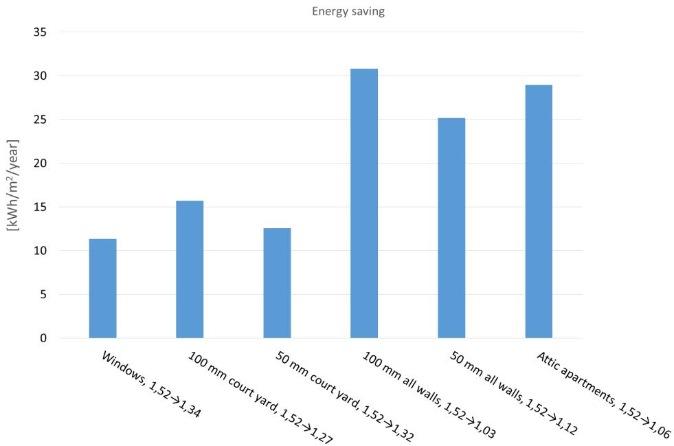
Figure 7.1 Diagram with energy savings due to U-value reduction from renovations.
