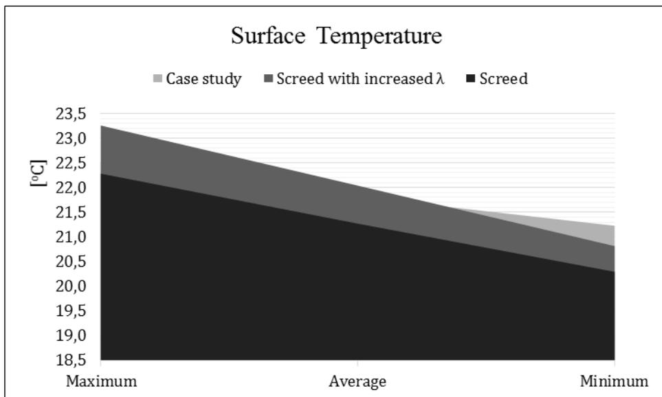
Figure 6.9 Surface temperature of increased thermal mass in floor construction
