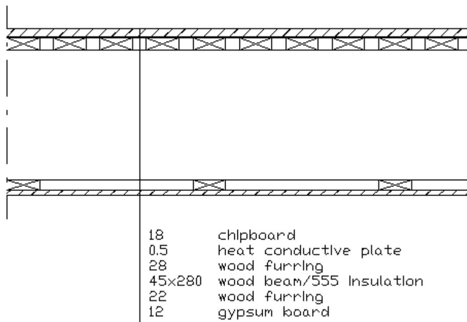
Figure 4.2 Geometry and material of floor construction in Standard room
