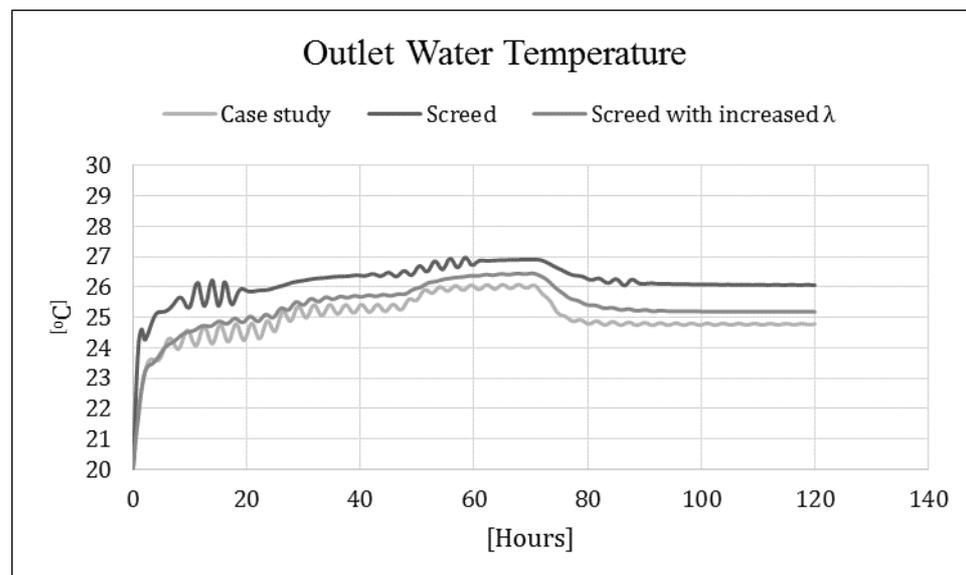
Figure 6.12 Outlet water temperature when simulating transient with increased thermal mass in floor construction
