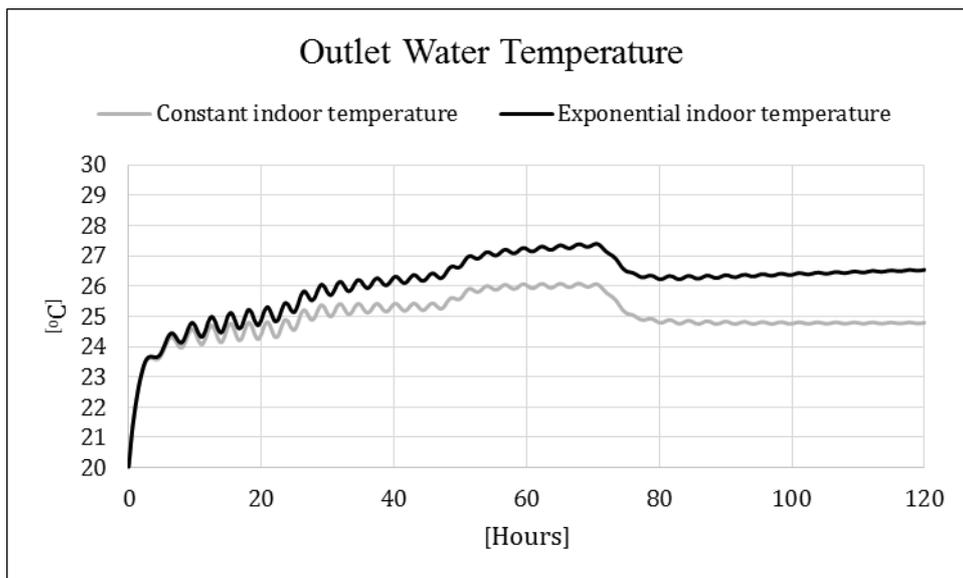
Figure 5.11 Outlet water temperature of transient analysis with positive disturbance
