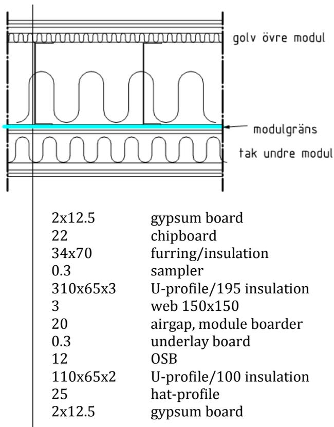
Figure 5.3 Floor construction in HSB Living Lab
