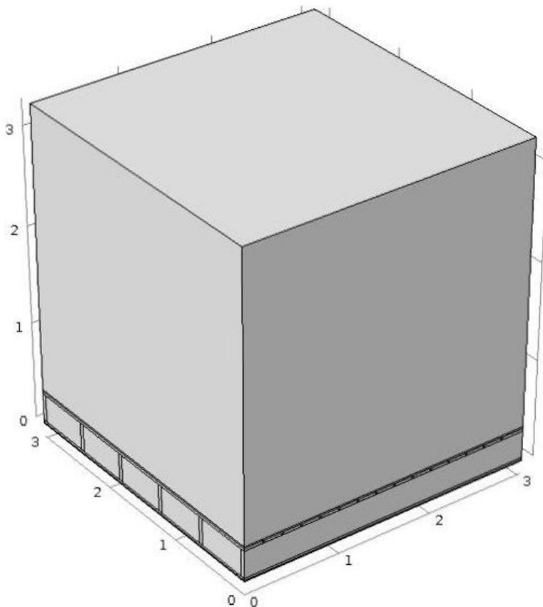
Figure 4.7 COMSOL Multiphysics model representing floor construction with embedded floor heating system and added air box
