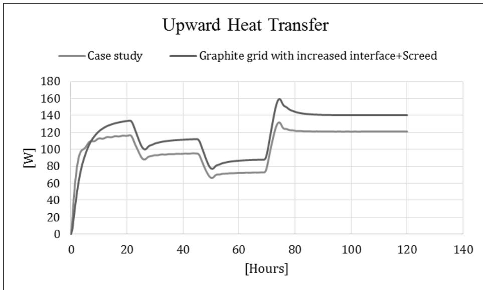
Figure 6.16 Upward heat transfer when simulating transient with combined solution
