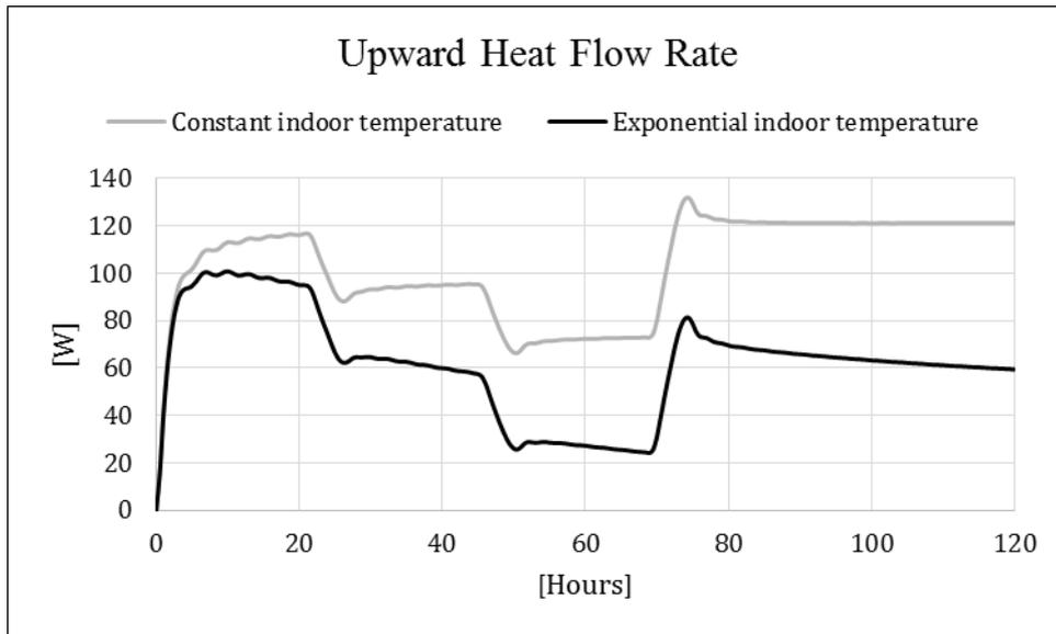
Figure 5.10 Heat transfer upward of transient analysis with positive disturbance
