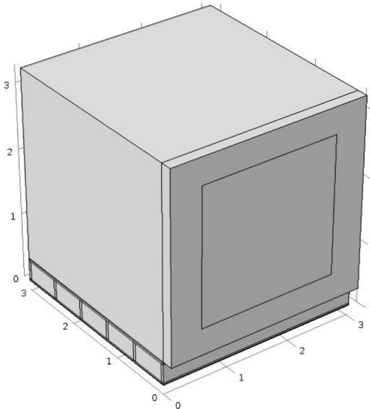
Figure 4.8 COMSOL Multiphysics model representing floor construction with embedded floor heating system and added air box and external wall
