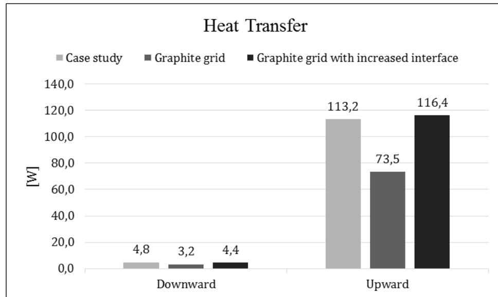
Figure 6.2 Upward and downward heat transfer with increased heat distribution
