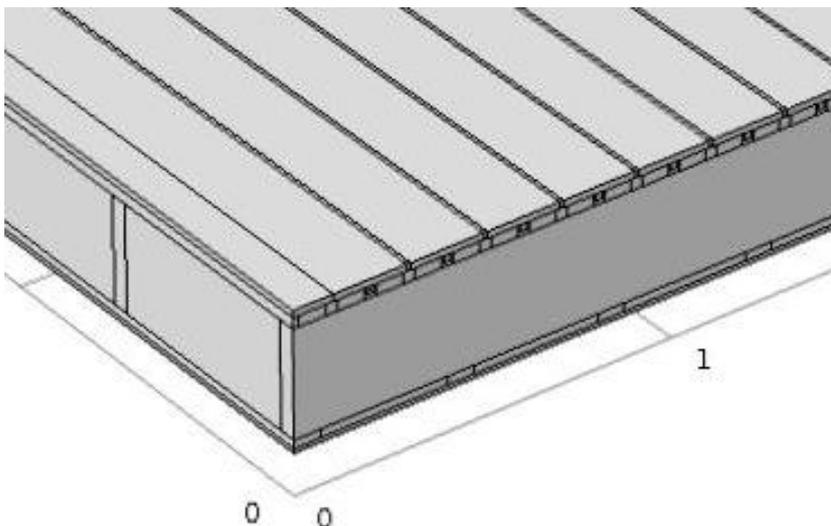
Figure 4.9 Non-homogenous model of Standard room in COMSOL Multiphysics 5.2
