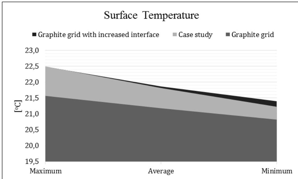
Figure 6.3 Surface temperature with increased heat distribution
