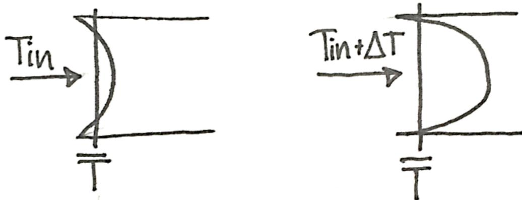
Figure 4.5 Temperature distribution within the cross section of the pipe inlet
