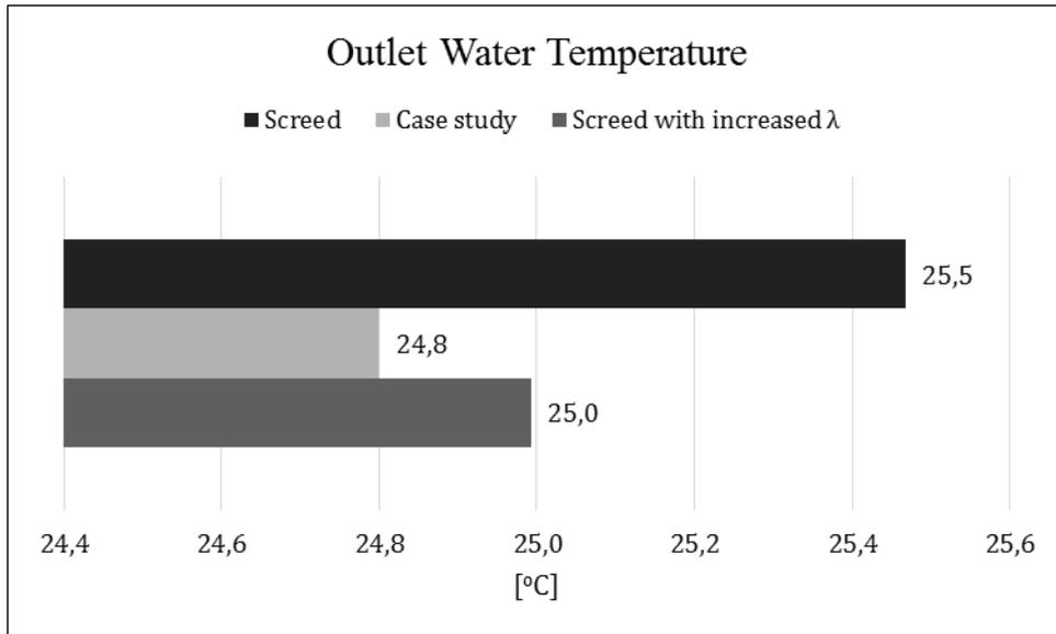
Figure 6.10 Outlet water temperature with increased thermal mass of floor construction
