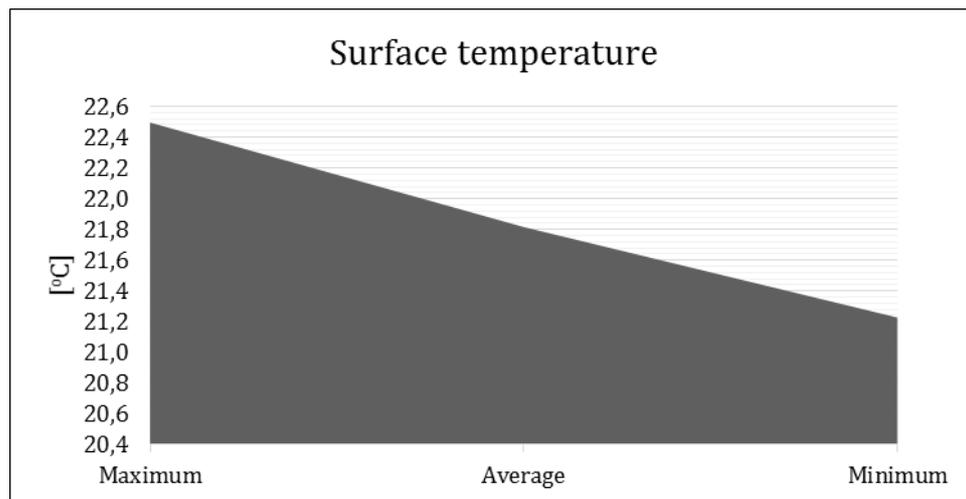
Figure 5.9 Floor surface temperature of case study model when simulated stationary
