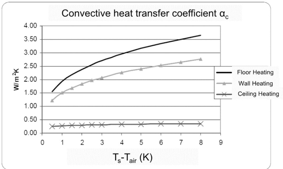
Figure 3.2 Convective heat transfer coefficient between floor surface and ambient air when using a building integrated heating system.
