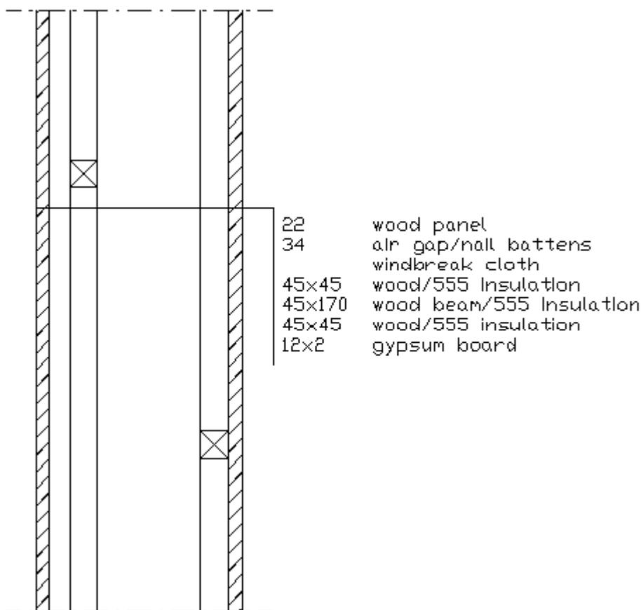
Figure A.1 Geometry and materials of external wall in standard room
