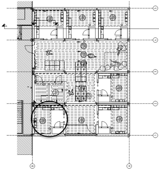
Figure 5.2 Floor heating system in one side of floor two and four in HSB Living Lab
