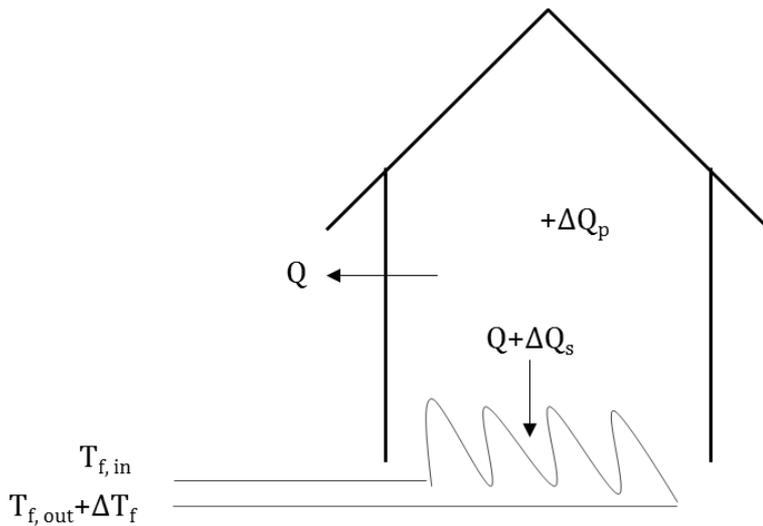
Figure 3.5 Function of self-regulation ability of floor heating systems
