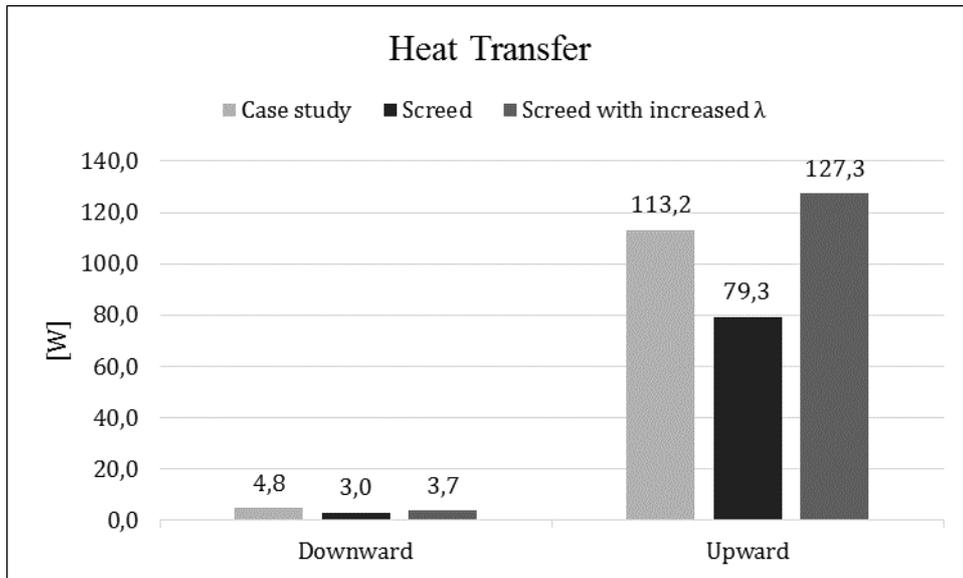
Figure 6.8 Upward and downward heat transfer of increased thermal mass in floor construction
