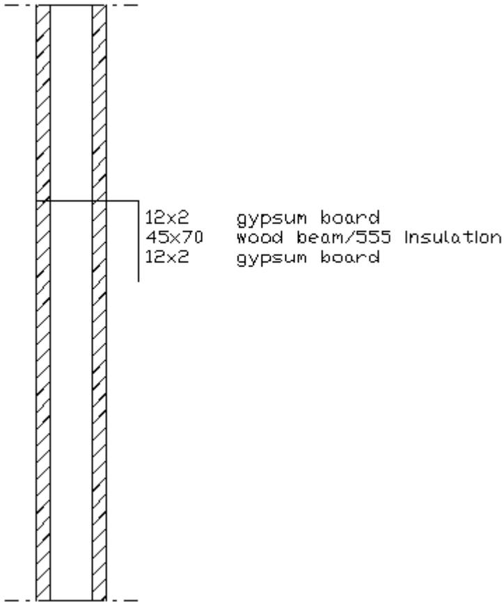
Figure A.2 Geometry and material of internal wall in standard room
