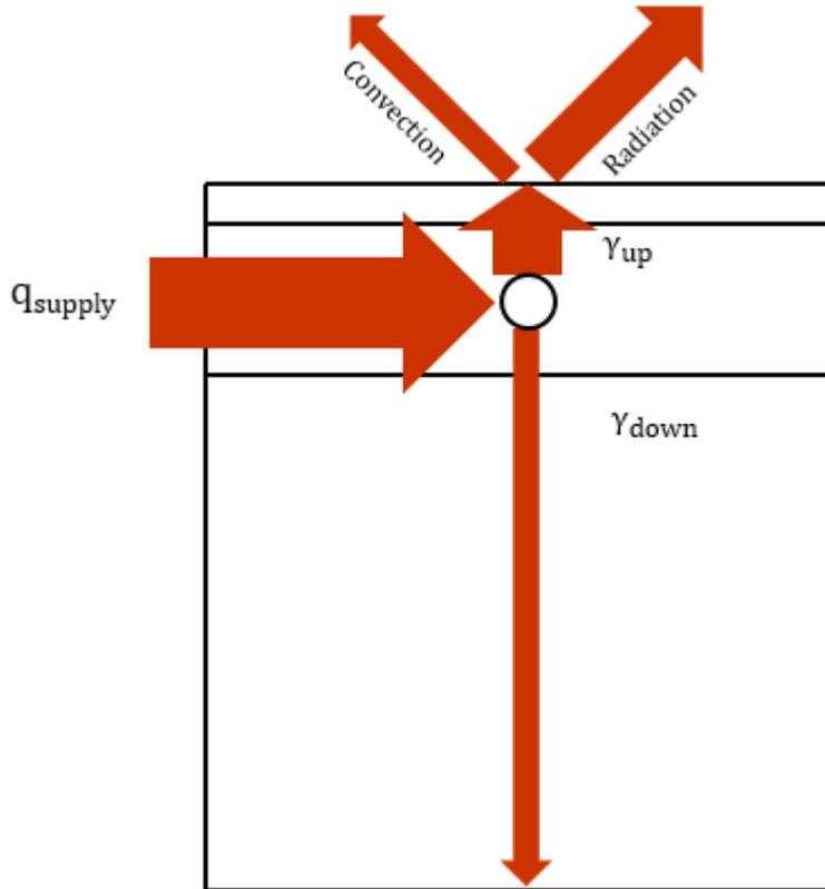
Figure 3.4 Heat transfer mechanisms of a floor heating system
