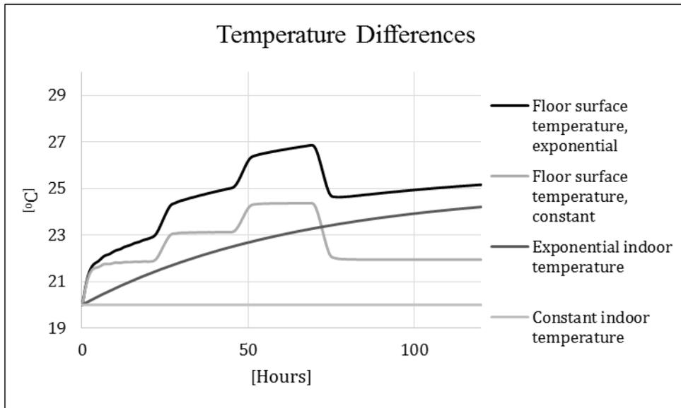
Figure 5.12 Temperature differences between floor surface and indoor temperature of transient analysis with positive disturbance
