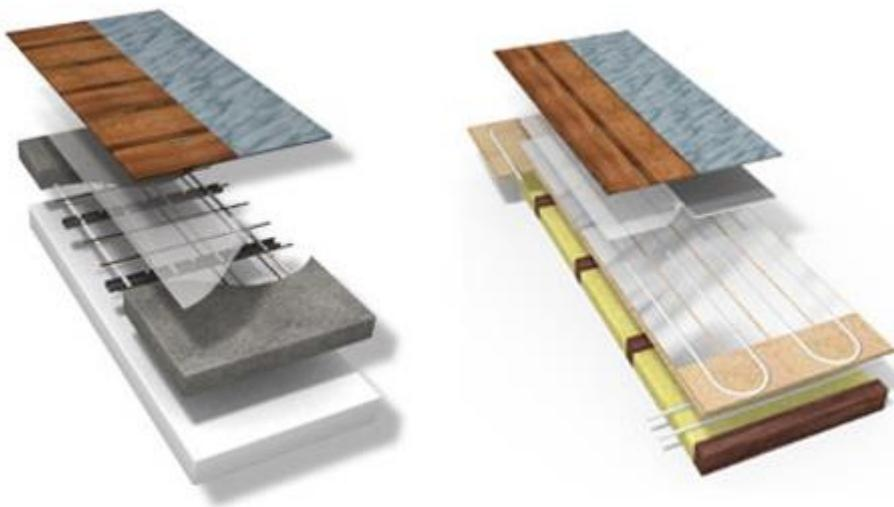
Figure 3.1 Floor heating system installed in heavy-weight floor construction, left picture, and light-weight floor construction, right picture. [Electronic image]
