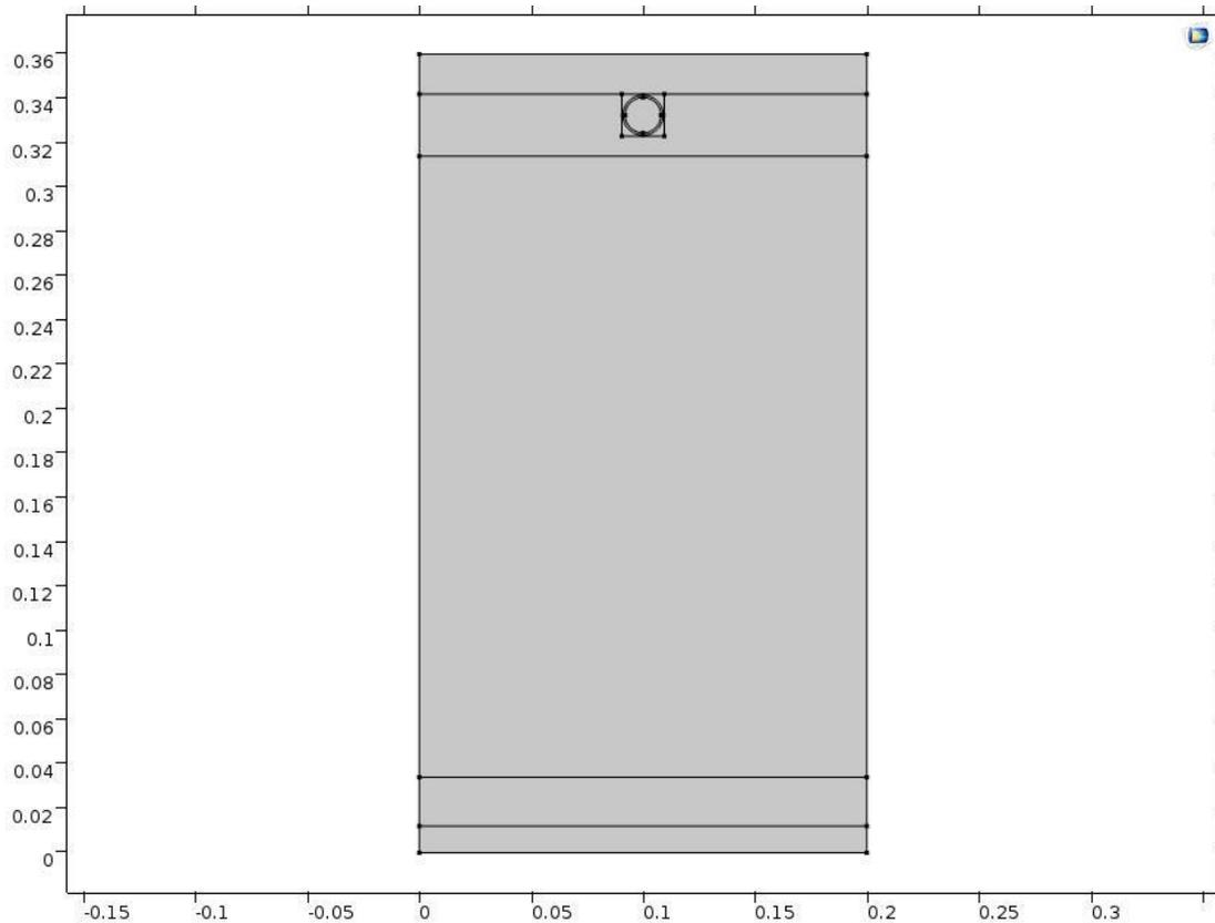
Figure B.1 2D model of the cc-distance of the pipes in the standard room
