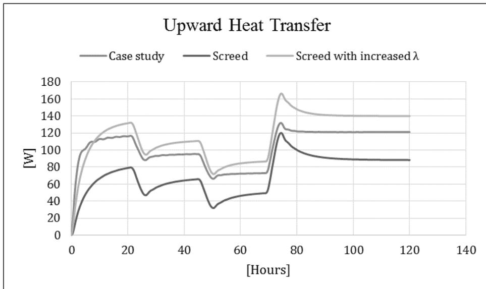
Figure 6.11 Upward heat transfer when simulating transient with increased thermal mass in floor construction
