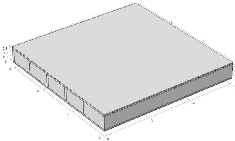
Figure 4.6 COMSOL Multiphysics model representing floor construction with embedded floor heating system
