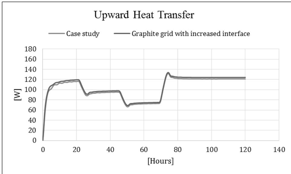
Figure 6.5 Upward heat transfer when simulating transient with increased heat distribution
