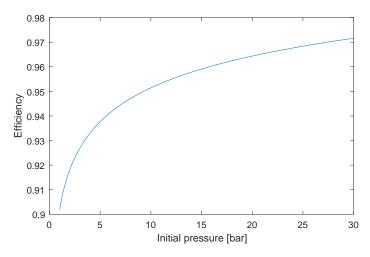
Figure 4.4: Efficiency dependence on initial compression pressure
