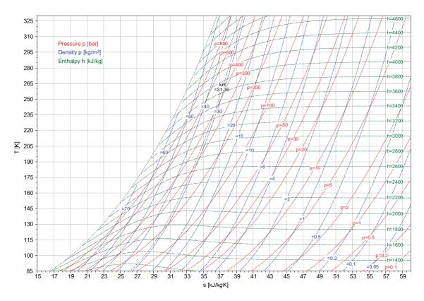
Figure 4.3: T-s diagram for equilibrium hydrogen[76]
