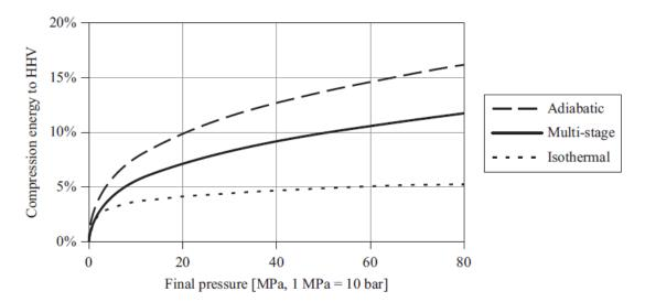
Figure 3.4: Hydrogen compression requirements[59]
