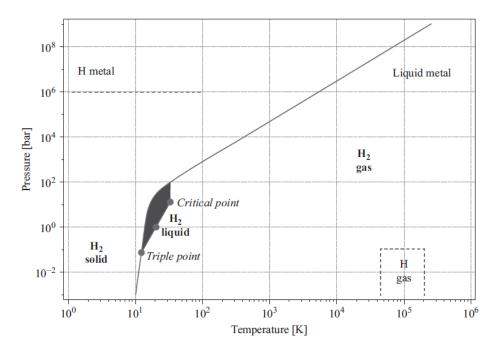
Figure 3.3: Hydrogen phase diagram
