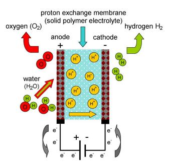
Figure 2.4: PEM electrolyzer layout [46]
