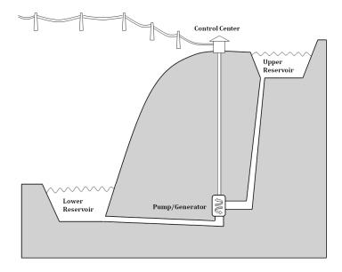
Figure 2.2: Pumped hydroelectric storage plant layout [35]
