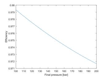
Figure 4.5: Efficiency dependence on maximum pressure
