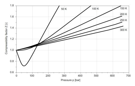
Figure 3.2: Compressibility factor of Hydrogen
