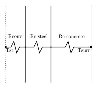
Figure 3.5: Lumped parameter representation
