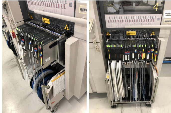
Figure 14 - Material carrier plugged into a SMT line
