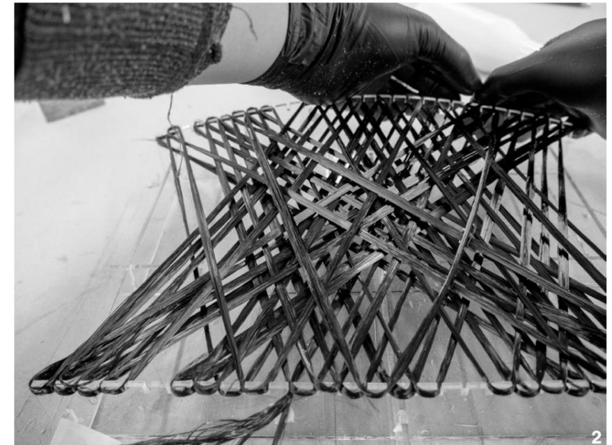
Figure 23. Carbon fiber weaving, Stop Motion Photo 4. Author's own copyright.
