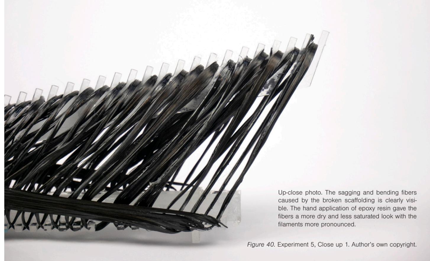
Up-close photo. The sagging and bending fibers caused by the broken scaffolding is clearly visible. The hand application of epoxy resin gave the fibers a more dry and less saturated look with the filaments more pronounced.
