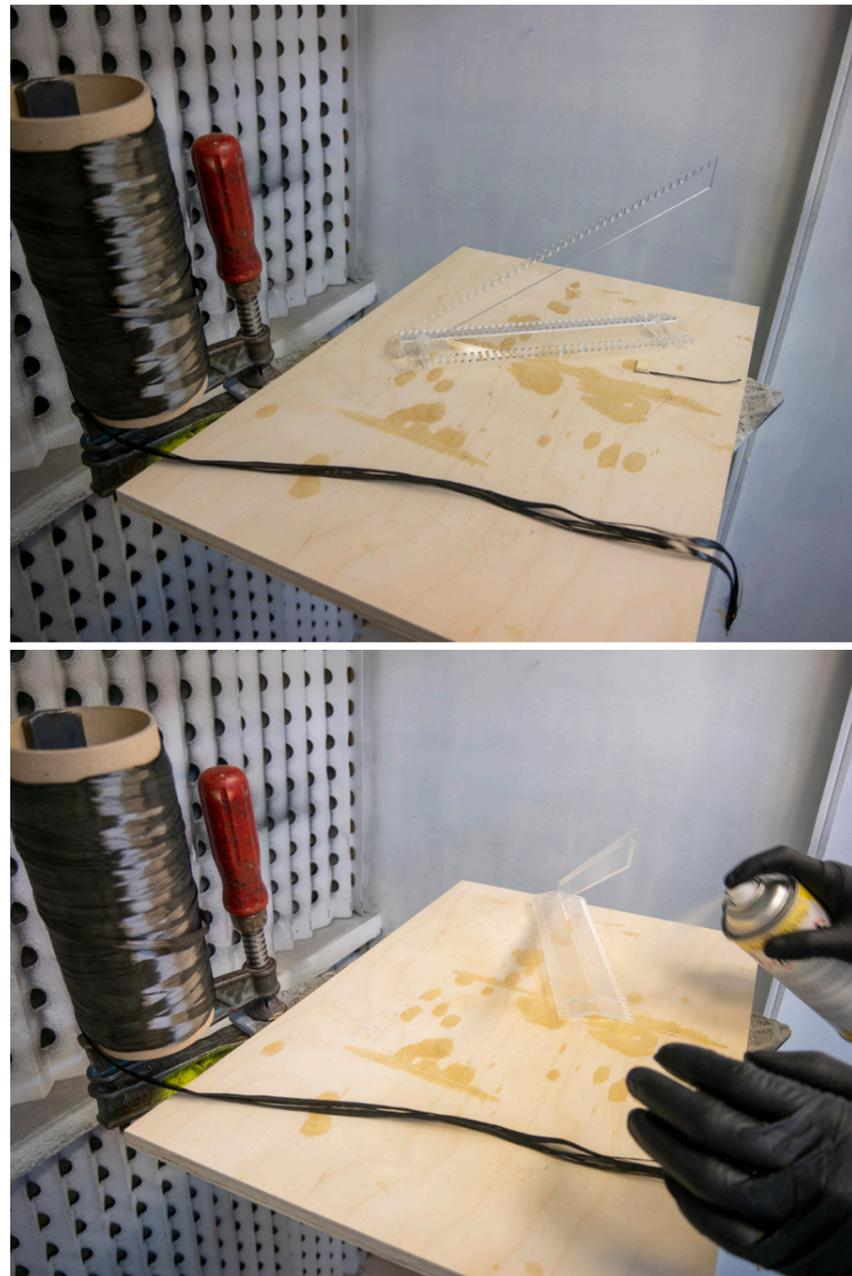
Figure 37. Experiment 5, applying release agent. Author's own copyright.
