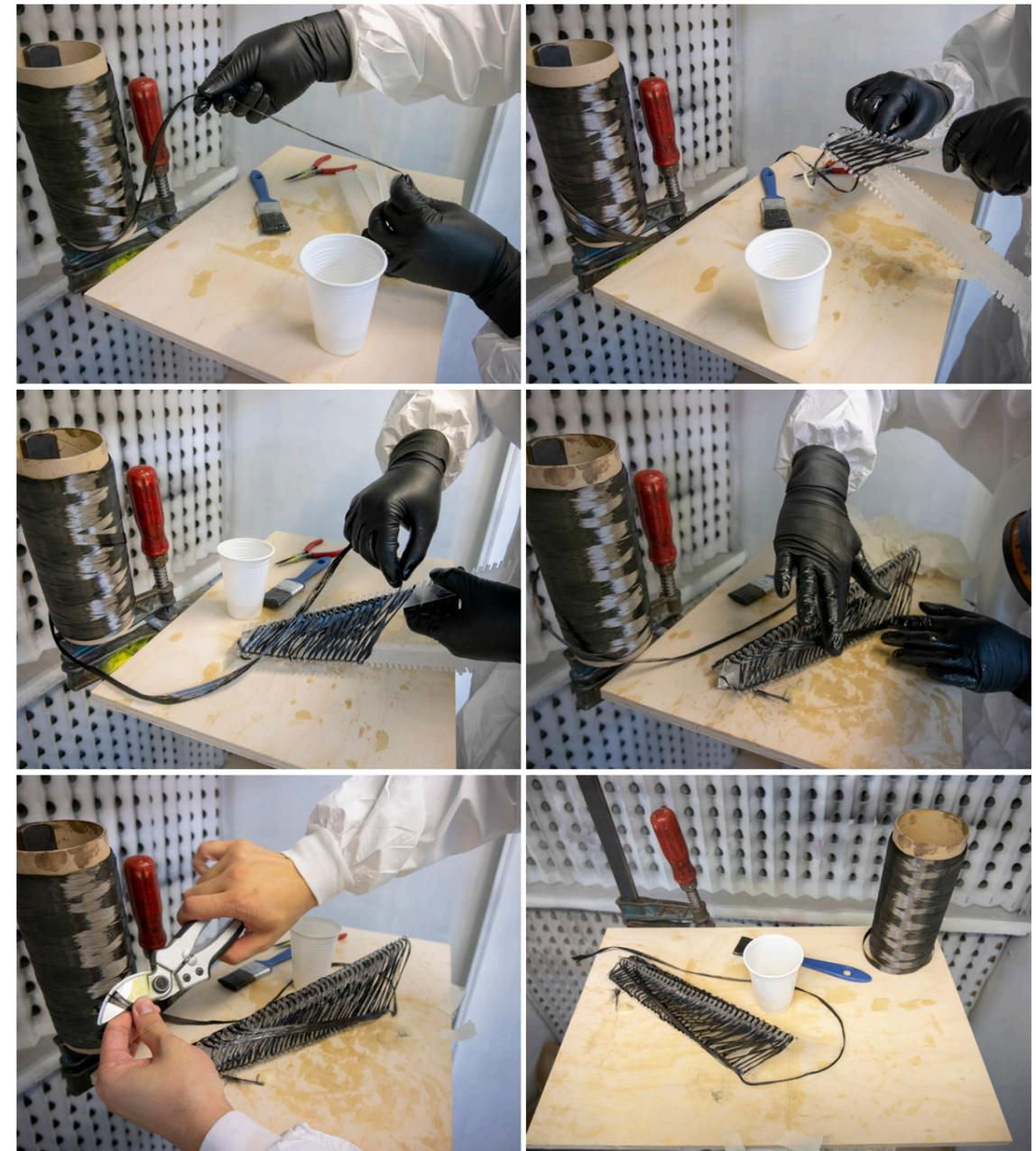
Figure 38. Experiment 5, Weaving process1-6. Author's own copyright.
