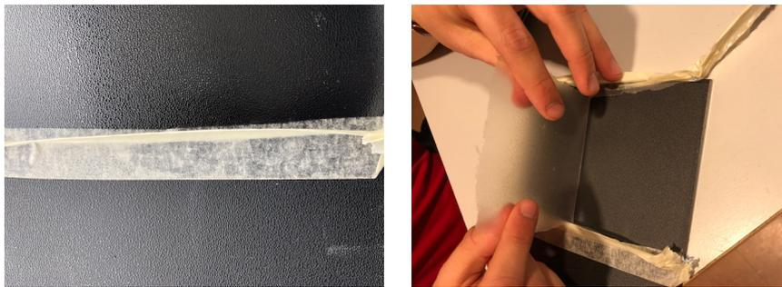
(a) *Paint applied to test plate 2 (above split line).* (b) *Paint in the process of removal from test plate.*
