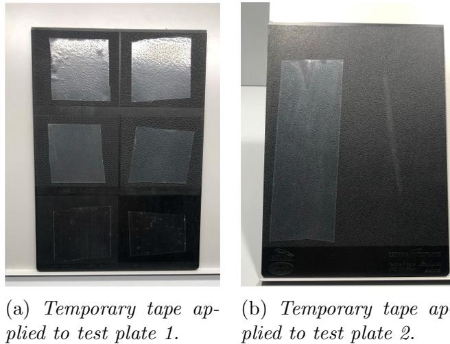
Figure 6.1: *Temporary tape applied to test plates in light D65. D65 light mimics daylight.*
