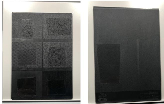
(a) *Scratch & resistant tape applied to test plate 1.* (b) *Scratch & wear resistant tape applied to test plate 3.*
