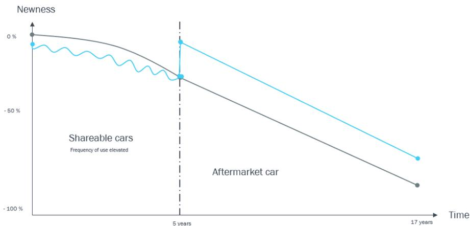
Figure 6.6: *Visualizing the decrease in newness of baseline lower cover (starting from 0%) and of lower cover with a protective layer (starting from -10%).*
