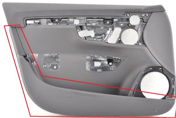
Figure 5.4: *The lower cover for Volvo S90. It is designed as a merged part with the panel carrier and the lower cover. (The red marked part is the lower cover). Copyright A2Mac1 [53].*
