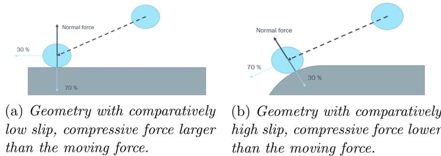
Figure 4.9: *Visualizing object hitting surface with associated force components.*
