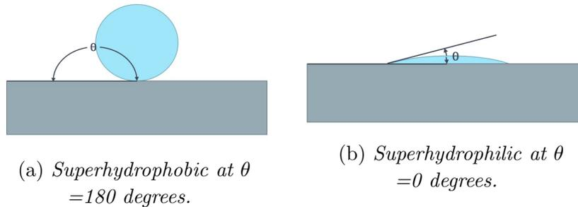
Figure 2.4: *Figure 2.4a and 2.4b illustrates a liquid drop in profile on a surface.*
