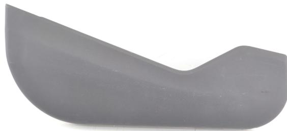
Figure 5.5: *The lower cover for the car model BMW X1. It is designed as one part (only the lower cover) which is mounted to the panel carrier in a later stage. Copyright A2Mac1 [53].*
