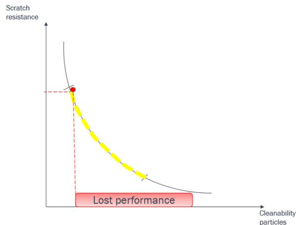
Figure 5.6: *Euler curve illustrating the trade off with scratch resistance texture and "cleanable" texture.*
