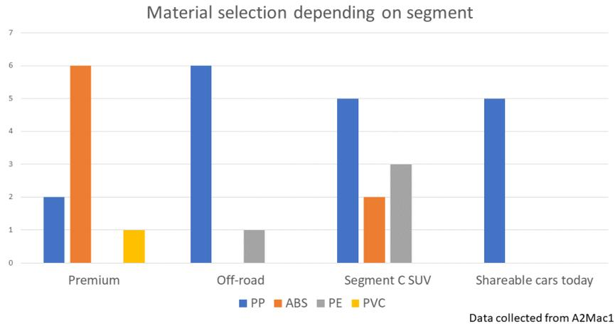
Figure 5.2: The figure illustrates a diagram which shows the material selection for the lower cover (of the door-panel) depending on different car segments [53].
