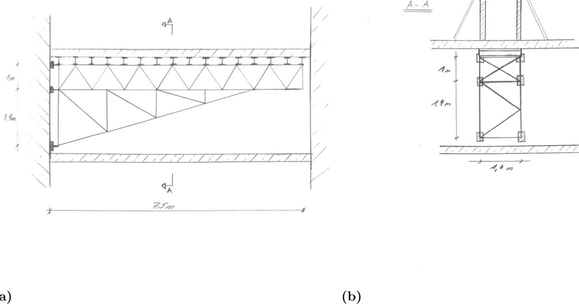
**Figure 6.4:** Conceptual sketches of the truss cantilever concept. To the left, the longitudinal section of the cantilever is shown. To the right, the section A-A can be seen.
