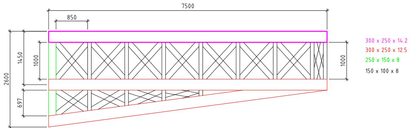
**Figure 6.6:** *Final truss dimensions.*
