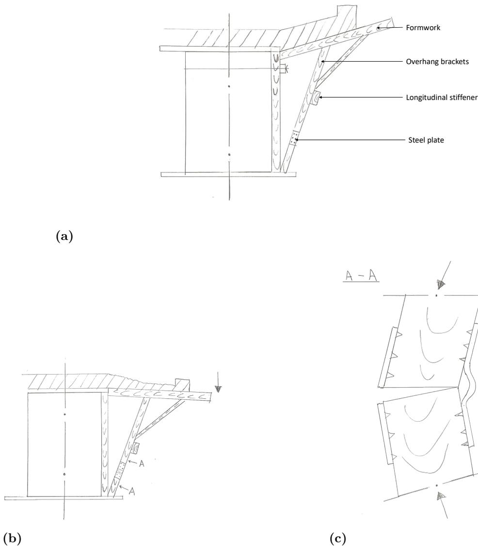
**Figure 4.1:** *The over hanging brackets seen in 4.1a were undersized in the longitudinal direction (into the picture). When loaded, see 4.1b, the circumstances lead to the buckling of the bracket and the nail plate, see 4.1c.*
