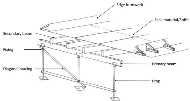
**Figure 2.1:** *Examples of different element types in a TWs design.*
