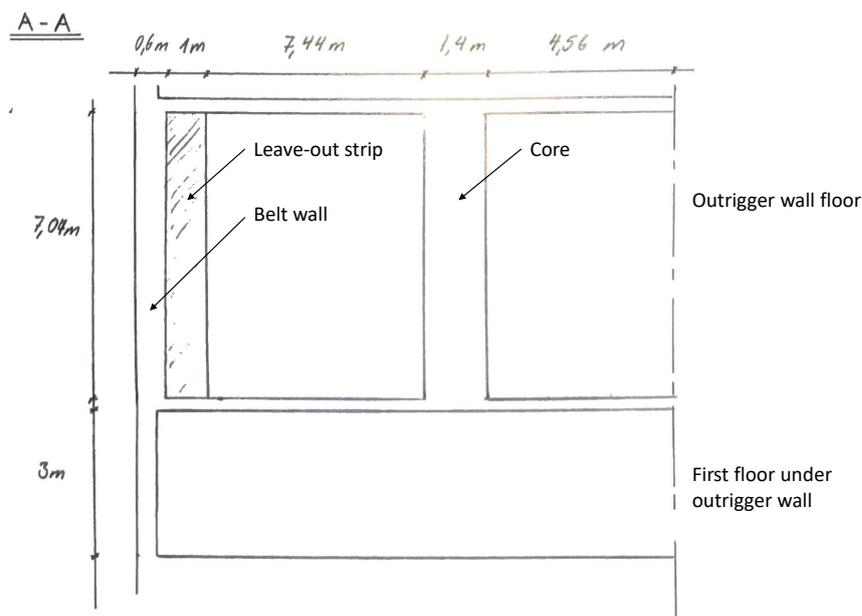
**Figure 6.3:** Simple sketch of the outrigger wall floor elevation.
