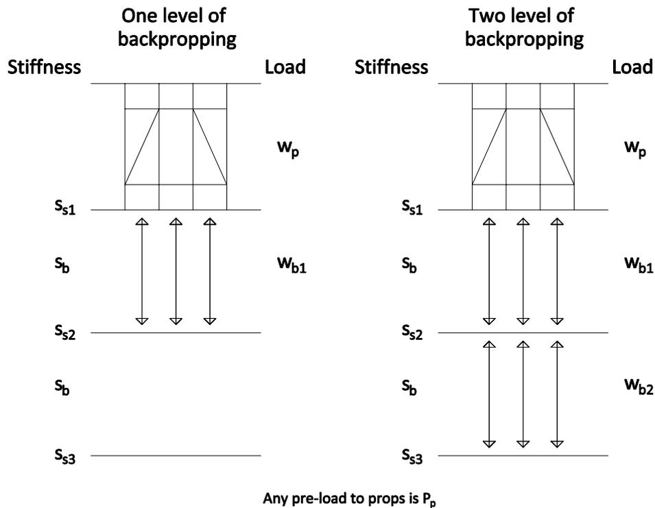
**Figure 2.5:** *How to backpropping in one and two levels, see Table 2.1 for load distribution.*
