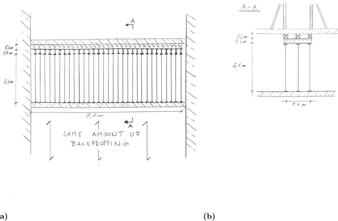
**Figure 6.5:** *Conceptual sketches of the propping concept. To the left, a section of the props together with the primary and secondary beam are illustrated. To the right, Section A-A can be seen with a row of props.*
