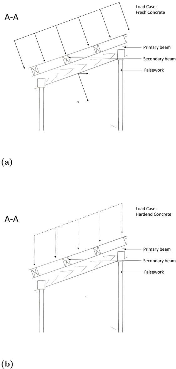
**Figure 4.3:** *On the left the behaviour off fresh concrete can be seen togheter with the resulting force components. On the right the behaviour of hardened concrete is shown.*
