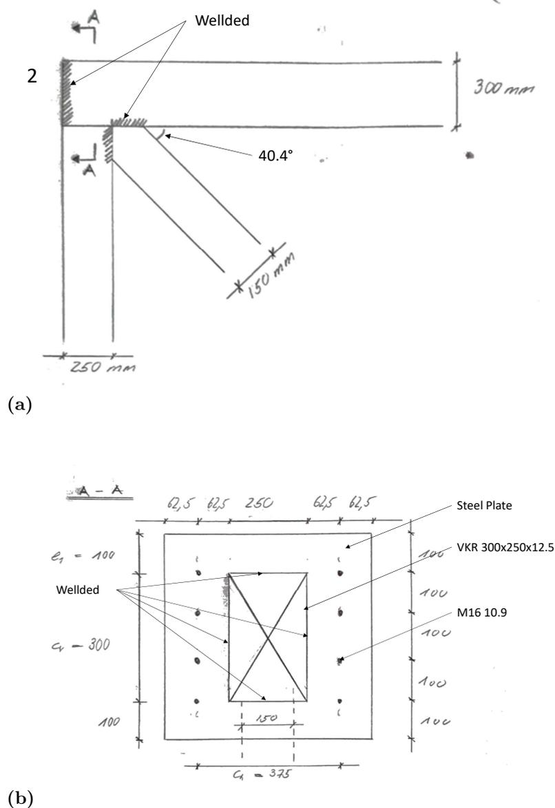
**Figure 6.8:** Dimensions and placements of the welds in node 2, see Figure 6.7.
