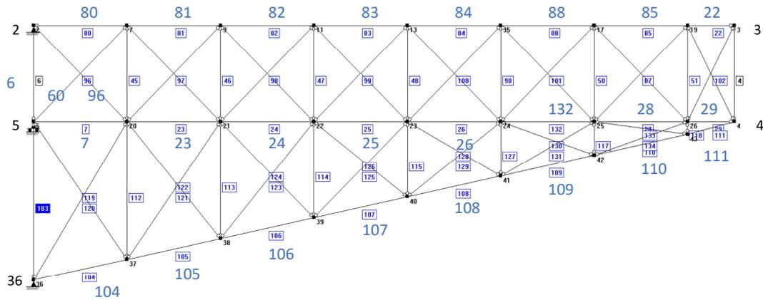
Figure 6.7: Modell of the truss (Appendix E).
