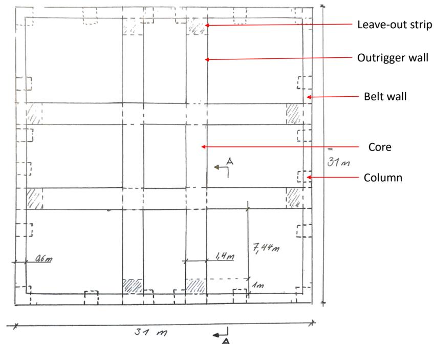
**Figure 6.2:** Sketch of the floor plan.
