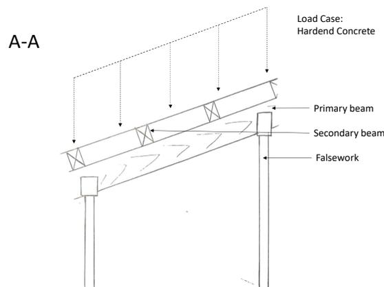
**Figure 4.4:** *Rods between the secondary beams could have helped prevent the accident (Personal communication, Mars 5, 2019).*
