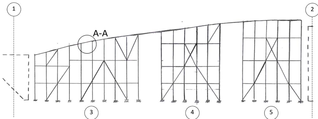
**Figure 4.2:** View of the two permanent supports (Number 1 and 2) and the three falsework sections (Number 3,4 and 5).
