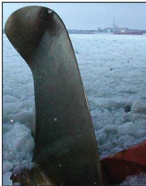
Figure 2.1: Bending of tip of open profile propeller due to ice-propeller interaction (Norhamo et al., 2009)
