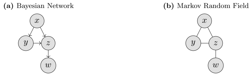
Figure 7.2: Shown in (a) is a Bayesian Network representing the probability distribution p(x,y,z,w) = p(x)p(y|x)p(z|x,y)p(w|z) . In (b) is a Markov random field representing the probability distribution p(x,y,z,w) = \frac{1}{Z}e^{-E_1(x,y,z)-E_2(z,w)} .
