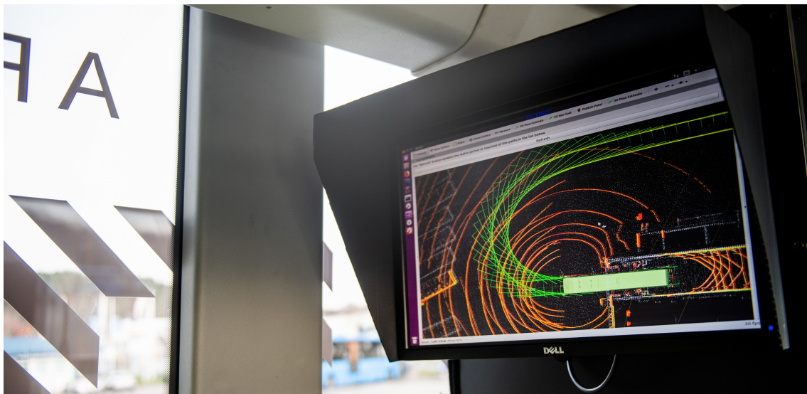
Figure 2.2: Example of what a LiDAR detects (Volvo Group, 2018)
