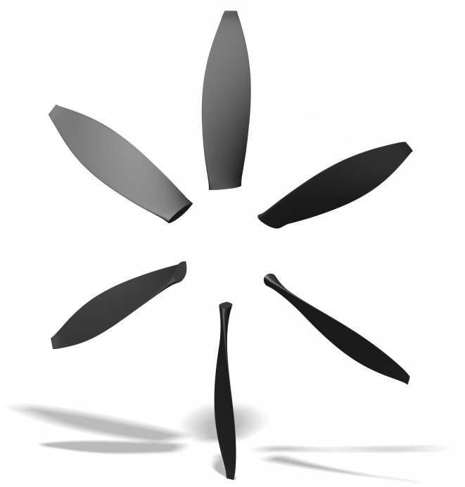
Figure 2.11: 3D model of baseline propeller created in CATIA V5.
