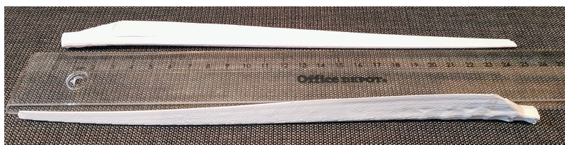
Figure 5.1: 3D-printed blade with a length of 25 cm.
