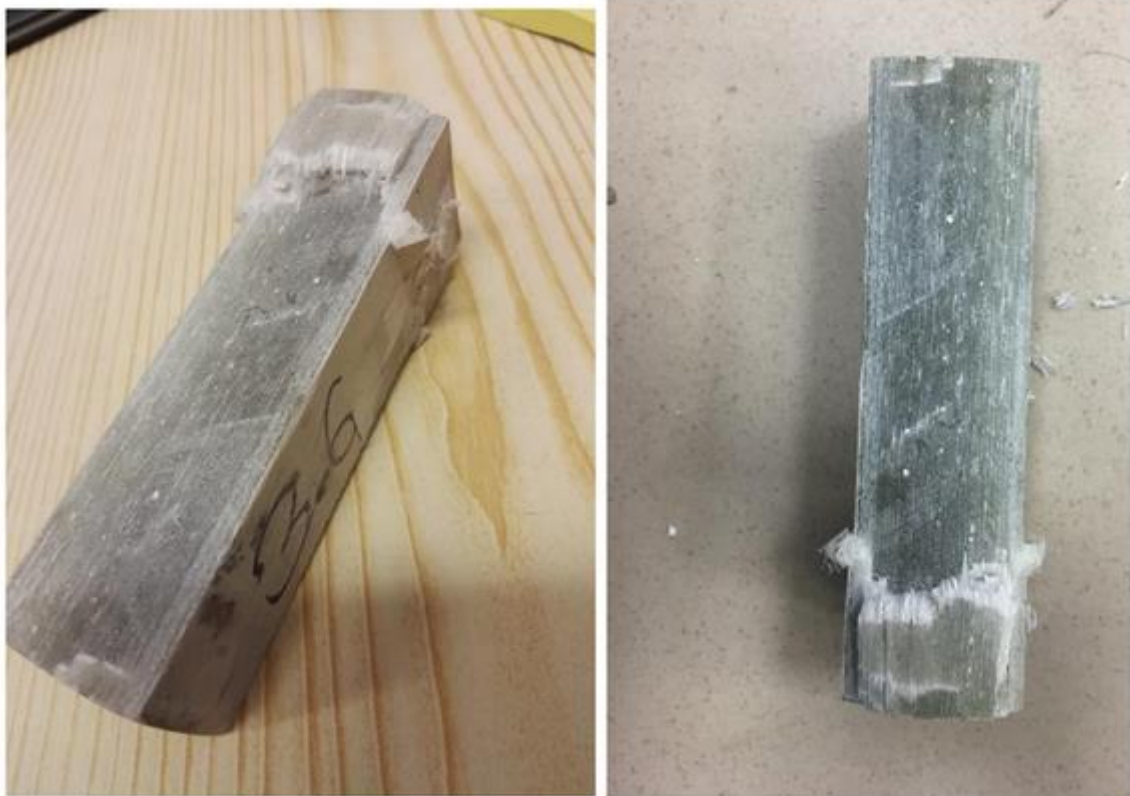
1.16. Form of destruction of sample 3.6 in the compression test
