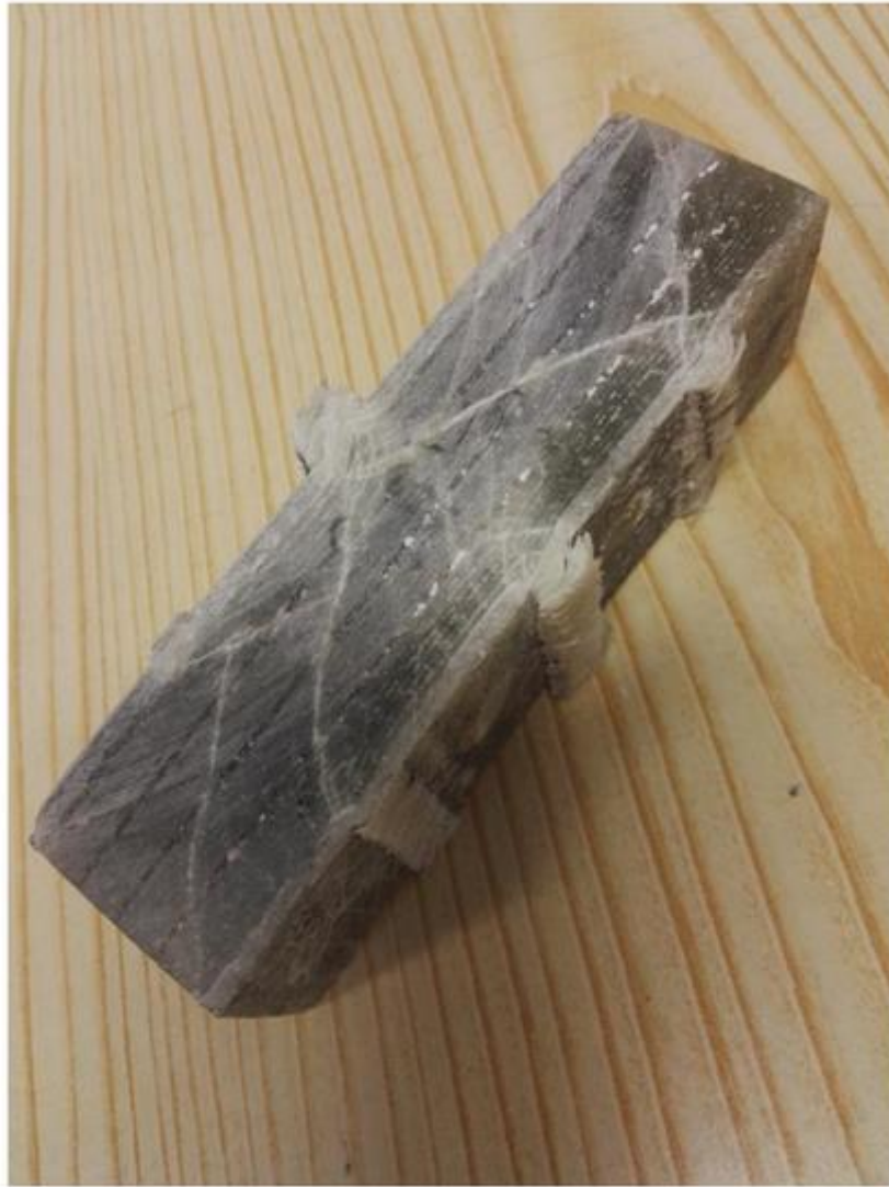
1.17. Form of destruction of sample 3.6 in the compression test
