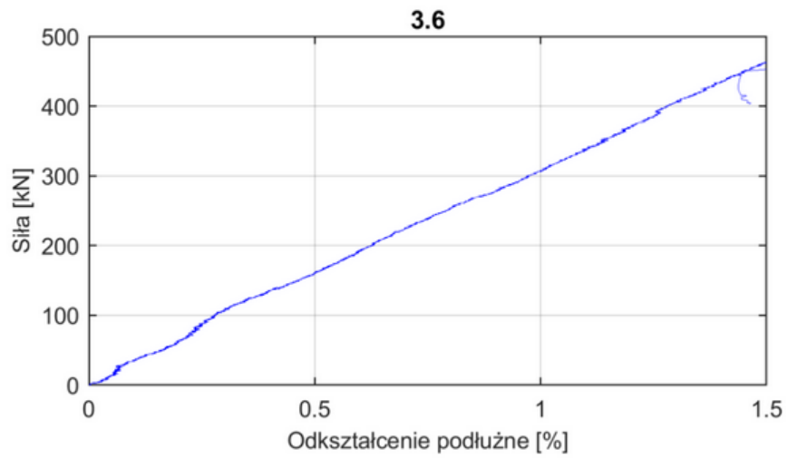
1.4. Load - longitudinal deformation for the sample 3.6
