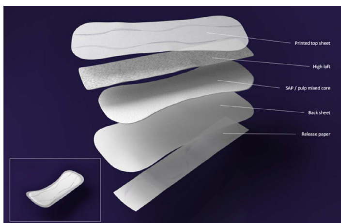
Figure 8. Layers of Tena Discreet Mini (Internally available information from Essity) Presented with permission.
