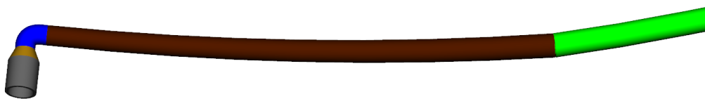
Figure 3.9: The end of the recirculation pipe that is fitted to the opening in the tank. The green part extends all the way up to the filler neck, as can be seen in figure 3.5.
