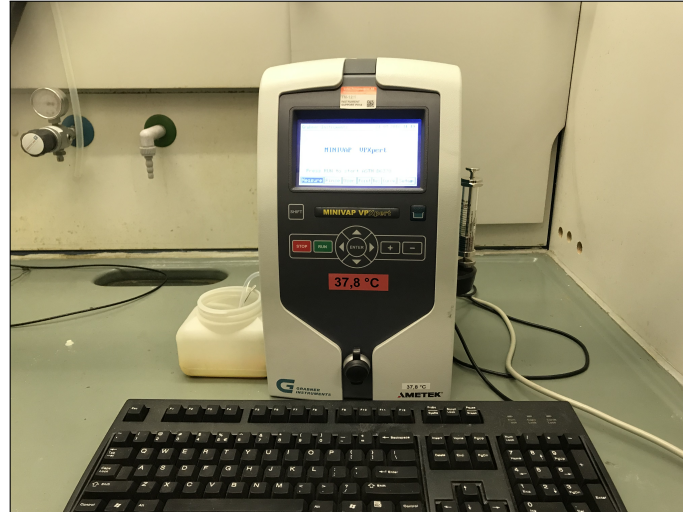
Figure 3.1: Machine used to measure the saturation pressure of the used fuel.
