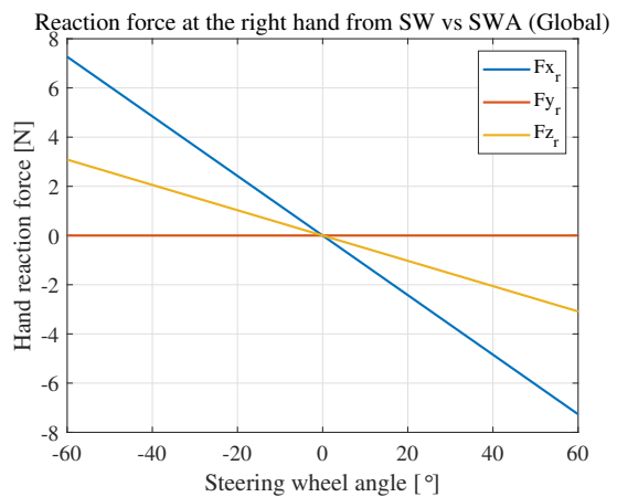
Figure A-4: Reaction force at the right hand over varying steering wheel angle
