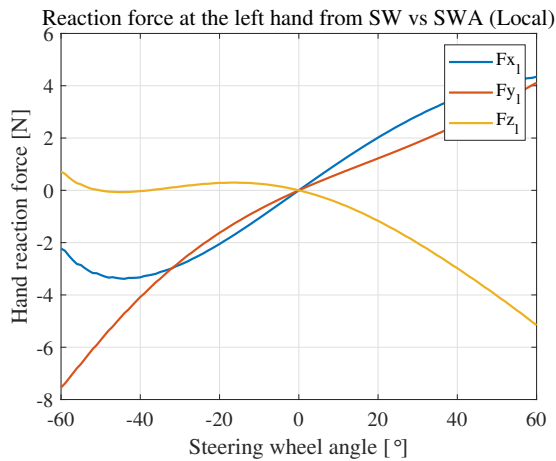
Figure A-5: Reaction force at the left hand expressed in local forearm frame
