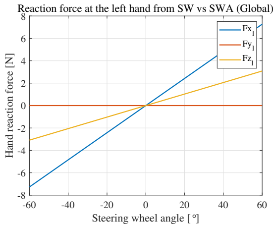
Figure A-3: Reaction force at the left hand over varying steering wheel angle
