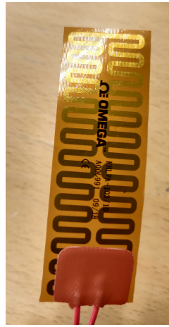
Figure 3.11: Kapton insulated flexible heater.
