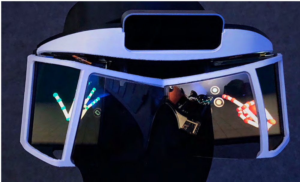
Figure 2.4: Helmet 3D printed that together with the Leap Motion Controller allows hand tracking. Image retrieved from the official website [3]
