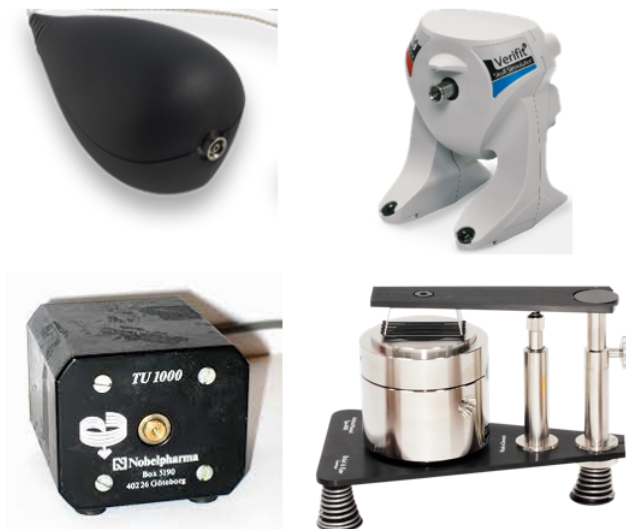
Figure 2.1: Examples of skull simulator and artificial mastoid. Skull Simulator SKS 10 by Interacoustics [16] (top left); Verifit Skull Simulator by Audioscan [17] (top right); Skull Simulator TU 1000 by B. Håkansson and P. Carlsson (1989) [18] (bottom left); Artificial Mastoid type 4930 by Bruel & Kjaer [19] (bottom right).
