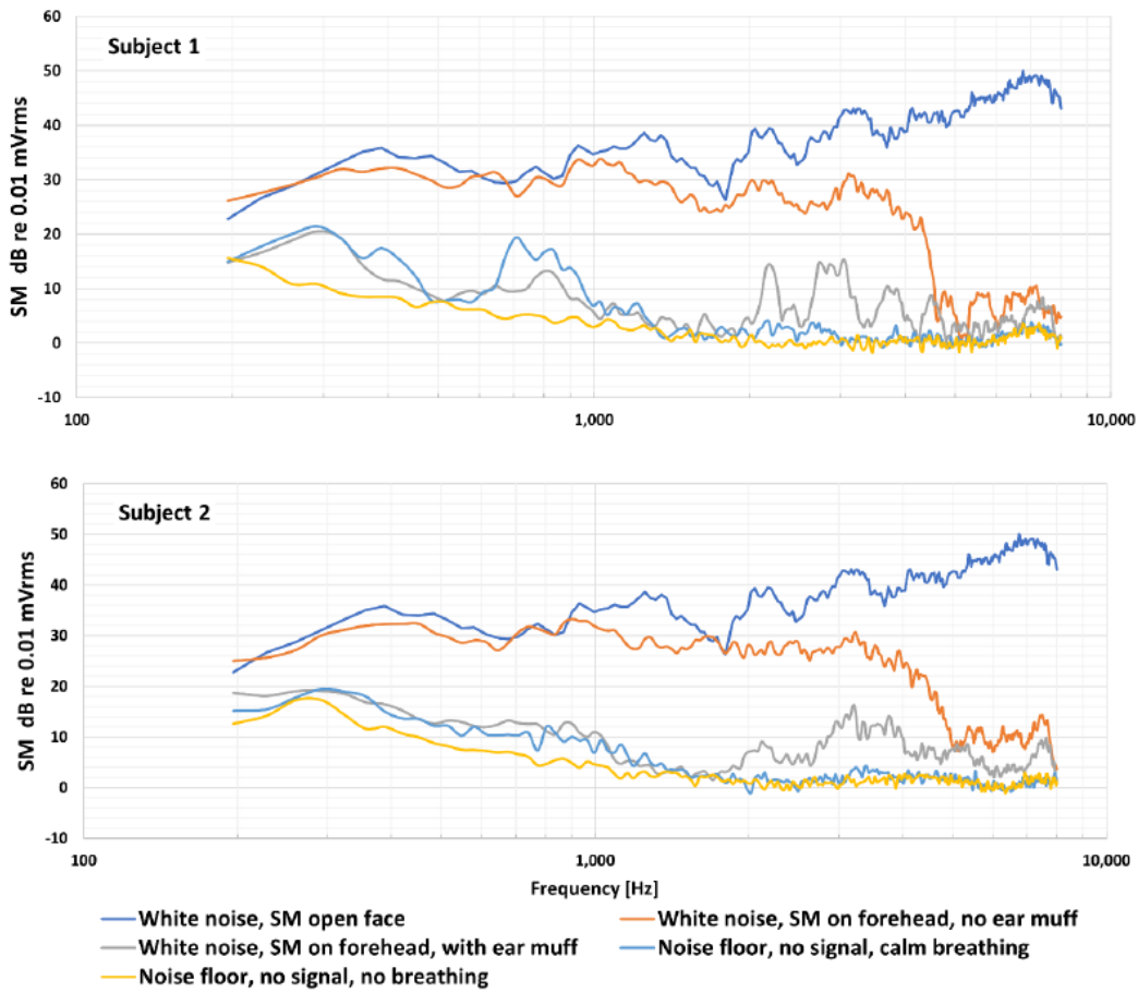
Figure 4.1: Skin microphone electrical output to input white noise in dB relative to 0.01 mV_{rms} on Subject 1 and 2.
