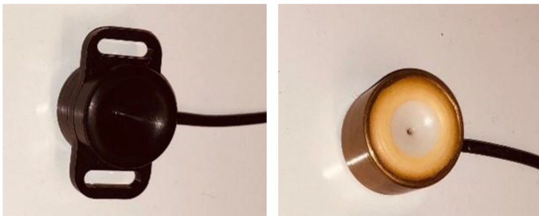
Figure 3.2: Skin microphone according to Hodgetts et al. 2018 [29] (left); Previous skin microphone with brass housing (right) according to Hodgetts and Scott (personal communication).
