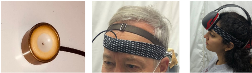
Figure 3.6: Skin microphone open faced (left); mounted on the forehead with soft band (middle); mounted on the forehead and with additional shielding by an earmuff (right).
