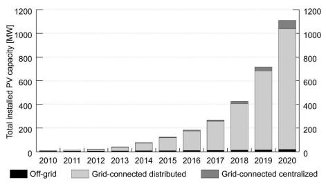
Figure 8 . Total installed PV capacity in Sweden (Lindahl et al., 2022)
