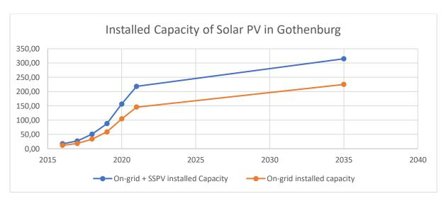
Figure 4 First Scenario Installed Solar PV capacity in Gothenburg (MW)
