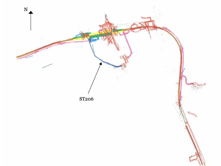
Figure 5.4: Map showing the service tunnel ST206 at the Korsvägen part of the West link, where some shotcrete arches have been constructed (Bergman & Andersson, 2019).
