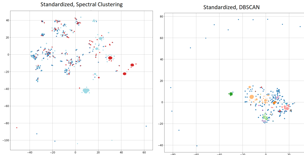
Figure 4.9: Two examples of bad clusterings due to clustering algorithm. The left image using Spectral clustering have entangled the clusters. The right image using DBSCAN have a bit too many data points clustered as noise. The noise class is colored with blue.
