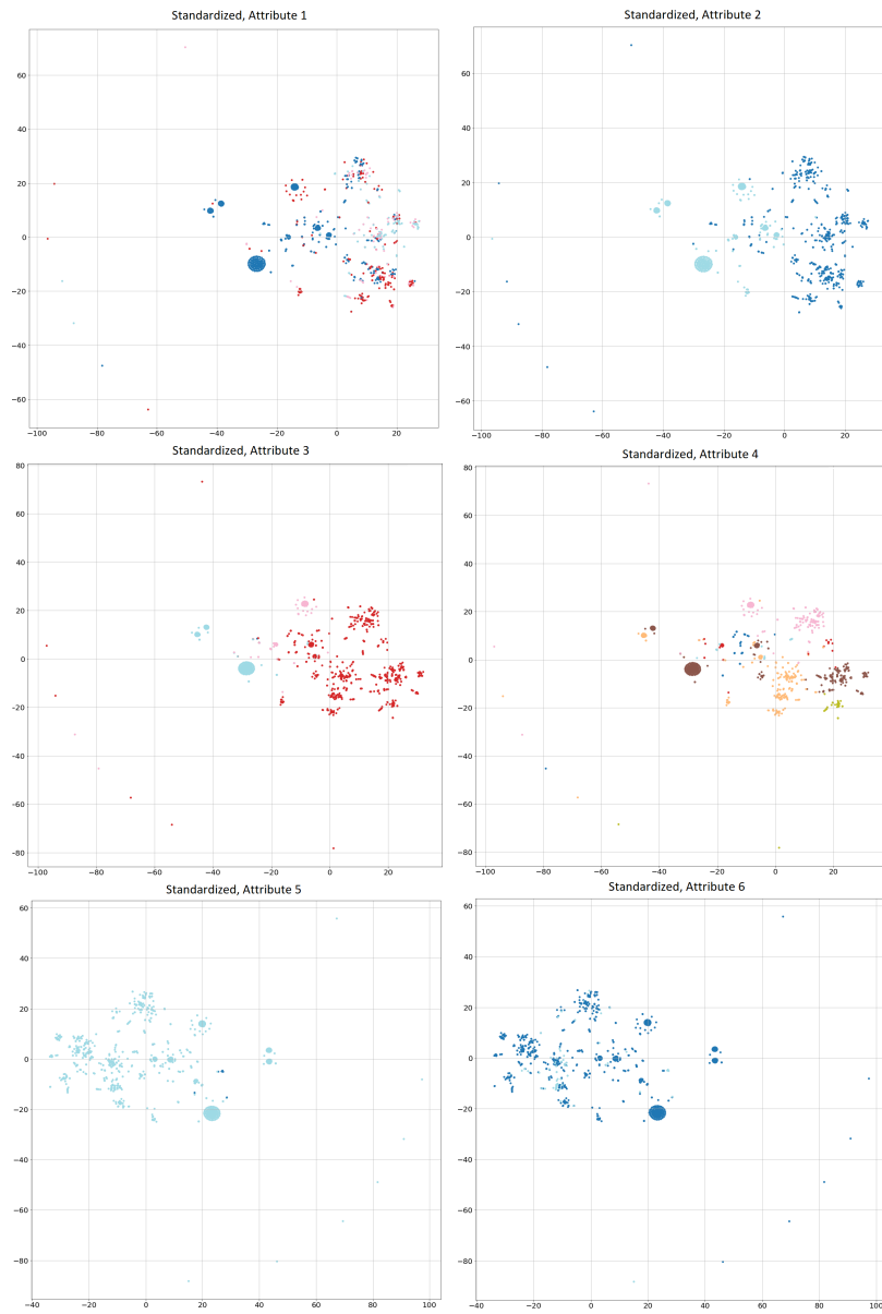
Figure 4.4: t-SNE mapping of standardized feature vectors coloured by selected attributes 1 to 6, counting left to right, top to bottom. The colouring of the t-SNE mappings shows quite clear patterns for attributes 1 to 4, 5 is debatable whether it is a good cluster or not and attribute 6 display no obvious pattern. For full scale mappings, see Appendix A.
