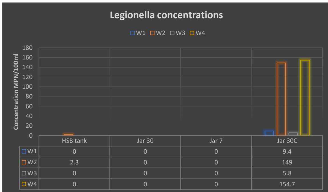
Figure 22. Graphs showing L. Pneumophila concentrations in HSB tank, Jar 30, Jar 7, Jar 30C over four weeks.
