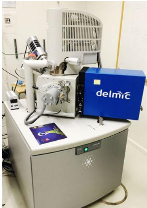
Figure 21 showing Quanta 200 ESEM used for imaging biofilms on the coupons.
