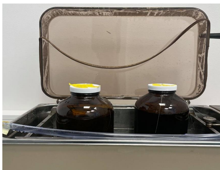
Figure 16 showing the Jar 30 and Jar 30C placed in water bath at 30 °C.
