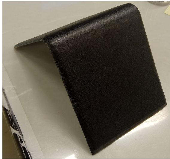
Figure 3.5: Manufactured L-shaped composite, [0]_{16} using titanium tool.
